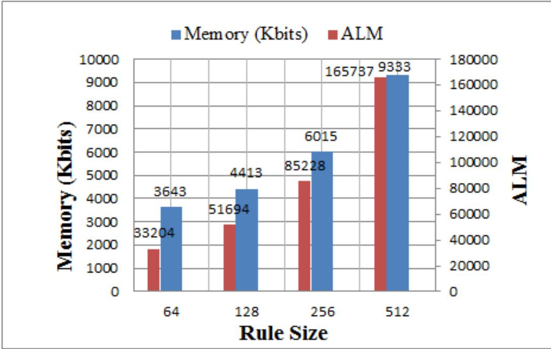
Figure 5.15: Logic gate and memory bit scalability with increasing rule size
