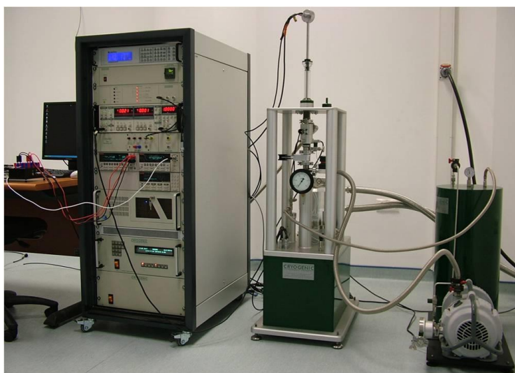
Figure 3.3 Vibrating sample magnetometer (VSM) in Central Laboratory, METU-Ankara, TURKEY (Cryogenic Limited PPMS).
