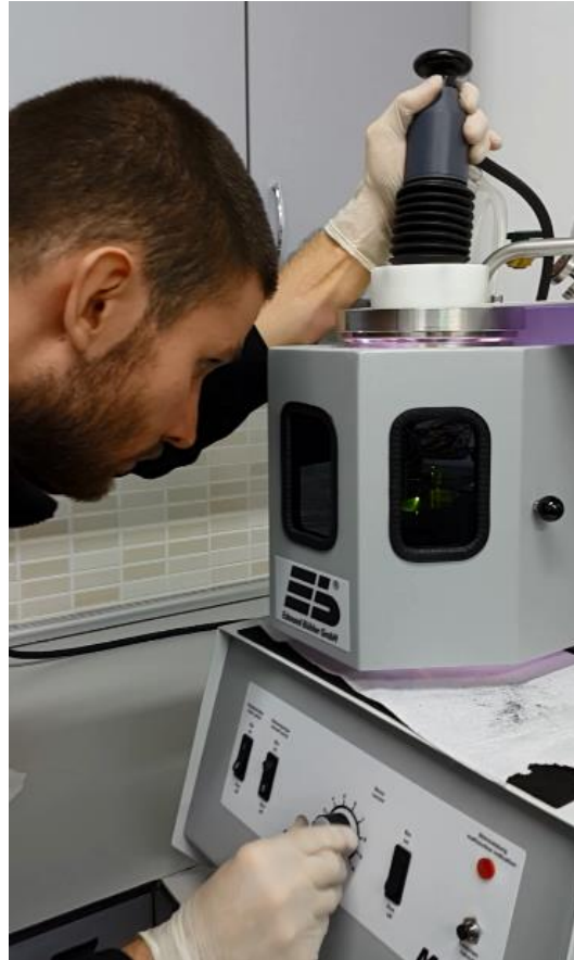
Figure 3.1 A capture of alloy production in an arc melting furnace.
