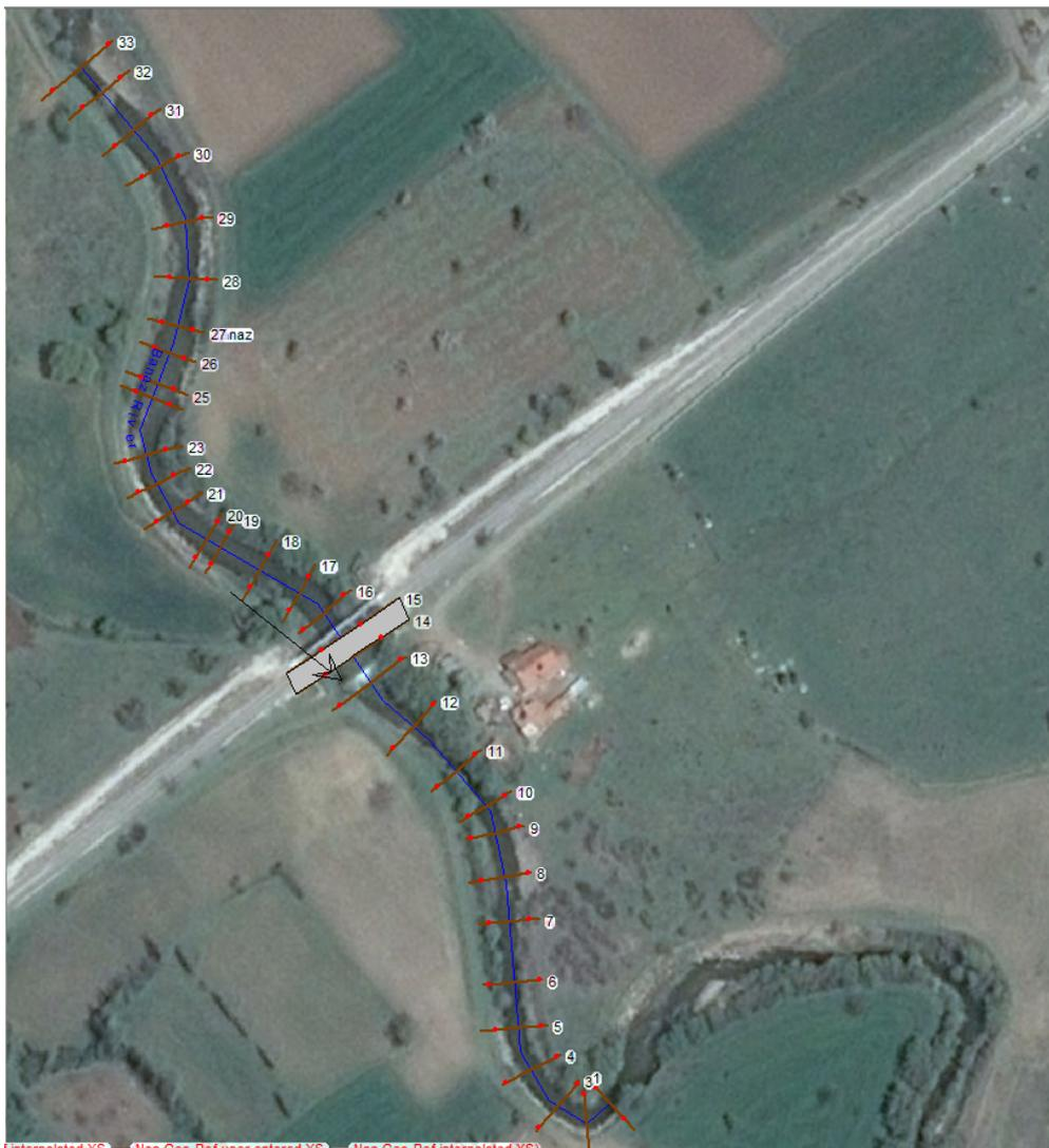
Figure 3.5. HEC-RAS view of river geometry and cross-sections
