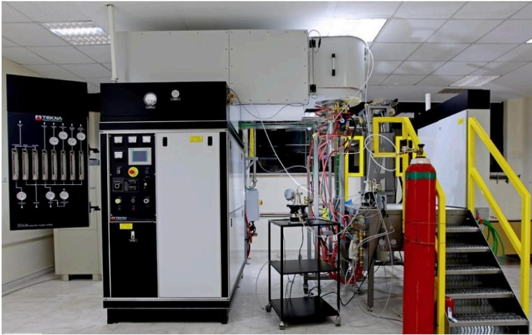
**Figure A.1:** Photograph of induction plasma system
