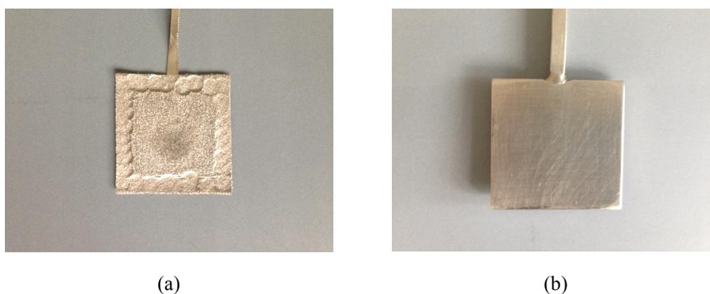
**Figure 3.10:** Photographs of (a) negative electrode prepared with paste and foam and (b) corresponding counter electrode for electrochemical measurements.
