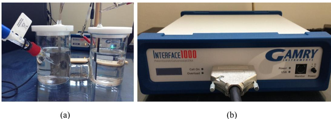
**Figure 3.11:** Photographs of (a) the electrochemical charge-discharge measurement setup for electrode prepared by paste and foam and (b) Gamry Interface 1000 potentiostat/galvanostat/ZRA.
