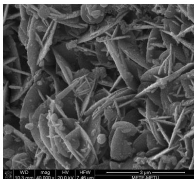
**Figure 4.12:** SEM image of the surface of AB<sub>2</sub> powder subjected to hot KOH treatment for 100 minutes.
