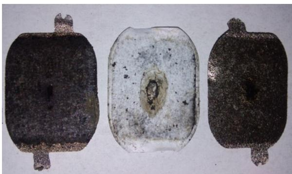
**Figure 2.13:** The negative electrode, separator and the positive electrode of the battery
