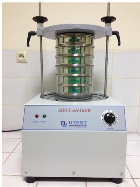
**Figure 3.2:** The sieve shaker with the sieves
