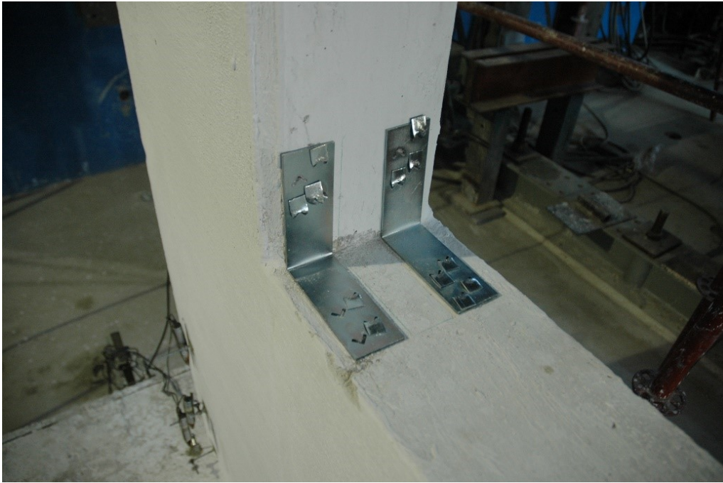
Figure 2.16: Steel angle brackets used at the lower corners of window opening
