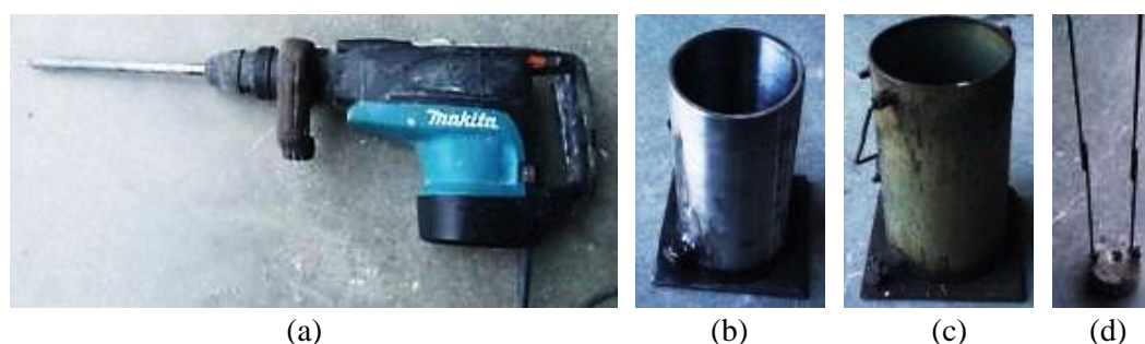
Figure 3.6. Apparatus Used in RCC Placement : (a) Pneumatic Hand Compactor; (b) 100x200mm Cylindrical Mold; (c) 100x200mm Cylindrical Mold and (d) Steel Apparatus for Uniform Compaction
