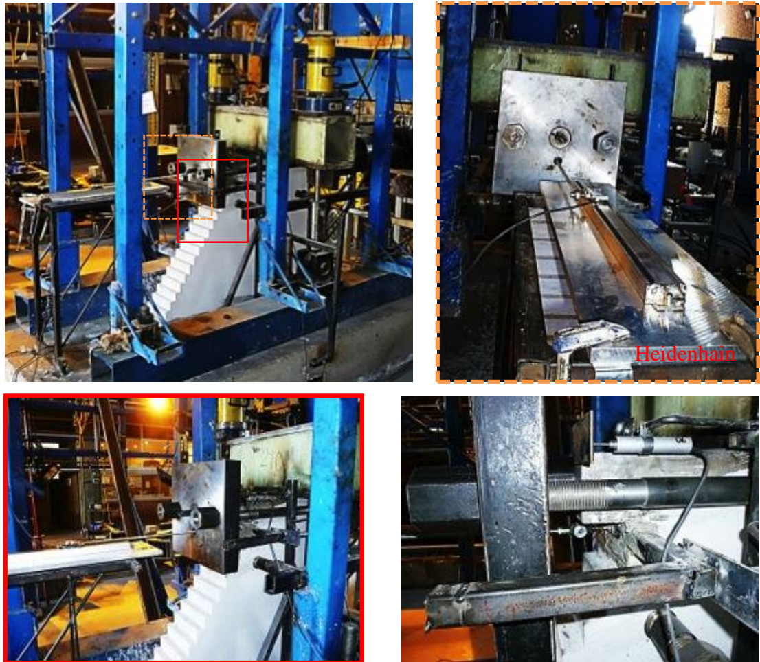
Figure 4.17. Test Setup and LVDT's for Tip Displacement Recording in Specimen 3
