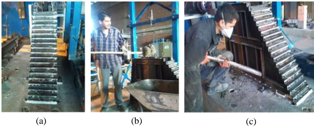
Figure 4.18. Preparation of Specimen : (a) Formwork, (b) Concrete Placement and (c) Vibration for Concrete Settling
