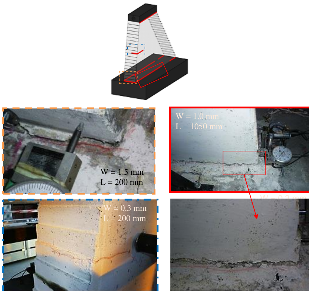
Figure 5.14. Cracks Formed during Pushover Experiment for Specimen 1
