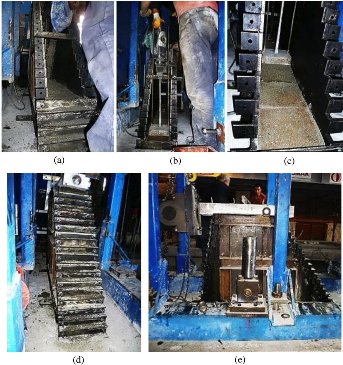
Figure 4.23. Preparation of Specimen : (a) Placement of Concrete, (b) Compaction, (c) Compacted Concrete Layer, (d)-(e)
