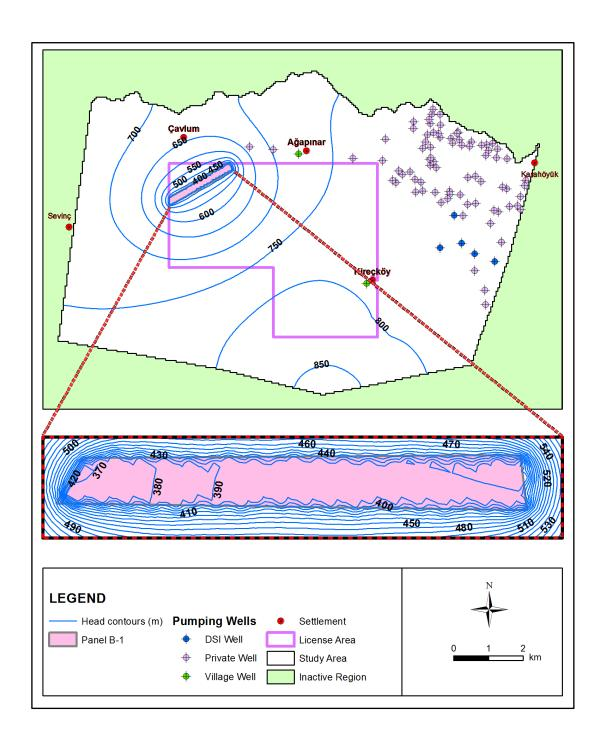
Figure 6.5. Head contours after dewatering simulations at panel B-1
