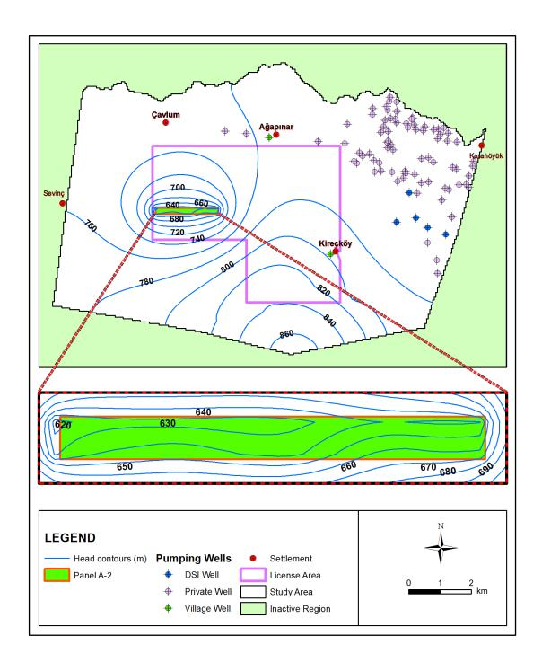
Figure 6.4. Head contours after dewatering simulations at panel A-2
