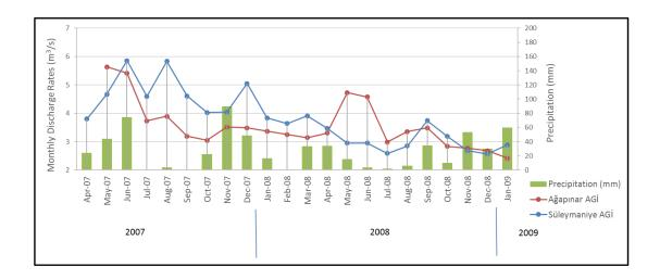
Figure 3.2. Monthly discharge rates at Ağapınar and Süleymaniye gauging stations between 2007-2009 (DSI, 2010)
