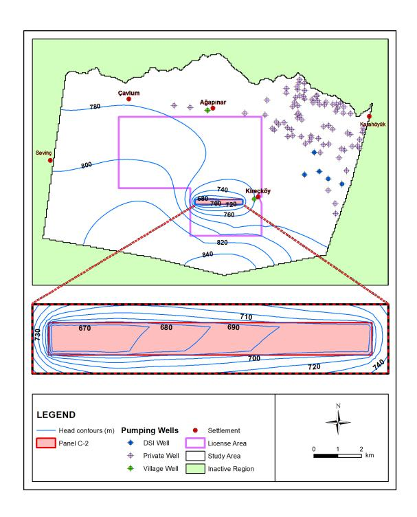
Figure 6.8. Head contours after dewatering simulations at panel C-2
