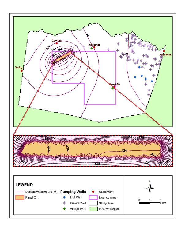
Figure 6.9. Drawdown contours after dewatering simulations at panel C-1
