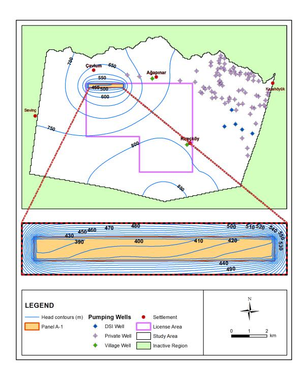
Figure 6.3. Head contours after dewatering simulations at panel A-1
