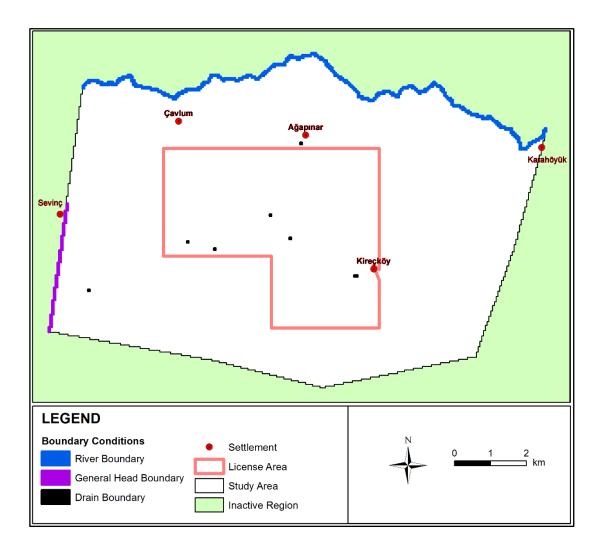
Figure 4.4. Boundary conditions of the model domain
