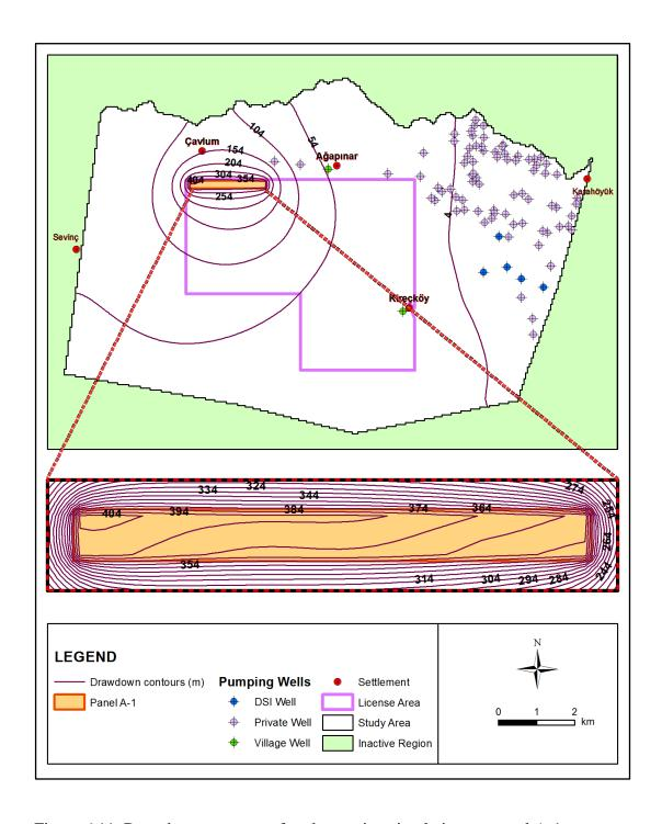
Figure 6.11. Drawdown contours after dewatering simulations at panel A-1
