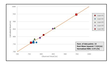
Figure 5.6. Calculated versus observed head values and calibration results of the model
