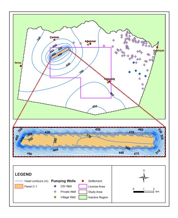
Figure 6.7. Head contours after dewatering simulations at panel C-1
