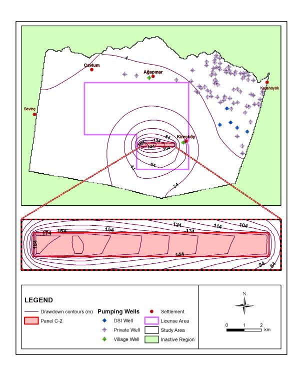
Figure 6.14. Drawdown contours after dewatering simulations at panel C-2
