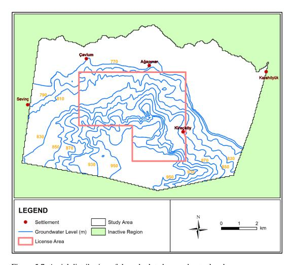
Figure 5.7. Aerial distribution of the calculated groundwater levels
