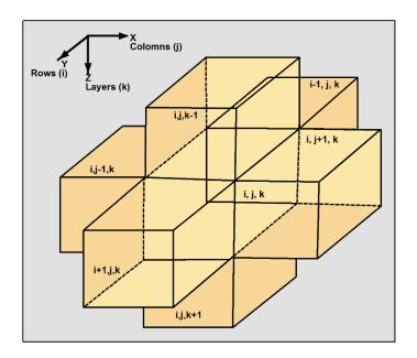
Figure 4.2. Cell i, j, k and indices for the six adjacent cells (Modified from McDonald and Harbaugh, 1988).
