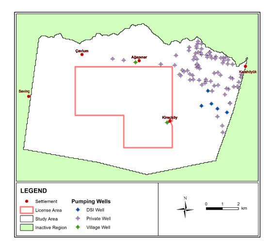
Figure 5.4. Pumping wells within the model domain
