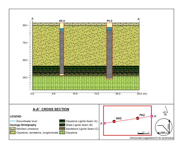
Figure 3.7. Cross section of the first nested wells group
