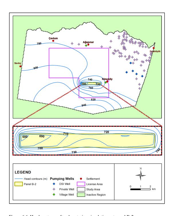
Figure 6.6. Head contours after dewatering simulations at panel B-2
