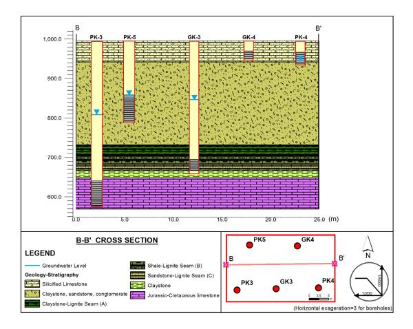
Figure 3.8. Cross section of the second nested wells group
