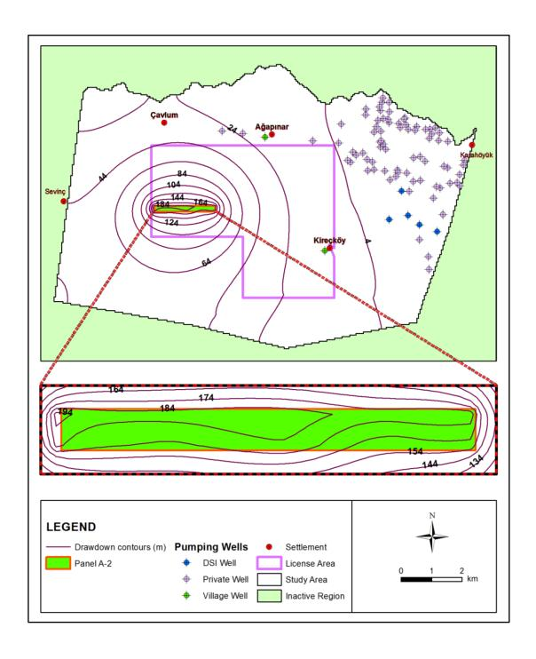
Figure 6.12. Drawdown contours after dewatering simulations at panel A-2
