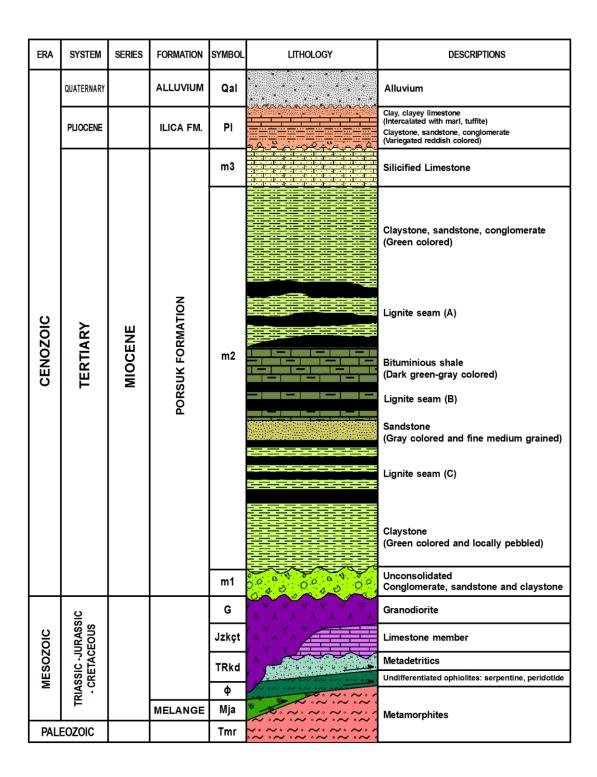
Figure 2.13. Generalized columnar section of the study area and its surroundings (Modified from Gözler et al., 1997, Siyako et al., 1991 and Senguler, 2013)
