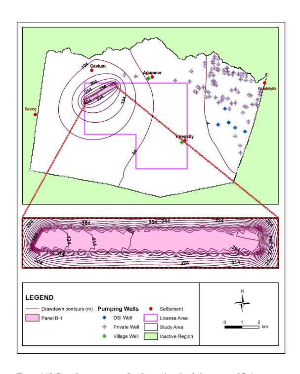
Figure 6.13. Drawdown contours after dewatering simulations at panel B-1
