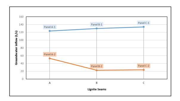
Figure 6.2. Groundwater inflow amounts for the A, B, C lignite seams dewatering simulations
