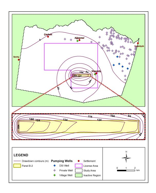
Figure 6.10. Drawdown contours after dewatering simulations at panel B-2
