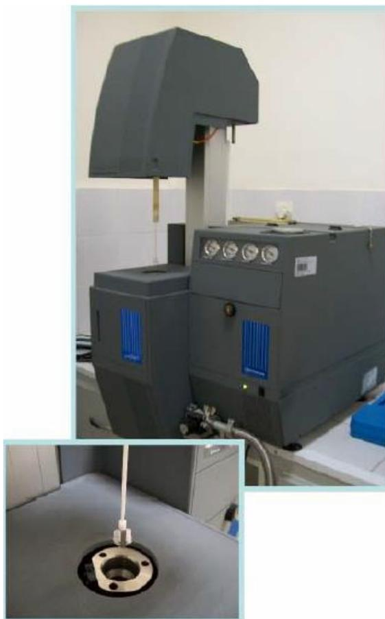
**Figure 3.3** DSC used in isochronal thermal analysis.
