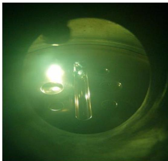
**Figure 3.1** Copper heart and arc melting.
