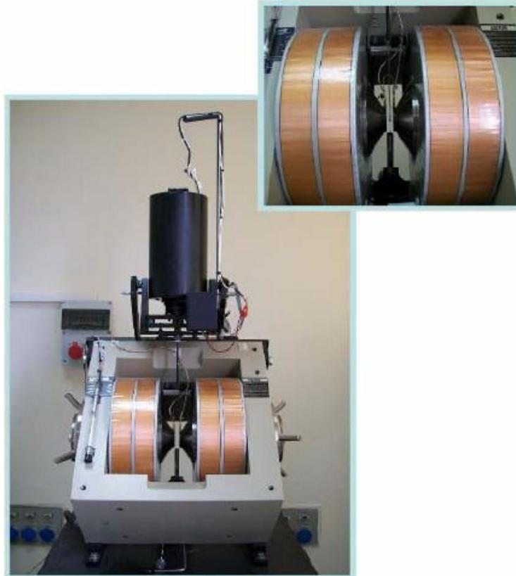
**Figure 3.4** VSM used for magnetic measurements.
