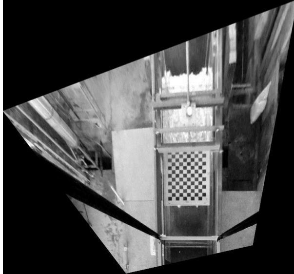
Figure 2-30 : The image after geometrical correction is applied
