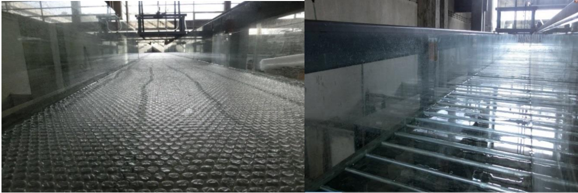
Figure 2-7 : Two different roughness types seen on the channel bed
