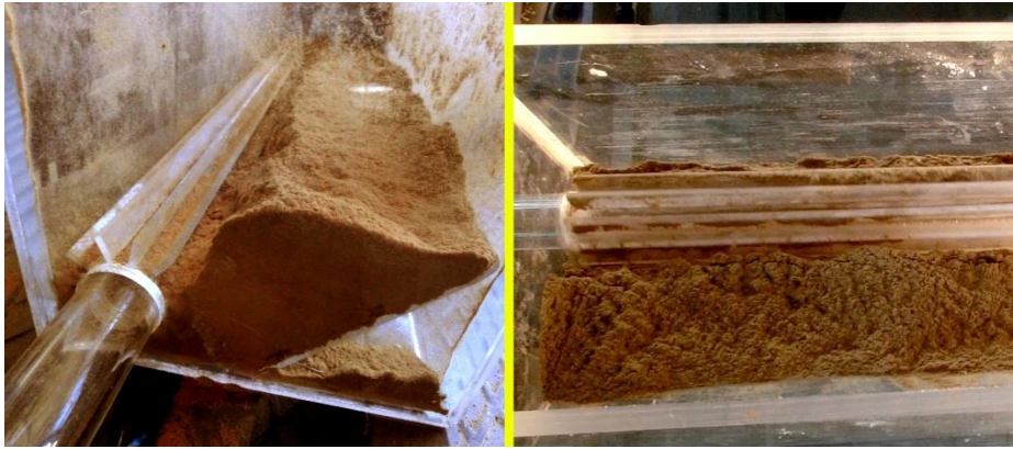
Figure 2-23 : Particle dispenser used to seed the flow with sawdust in PIV experiments viewed from two different angles
