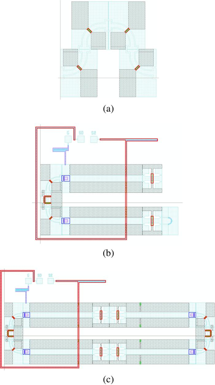
Figure 2.18: Layouts of (a) CWP bend test structure, (b) one port terminated with match load SPDT switch and (c) two SPDT switches cascaded back-to-back.
