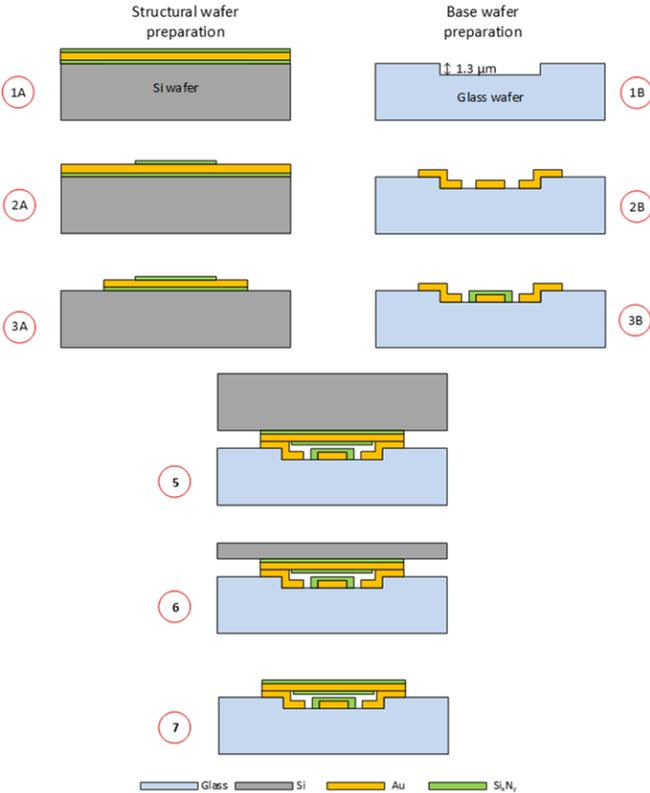
Figure 2.16: Schematic description of the fabrication process.
