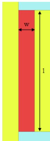
Figure A.2: Dimensions of a lumped port.
