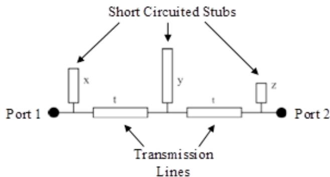
Figure 4.1: Schematic of the triple stub topology where  $x$ ,  $y$ ,  $z$  and  $t$  are the corresponding lengths.
