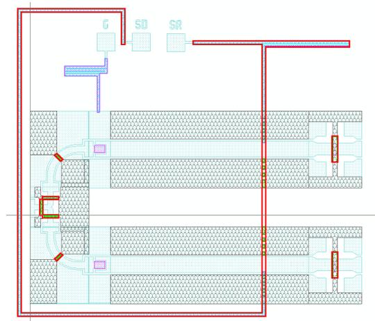
Figure 2.12: Layout of the designed SPDT switch from the wafer.
