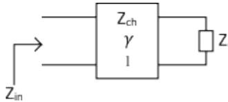
Figure 4.3: Schematic an unknown load with impedance  $Z_L$  is connected to one of the ports a transmission line.
