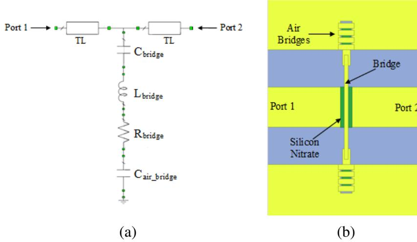
Figure 3.2: (a) Circuit model and (b) top view of the fixed-fixed beam.
