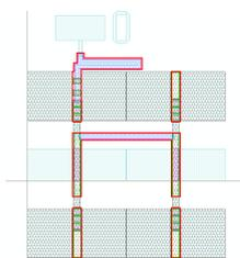
Figure 3.6: Layout of the first bit of the DMTL phase shifter.
