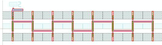
Figure 3.8: Layout of the third bit of the DMTL phase shifter.
