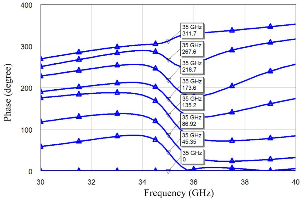
Figure 4.6: Expected phase characteristic of the designed 3-bit triple stub phase shifter.
