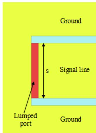
Figure A.1: Schematic of a lumped port excitation.
