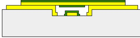
Figure 2.10: Section of a fixed-fixed beam.
