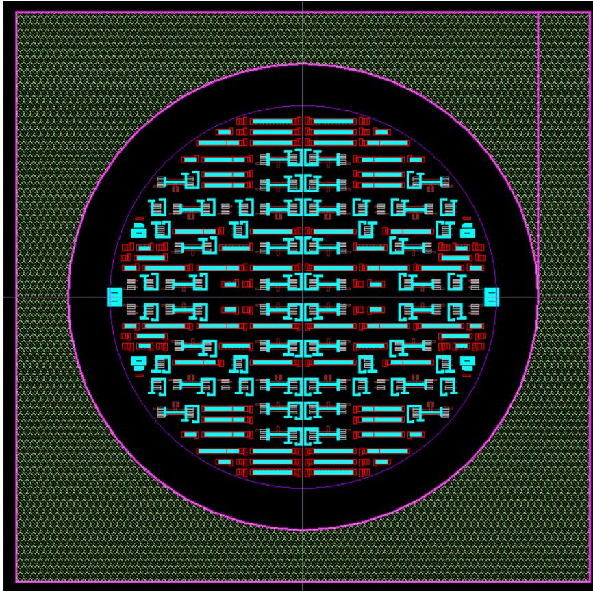
Figure 5.1: Layout of the full 4 inch wafer.
