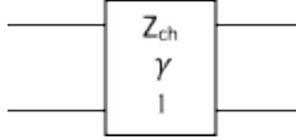
Figure 4.2: Schematic a two port transmission line with characteristic impedance  $Z_{ch}$ , propagation constant  $\gamma$  and length  $l$ .
