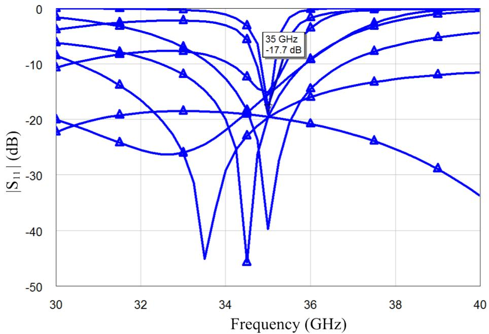
Figure 4.7: Expected return loss characteristic of the designed 3-bit triple stub phase shifter.
