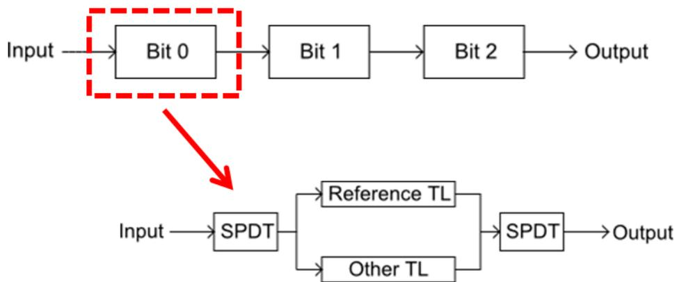
Figure 2.1: Layout of a 3-bit switch-line phase shifter.
