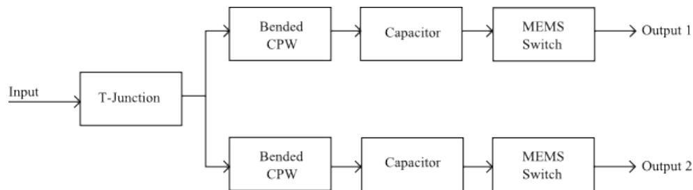
Figure 2.2: Illustration of the SPDT switch and its components.
