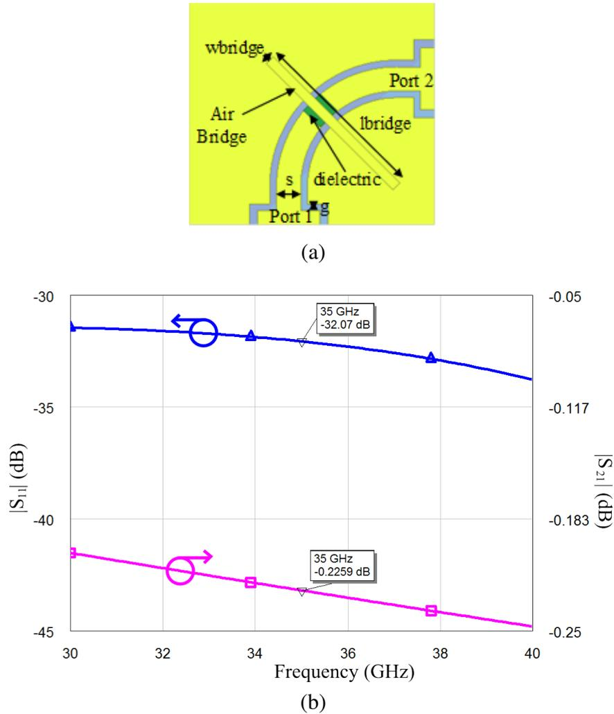
Figure 2.6: (a) Top view and (b) simulated  $|S_{i1}|$  of the designed CPW bend.
