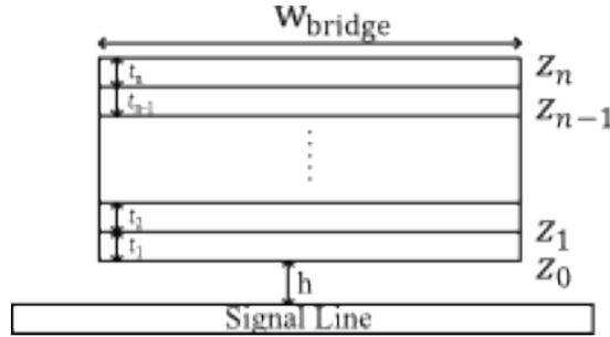
Figure 2.11: Section of an n-layer fixed-fixed beam with different widths of layers.
