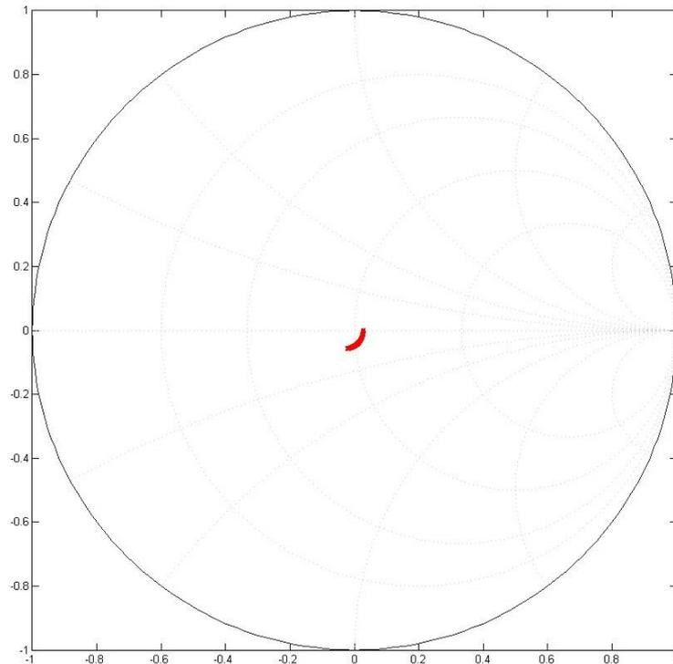
Figure A.3:  $S_{11}$  of a CPW simulated with lumped port.
