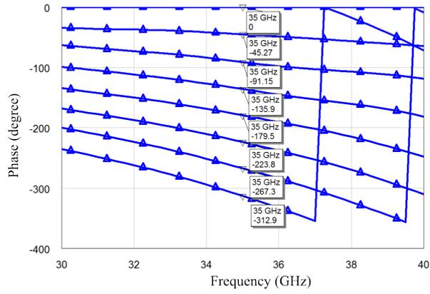
Figure 3.10: Expected phase characteristic of the designed 3-bit DMTL phase shifter.
