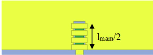
Figure 3.3: Top view of a MAM capacitor in one of the unit cells.
