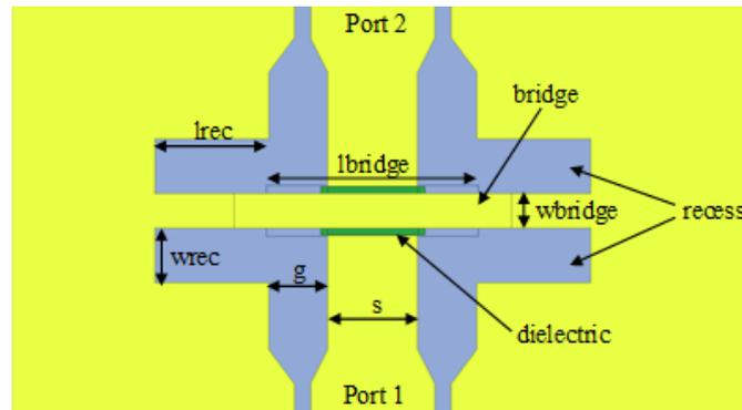
Figure 2.8: Layout of the designed capacitive-contact RF-MEMS switch.
