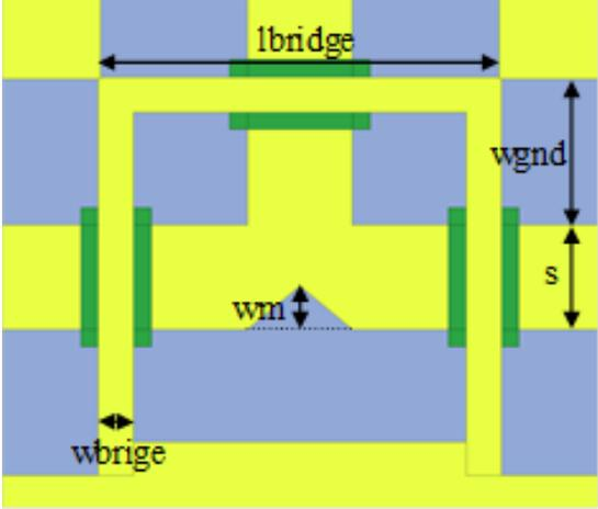
Figure 2.5: Notations used for the dimensions of the designed T-junction with 3 air-bridges.
