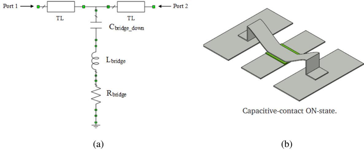
Figure 1.2: (a) Circuit model and (b) schematic projection of a switch in down position [9].
