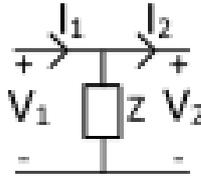
Figure 4.4: Schematic of a load with impedance  $Z$  parallel connected to a transmission line.
