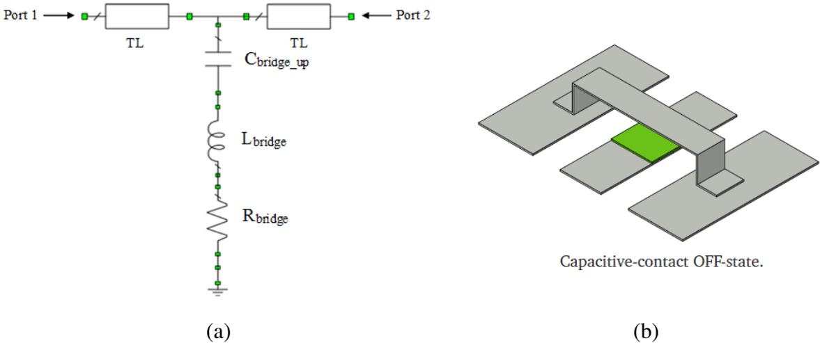
Figure 1.1: (a) Circuit model and (b) schematic projection of a switch in up position [9].
