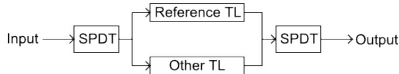
Figure 2.14: Illustration of one of the bits of the switch-line phase shifter.
