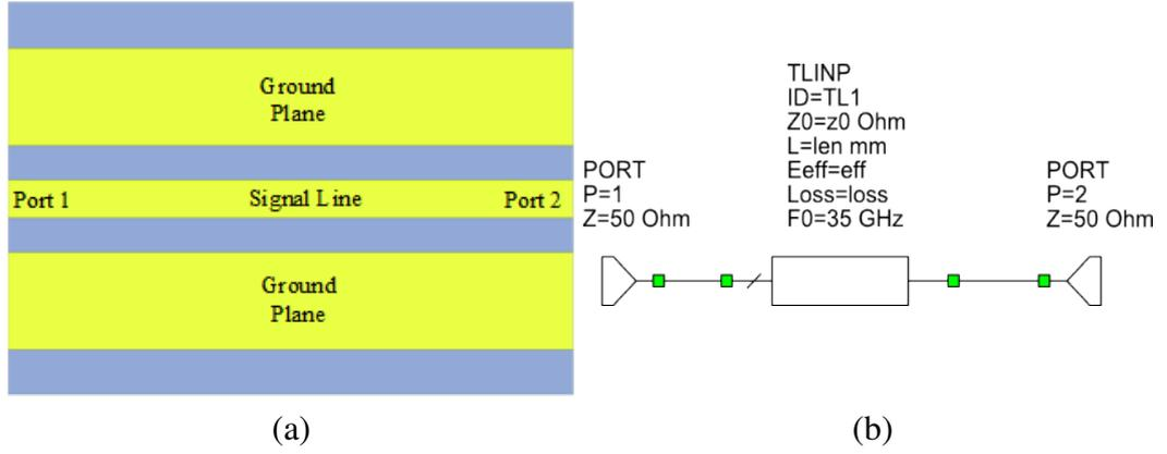
Figure 3.1: (a) 3D model and (b) transmission line model of a CWP .
