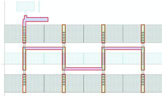
Figure 3.7: Layout of the second bit of the DMTL phase shifter.
