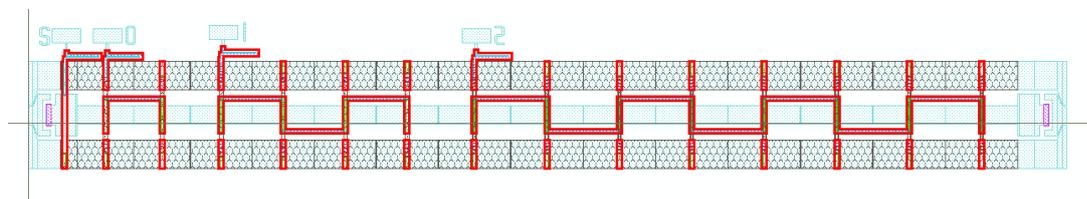
Figure 3.5: Layout of the overall 3 bit DMTL phase shifter.
