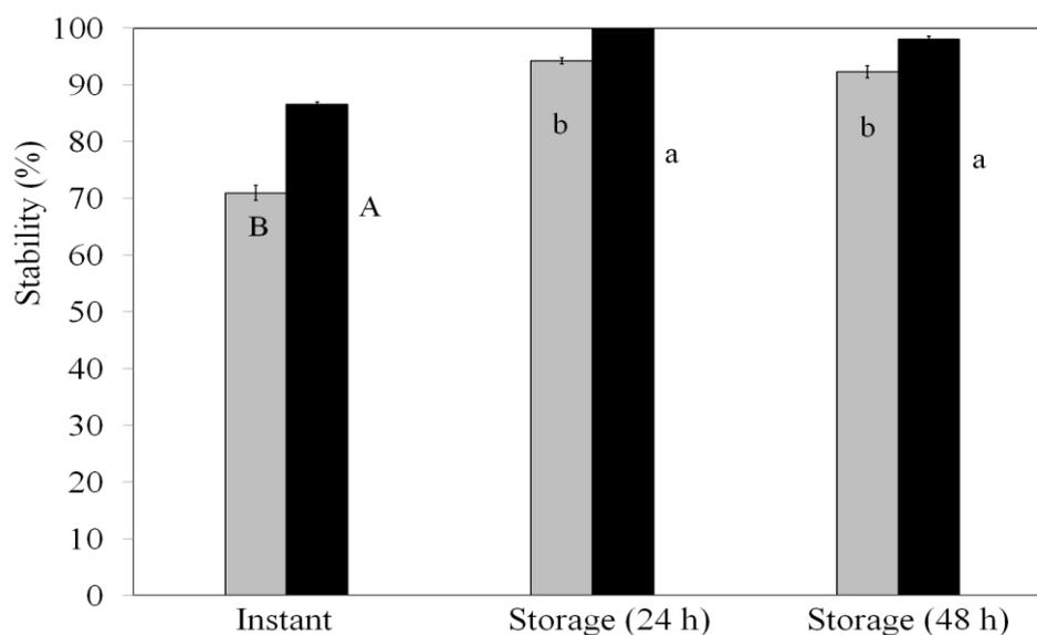
**Figure 3.15:** Effect of emulsion production method on stability of coated system; HSH (■) and US (■). Capital and small letters corresponds to individual statistical analysis. Bars with different letters represent significant difference ( $p \leq 0.05$ ).
