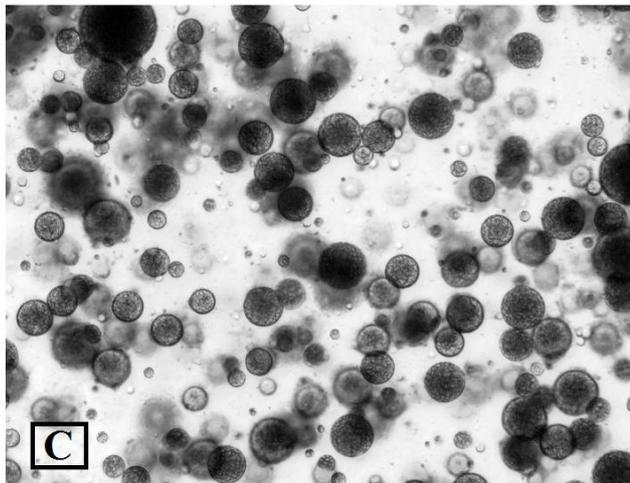
**Figure 3.5:** Microscopic images of double emulsions prepared by different homogenization methods: MF (A), US (B) and HSH (C).
