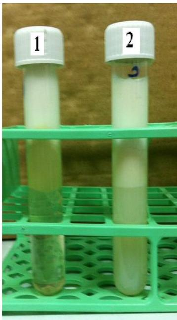
**Figure 3.16:** Separation of covered systems prepared with different stabilizers, by centrifugation force: 20% (w/w) gum arabic (1) and 7% (w/w) NaCN (2).
