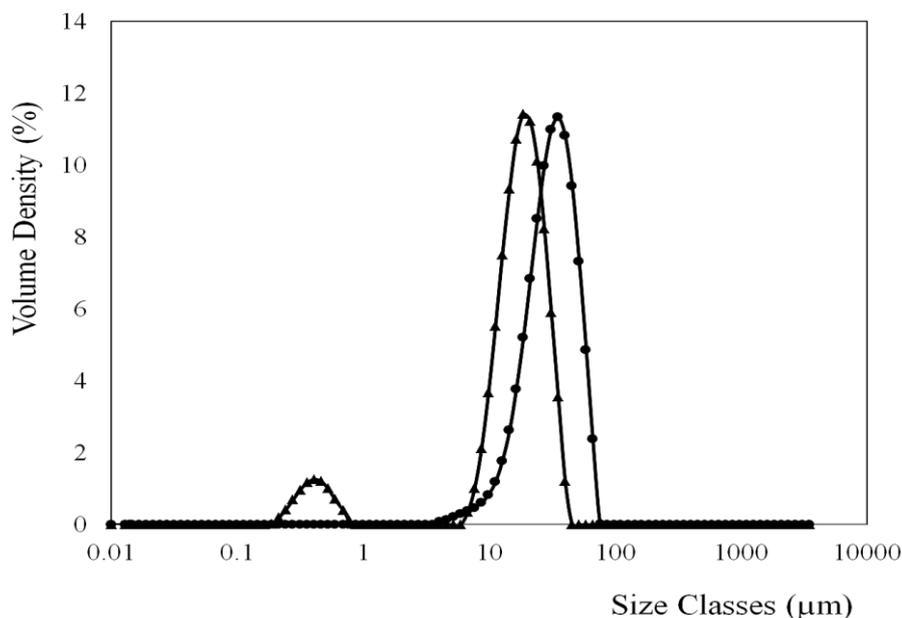
**Figure 3.2:** Droplet size distribution of double emulsions produced by HTFP (▲) and MS (●).
