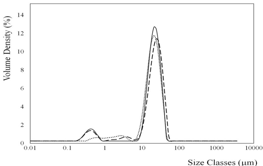
**Figure 3.8:** Effects of homogenization methods used in primary emulsion preparation on droplet size distribution when only PGPR was used as surfactant: HSH (—), US (- - -) and MF (·····).
