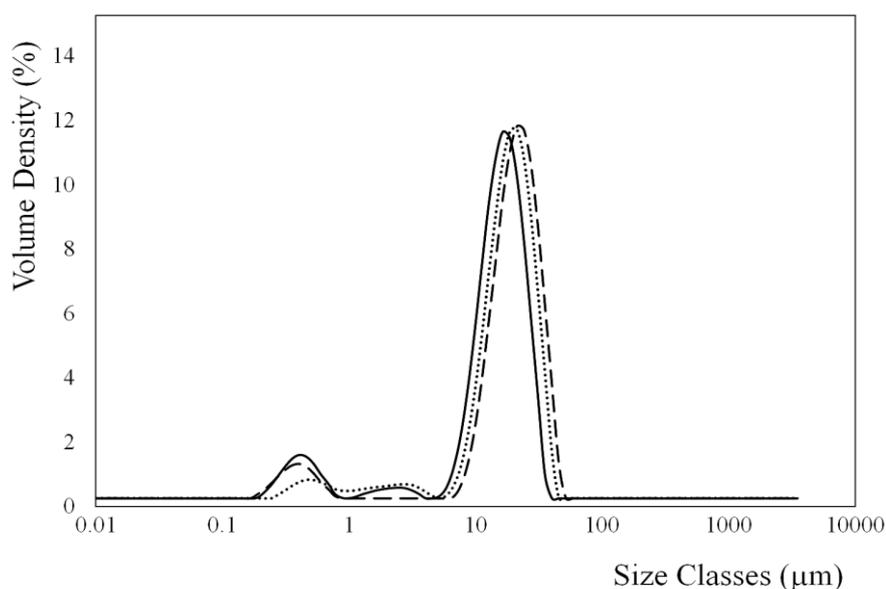
**Figure 3.7:** Effects of homogenization methods used in primary emulsion preparation on droplet size distribution when lecithin plus PGPR was used as surfactant: HSH (—), US (- - -) and MF (·····).
