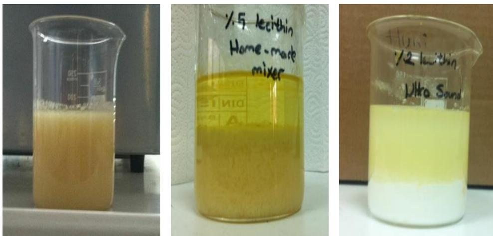
**A.** System containing 5% (w/w) lecithin prepared by HTFP just after preparation    **B.** System containing 5% (w/w) lecithin prepared by HTFP after 2 h storage    **C.** System containing 2% (w/w) lecithin prepared by US just after preparation
