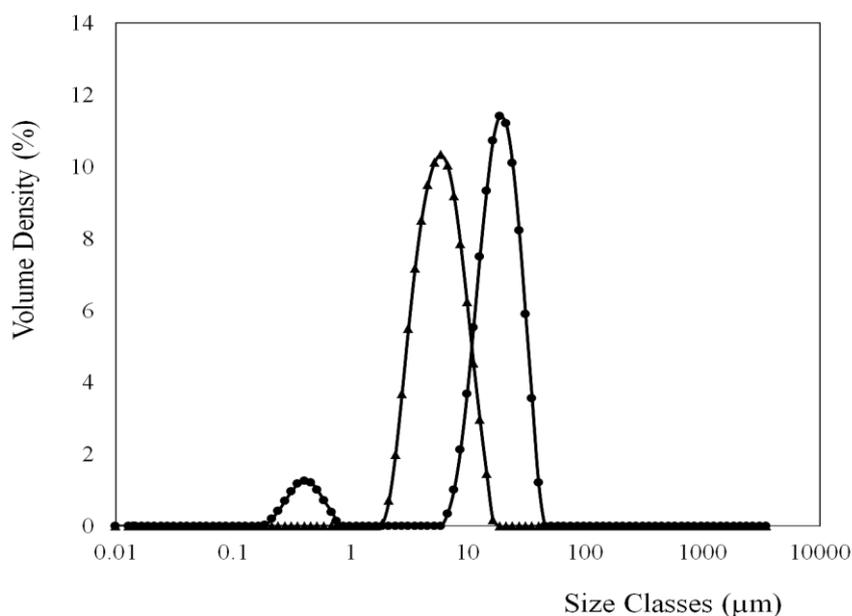
**Figure 3.3:** Droplet size distribution of emulsions with 11% (w/w) NaCN concentration: (●) and 15% (w/w) NaCN concentration: (▲).
