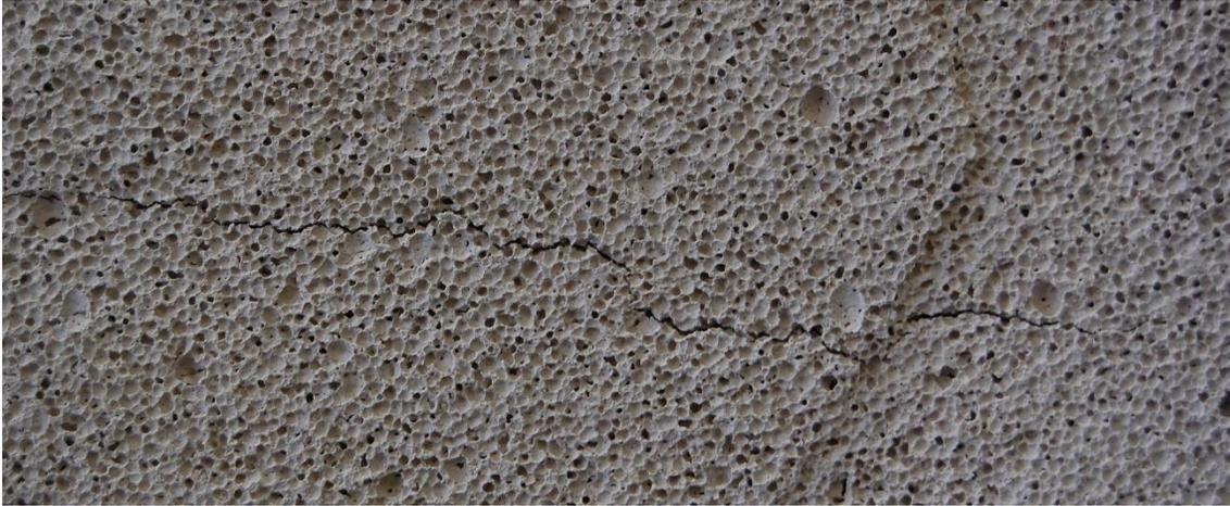
**Figure 4.22.** The macro view of the crack G2-e on the exposed G4 type AAC block (See in reference to Figure 4.17).
