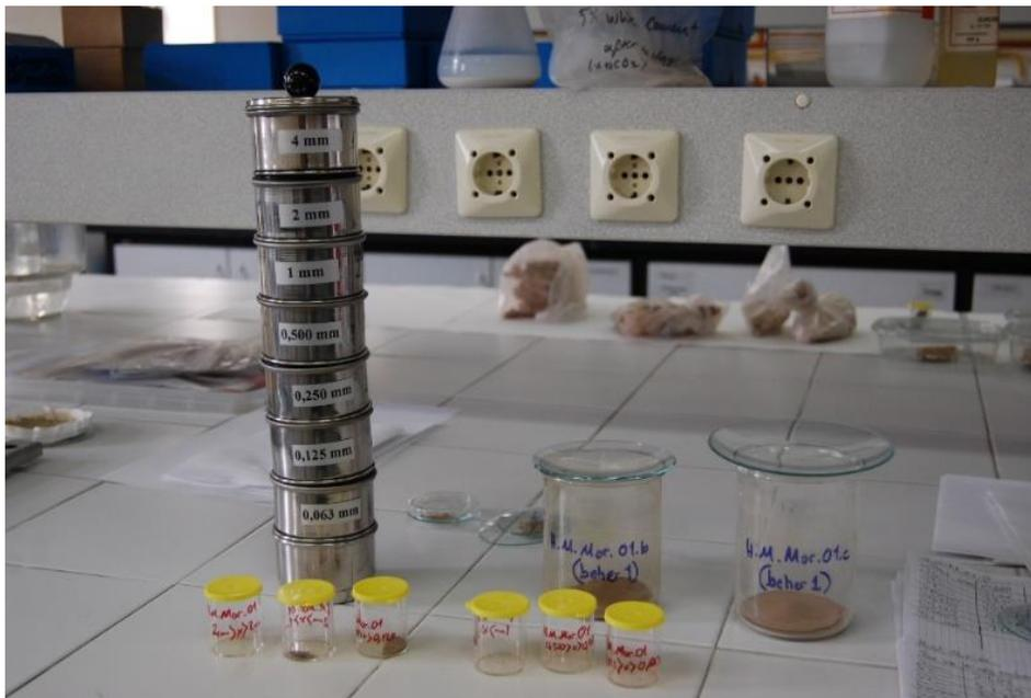
**Figure 3.03.** The sieves used for the sieve analysis in order to determine the particle size distribution of the mud brick, mud plaster and mud mortar samples.
