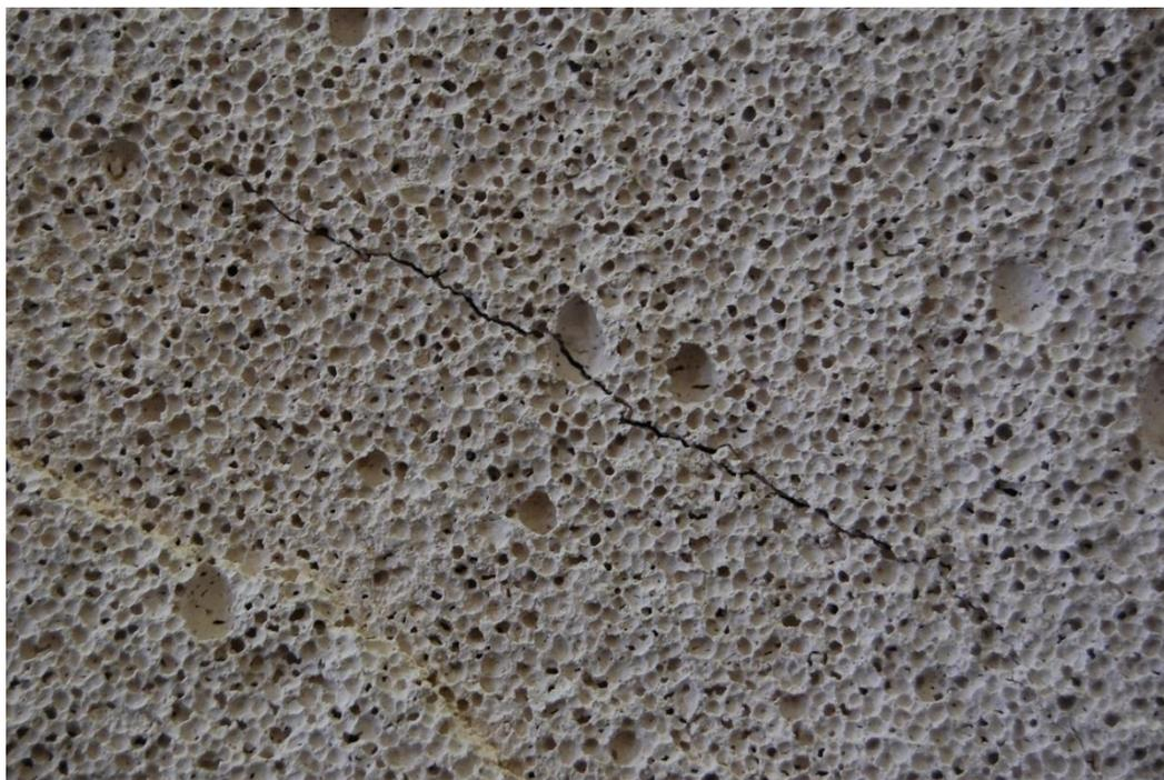
**Figure 4.21.** The macro view of the crack G2-d on the exposed G4 type AAC block (See in reference to Figure 4.17).
