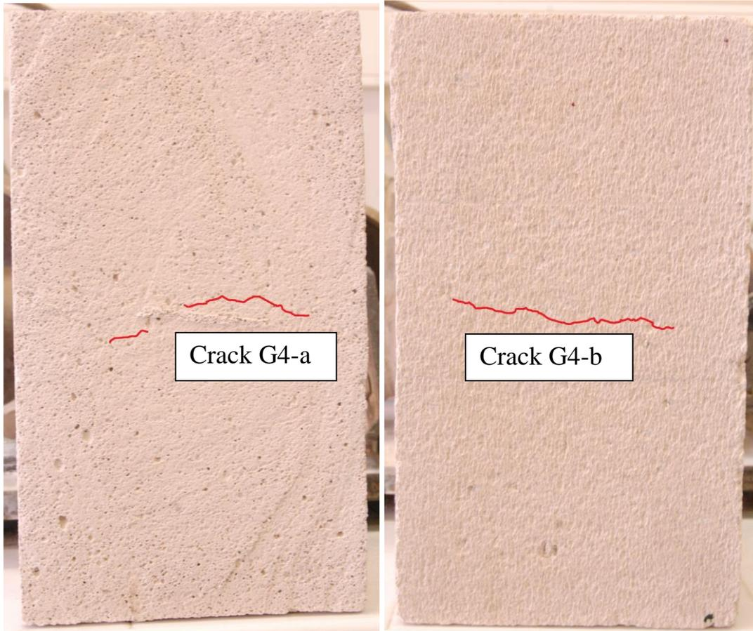
**Figure 4.25.** The horizontal and capillary cracks occurred parallel to the diffusion direction and visible on the G4 type AAC block after exposed to 20% CO<sub>2</sub> and 100% relative humidity for a period of three weeks (highlighted in red).
