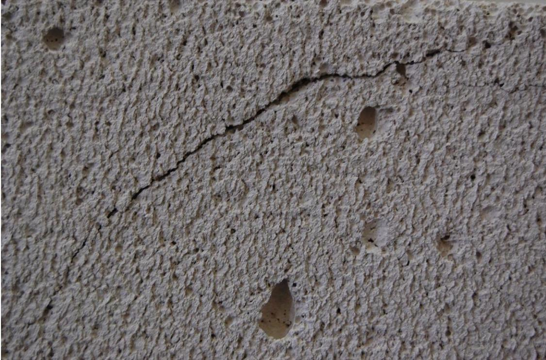
**Figure 4.18.** The macro view of the crack G2-a on the exposed G4 type AAC block (See in reference to Figure 4.17).
