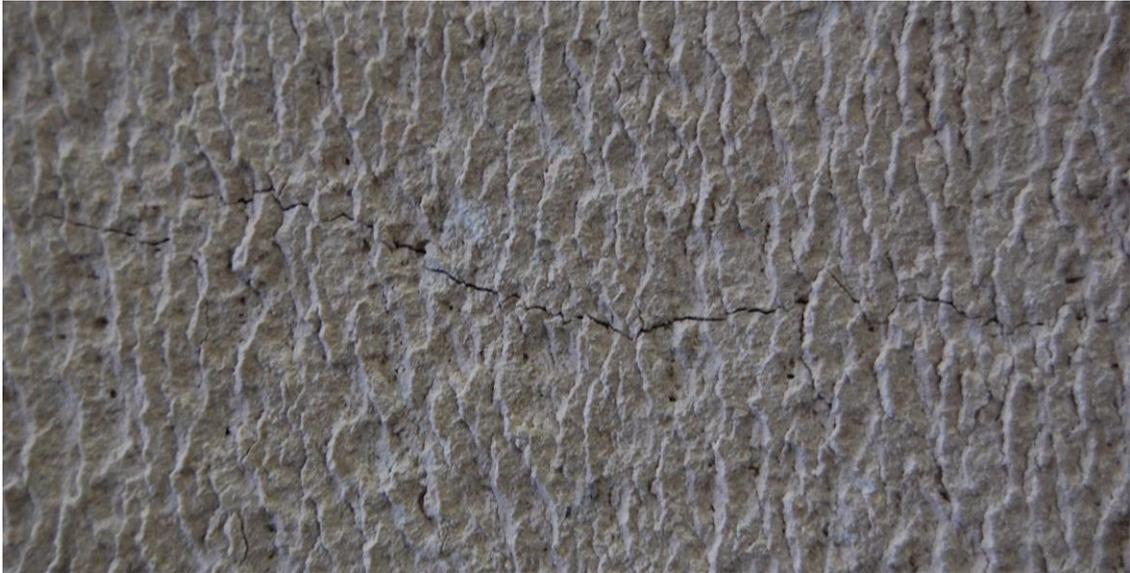
**Figure 4.27.** The macro view of the crack G4-b on the exposed G4 type AAC block (See in reference to Figure 4.25).
