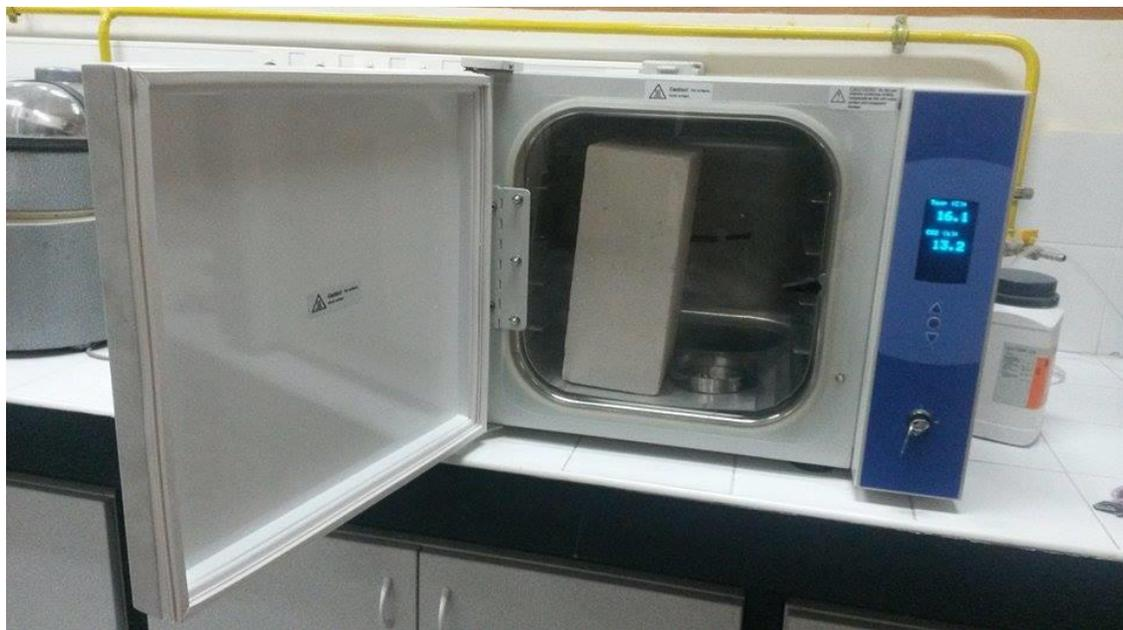
**Figure 3.14.** The CO<sub>2</sub> desiccator in which the AAC samples were exposed to 20% CO<sub>2</sub> concentration and 100% relative humidity.
