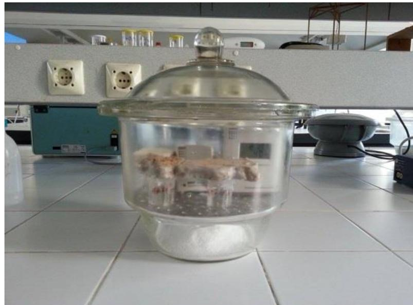
**Figure 3.06.** The experimental set up for the water vapor permeability tests in accordance with the related standards
