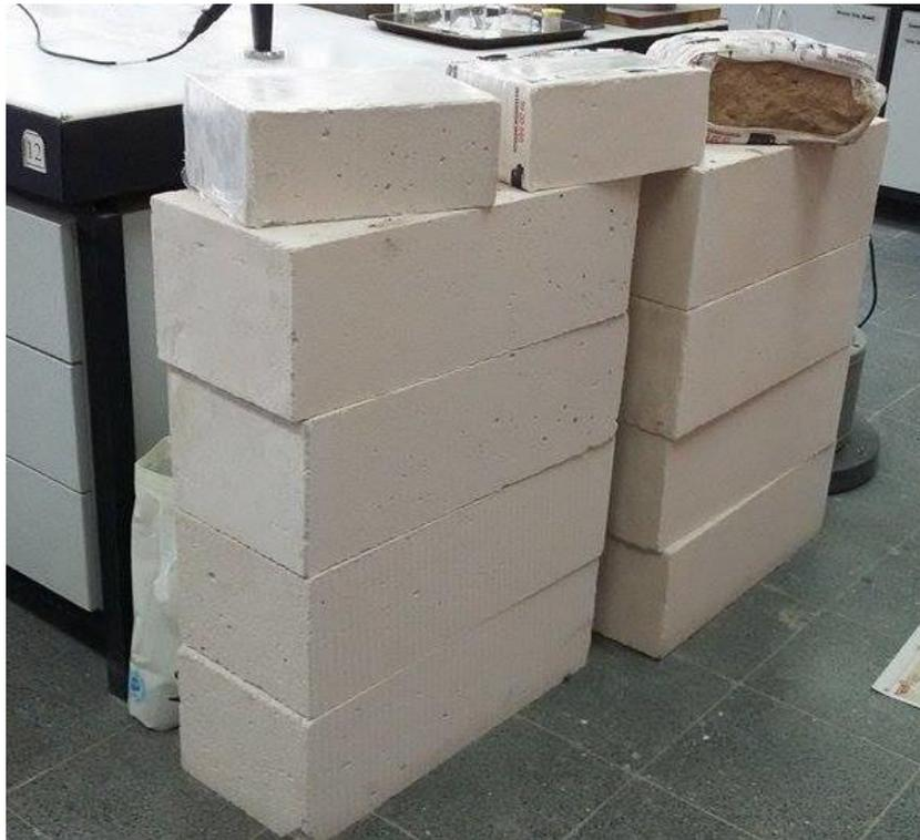
**Figure 3.02.** The G2 and G4 type AAC samples provided from a local producer and cut to the same size as mud brick from Hamzalı Village.
