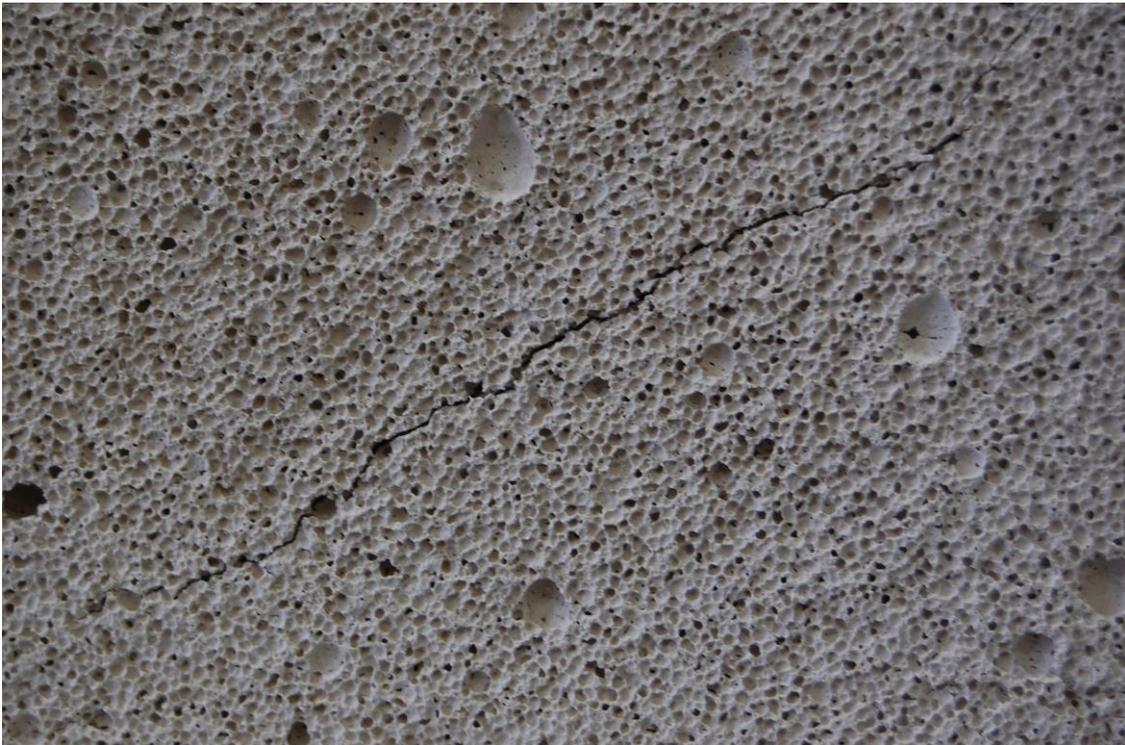
**Figure 4.23.** The macro view of the crack G2-f on the exposed G4 type AAC block (See in reference to Figure 4.17).
