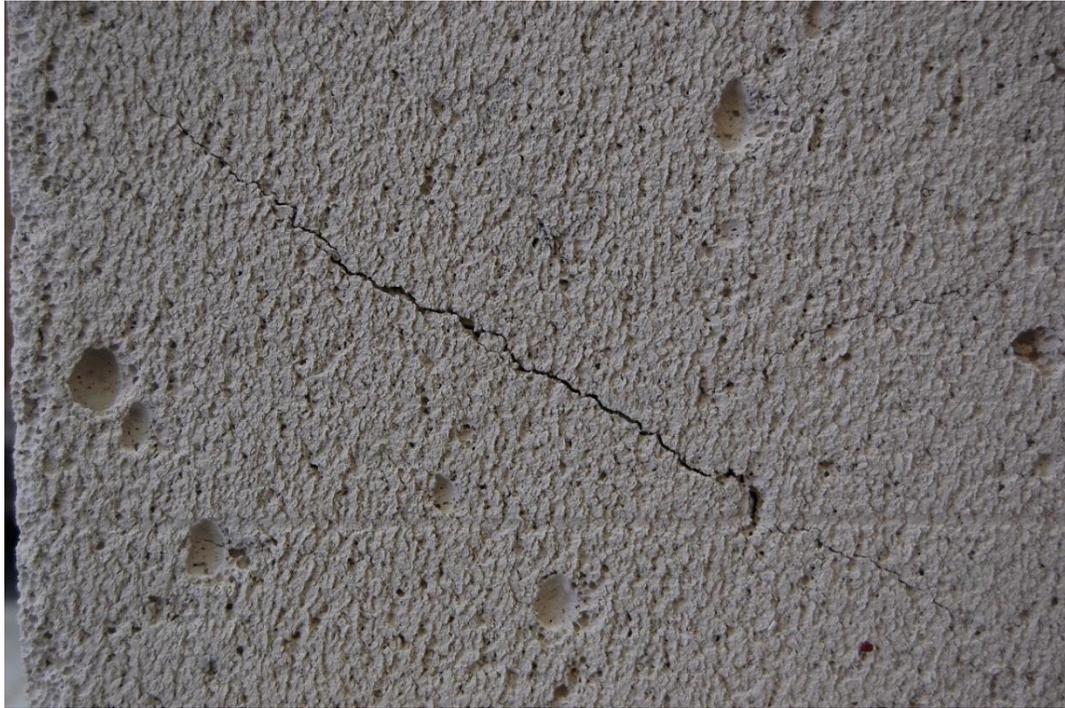
**Figure 4.20.** The macro view of the crack G2-c on the exposed G4 type AAC block (See in reference to Figure 4.17).
