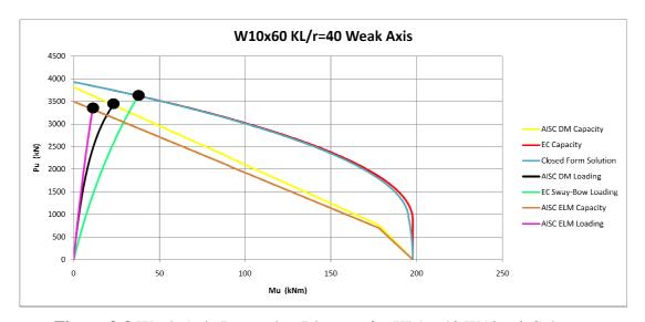
**Figure 3-9** Weak Axis Interaction Diagram for KL/r= 40 W10x60 Column
