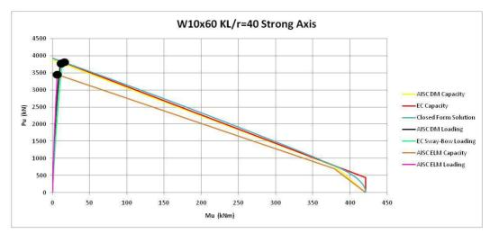
Figure 4-5 Strong Axis Interaction Diagram for  $\frac{KL}{r} = 40 \text{ W} 10x60 \text{ Column}$
