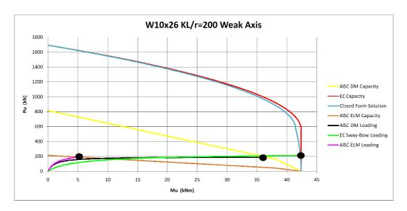
Figure 3-23 Weak Axis Interaction Diagram for KL/r= 200 W10x26 Column
