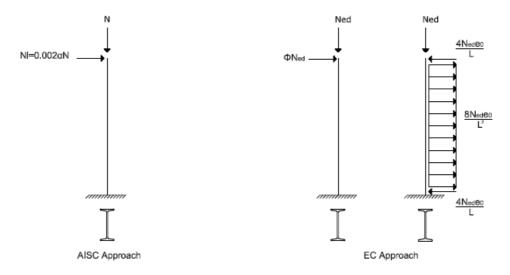
Figure 3-2 Members Under Weak Axis Bending with Compression
