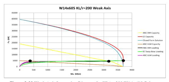
Figure 3-33 Weak Axis Interaction Diagram for KL/r= 200 W14x605 Column
