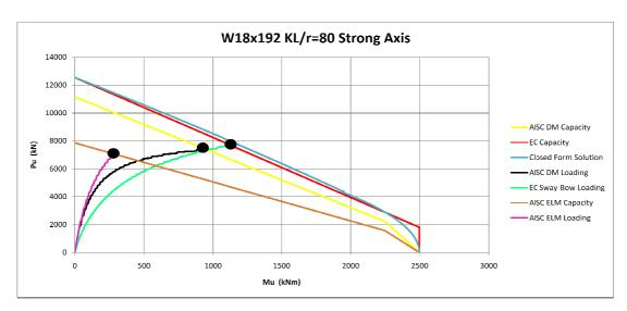
Figure 3-35 Strong Axis Interaction Diagram for KL/r=80 W18x192 Column
