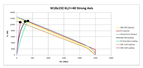
Figure 3-34 Strong Axis Interaction Diagram for KL/r=40 W18x192 Column
