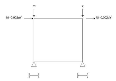
Figure 4-1 Loading of Plane Frame with AISC360 provisions
