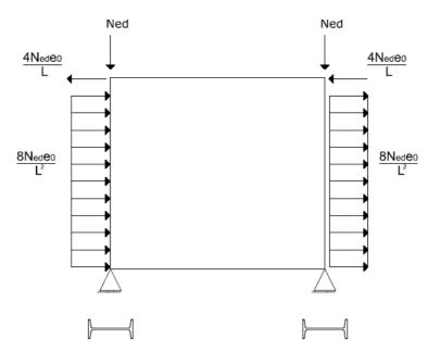
**Figure 4-3** Bow Imperfection Loading for Plane Frame (EC3 Direction)
