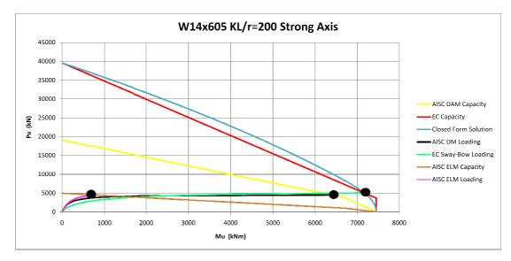
Figure 3-28 Strong Axis Interaction Diagram for KL/r=200 W14x605 Column
