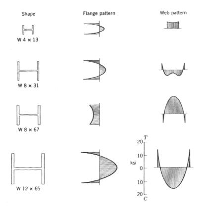
**Figure 1-4** Initial Residual Stress Distribution of Sections (Adopted from Guide to Stability Design Criteria for Metal Structures)
