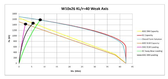
Figure 3-19 Weak Axis Interaction Diagram for KL/r= 40 W10x26 Column
