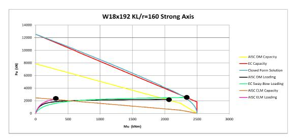
Figure 3-37 Strong Axis Interaction Diagram for KL/r=160 W18x192 Column
