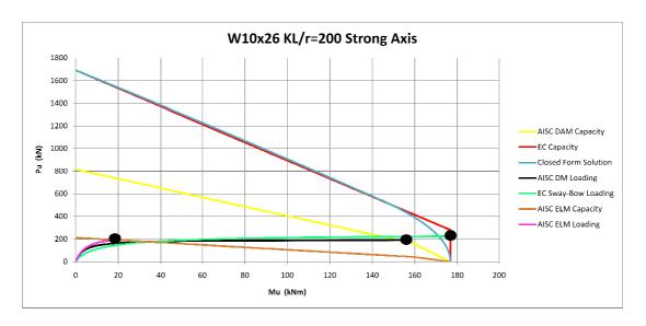
Figure 3-18 Strong Axis Interaction Diagram for KL/r=200 W10x26 Column
