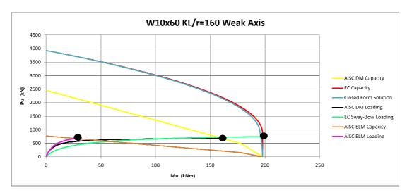
**Figure 3-12** Weak Axis Interaction Diagram for KL/r= 160 W10x60 Column
