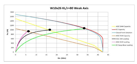
Figure 3-20 Weak Axis Interaction Diagram for KL/r= 80 W10x26 Column
