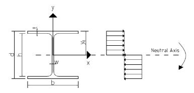
Figure 1-1 Stress Distribution of I Shape Subjected to Pure Bending
