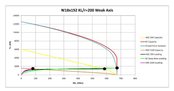
Figure 3-43 Weak Axis Interaction Diagram for KL/r= 200 W18x192 Column
