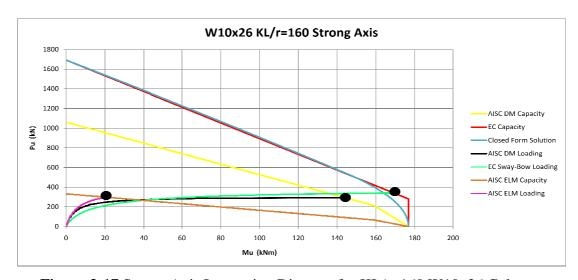
**Figure 3-17** Strong Axis Interaction Diagram for KL/r=160 W10x26 Column
