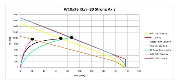
Figure 3-15 Strong Axis Interaction Diagram for KL/r=80 W10x26 Column
