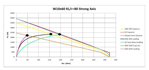
Figure 3-5 Strong Axis Interaction Diagram for KL/r=80 W10x60 Column
