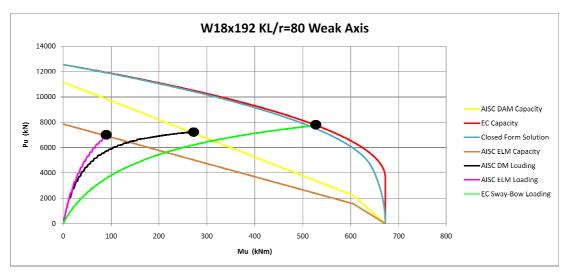
Figure 3-40 Weak Axis Interaction Diagram for KL/r= 80 W18x192 Column
