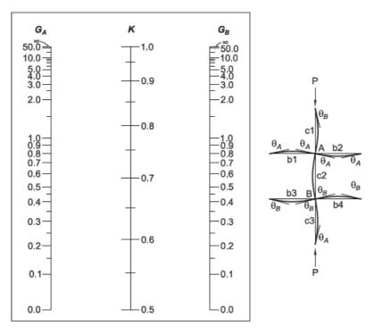
Figure 1-7 Alignment Chart-Sidesway Inhibited (Adopted from AISC 360-10)
