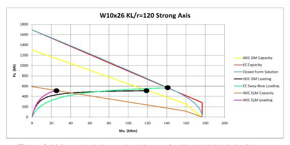
Figure 3-16 Strong Axis Interaction Diagram for KL/r=120 W10x26 Column
