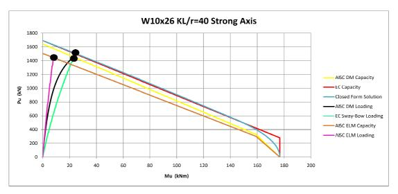
Figure 3-14 Strong Axis Interaction Diagram for KL/r=40 W10x26 Column
