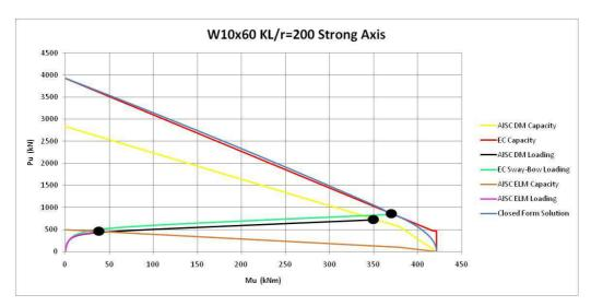
**Figure 4-9** Strong Axis Interaction Diagram for  $\frac{KL}{r} = 200 \text{ W} 10x60 \text{ Column}$
