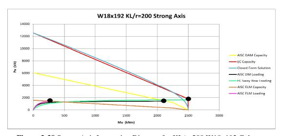
Figure 3-38 Strong Axis Interaction Diagram for KL/r=200 W18x192 Column
