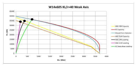
Figure 3-29 Weak Axis Interaction Diagram for KL/r= 40 W14x605 Column
