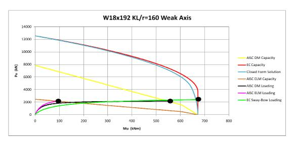
Figure 3-42 Weak Axis Interaction Diagram for KL/r= 160 W18x192 Column
