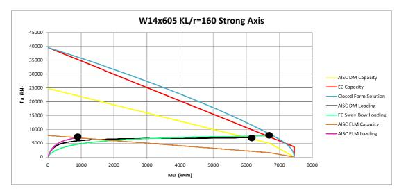
**Figure 3-27** Strong Axis Interaction Diagram for KL/r=160 W14x605 Column
