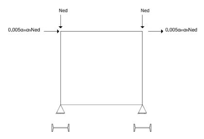
Figure 4-2 Sway Imperfection Loading for Plane Frame (EC3 Direction)
