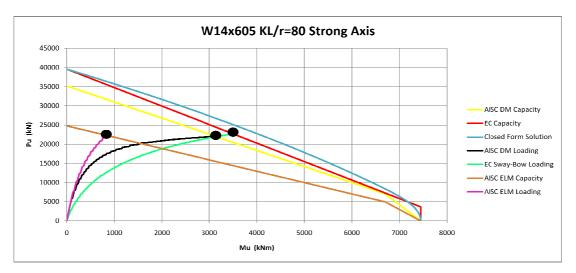
Figure 3-25 Strong Axis Interaction Diagram for KL/r=80 W14x605 Column
