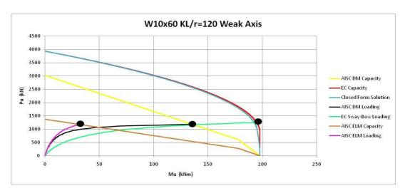
**Figure 3-11** Weak Axis Interaction Diagram for KL/r= 120 W10x60 Column
