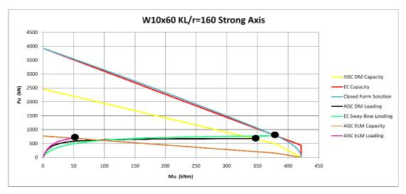
Figure 3-7 Strong Axis Interaction Diagram for KL/r=160 W10x60 Column
