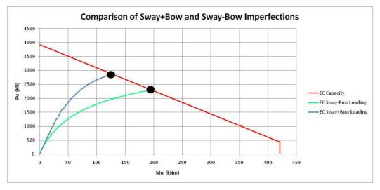
**Figure 3-3** Comparison of EC3 Sway-Bow and Sway+Bow Loadings for KL/r=80 W10x60 Column
