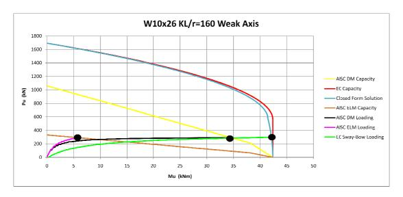
Figure 3-22 Weak Axis Interaction Diagram for KL/r= 160 W10x26 Column
