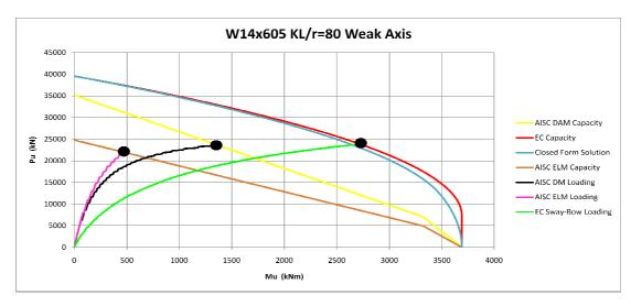
Figure 3-30 Weak Axis Interaction Diagram for KL/r= 80 W14x605 Column
