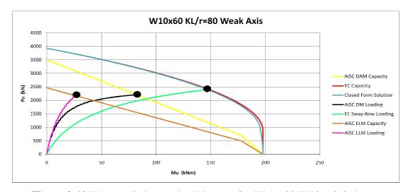
Figure 3-10 Weak Axis Interaction Diagram for KL/r= 80 W10x60 Column
