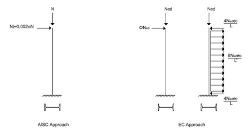
Figure 1-5 Notional Loads for AISC360 and EC3 specifications
