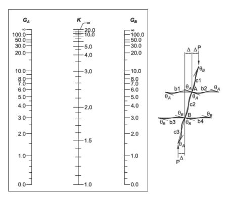
Figure 1-8 Alignment Chart-Sidesway Permitted (Adopted from AISC 360-10)
