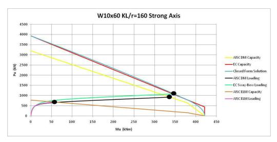
**Figure 4-8** Strong Axis Interaction Diagram for  $\frac{KL}{r} = 160 \text{ W} 10x60 \text{ Column}$
