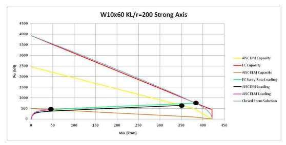
**Figure 4-10** Strong Axis Interaction Diagram for  $\frac{KL}{r} = 200$  Column (K=2.5)
