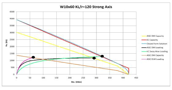
Figure 3-6 Strong Axis Interaction Diagram for KL/r=120 W10x60 Column
