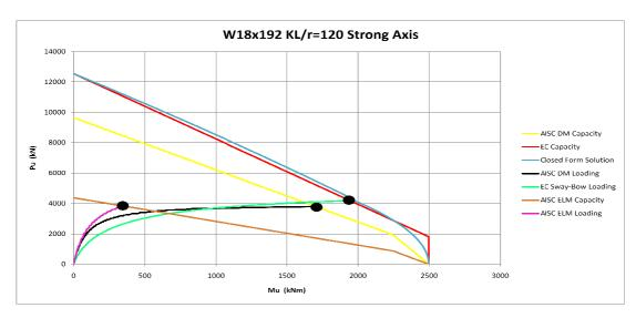
Figure 3-36 Strong Axis Interaction Diagram for KL/r=120 W18x192Column
