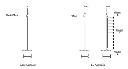
Figure 3-1 Members Under Strong Axis Bending with Compression
