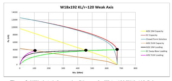
**Figure 3-41**Weak Axis Interaction Diagram for KL/r= 120 W18x192 Column
