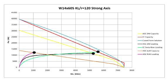
Figure 3-26 Strong Axis Interaction Diagram for KL/r=120 W14x605 Column
