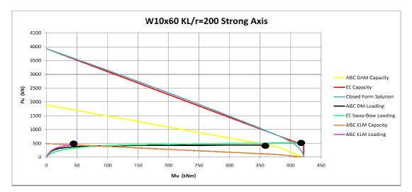
Figure 3-8 Strong Axis Interaction Diagram for KL/r=200 W10x60 Column
