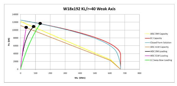
**Figure 3-39** Weak Axis Interaction Diagram for KL/r= 40 W18x192 Column
