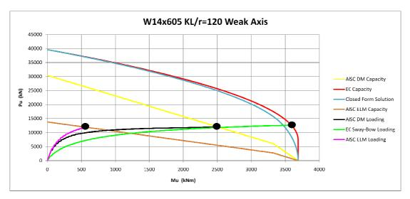
Figure 3-31 Weak Axis Interaction Diagram for KL/r= 120 W14x605 Column
