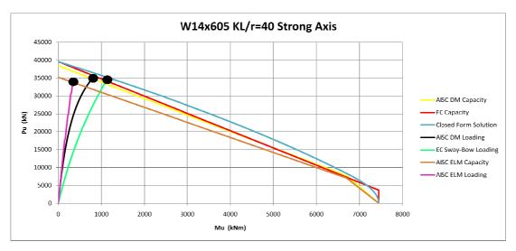
Figure 3-24 Strong Axis Interaction Diagram for KL/r=40 W14x605 Column
