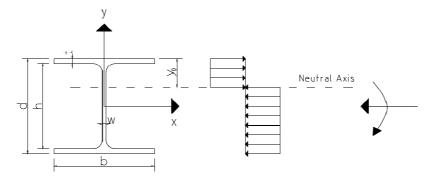
Figure 1-3 Stress Distribution of I Shape Subjected to Bending with Compression
