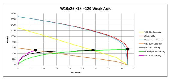
**Figure 3-21** Weak Axis Interaction Diagram for KL/r= 120 W10x26 Column
