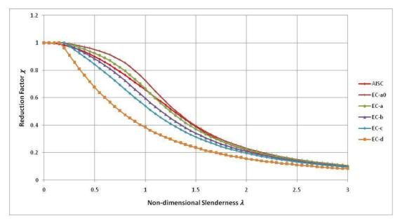
**Figure 1-9** Comparison of Reduction Factors Given in AISC360-10 and EC3 for Flexural Buckling
