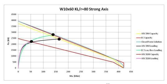
**Figure 4-6** Strong Axis Interaction Diagram for  $\frac{KL}{r} = 80 \text{ W} 10x60 \text{ Column}$
