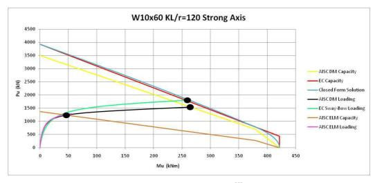
**Figure 4-7** Strong Axis Interaction Diagram for  $\frac{KL}{r} = 120 \text{ W}10x60 \text{ Column}$
