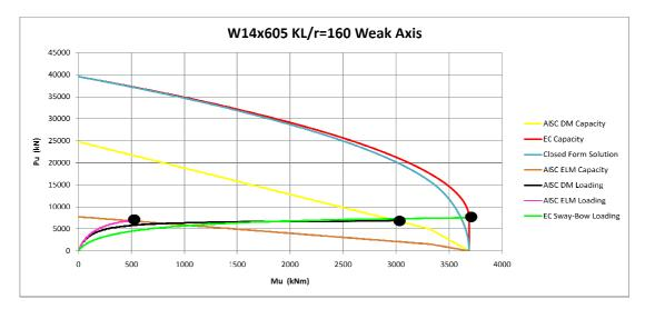
Figure 3-32 Weak Axis Interaction Diagram for KL/r= 160 W14x605 Column
