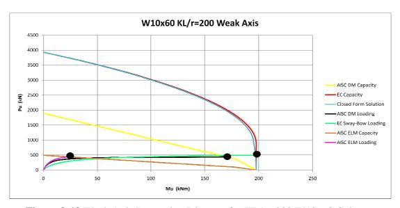
Figure 3-13 Weak Axis Interaction Diagram for KL/r= 200 W10x60 Column
