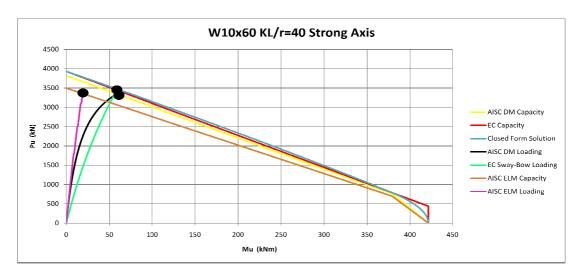
Figure 3-4 Strong Axis Interaction Diagram for KL/r=40 W10x60 Column
