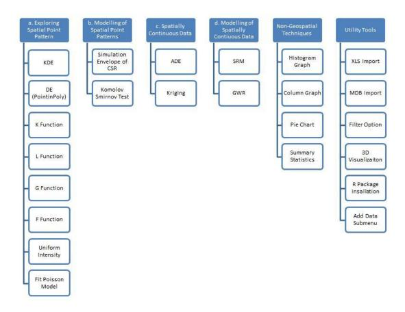
Figure 47. Geospatial, Non-geospatial and Utility Tools which are Integrated into GIS Software
