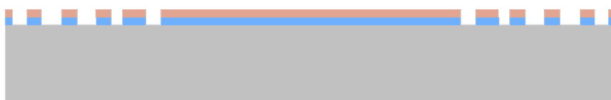
(b) The SiO 2 is patterned using wet etching.
