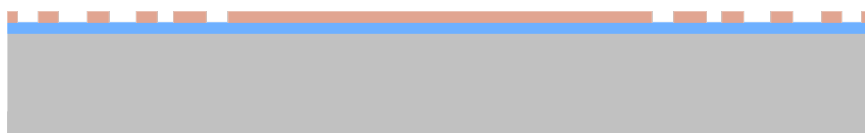
(a) The PR is patterned by through 1st mask.
