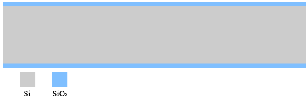
(a) The Si wafer with 2\mu m SiO 2 layer
