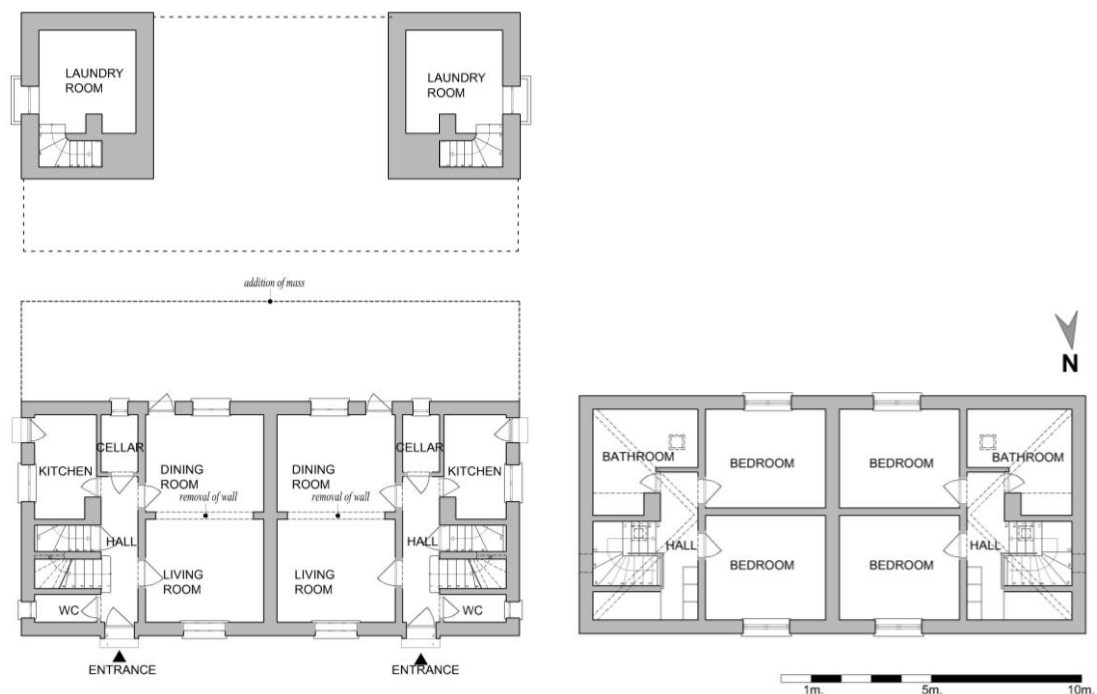
Figure 3.32: Ground floor and first floor plans of Employee Dwelling Type 3
