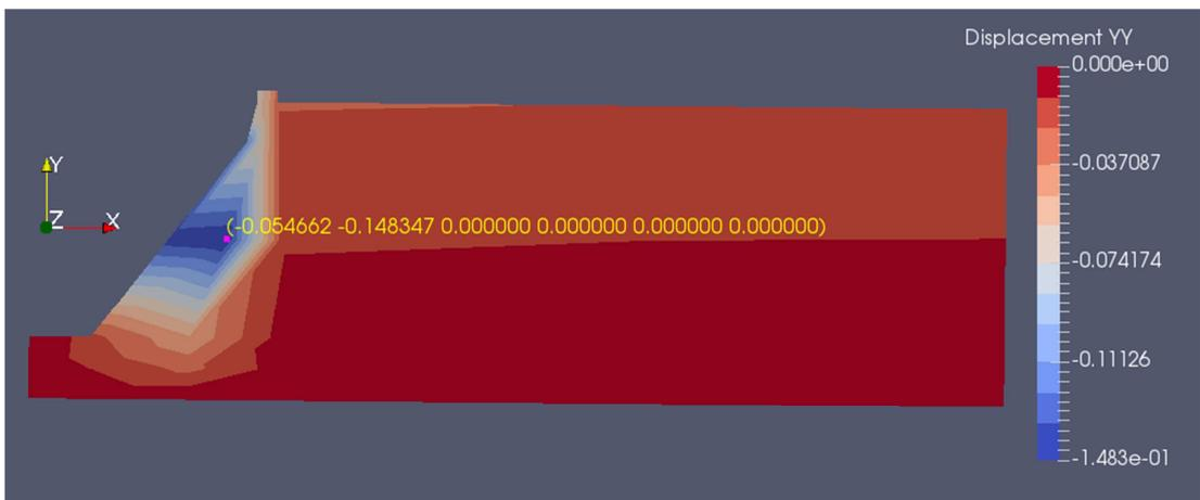
Figure B.18. Displacements on Y direction by Zargana
