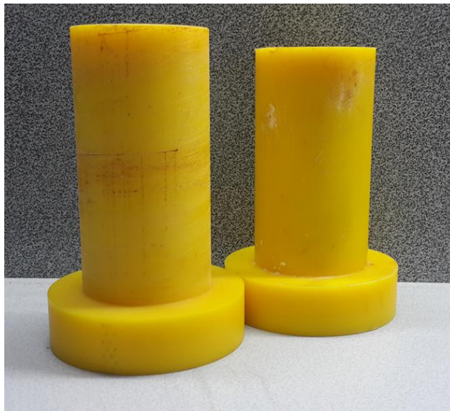
Figure 3.20 Spacers used to compact samples
