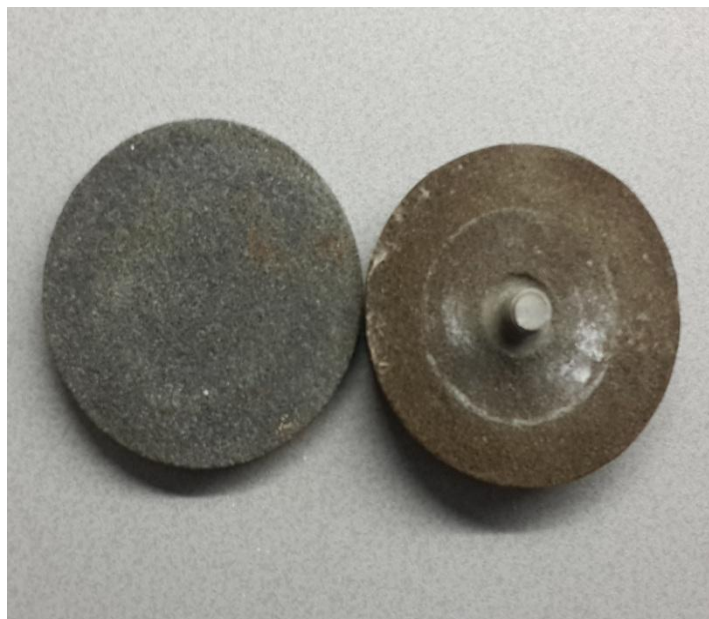
Figure 3.18 Porous disks used through the study
