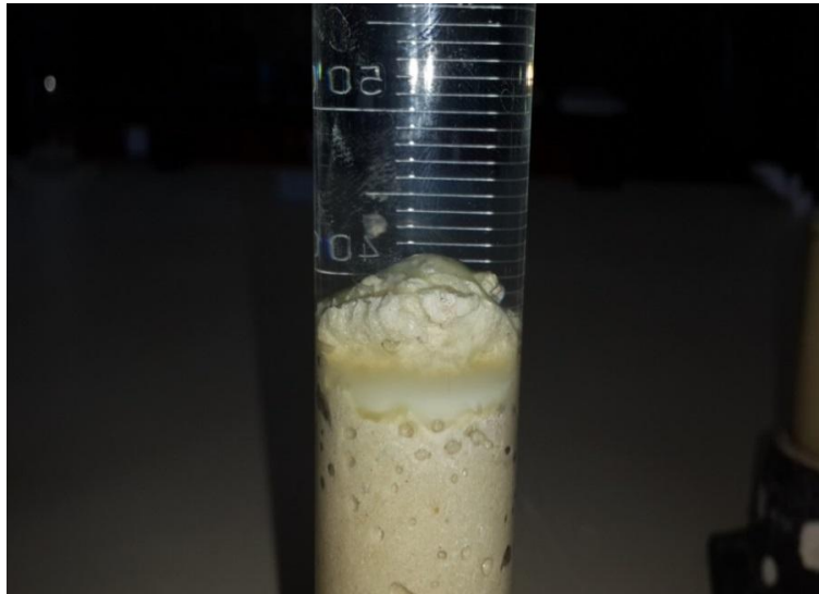
Figure 3.23 Formation of mud which prevent water penetration into lower layers
