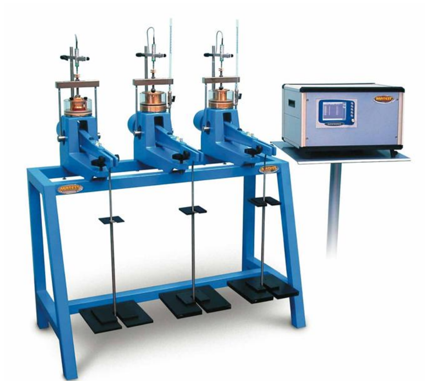
Figure 3.27 A view of conventional consolidometer setup
