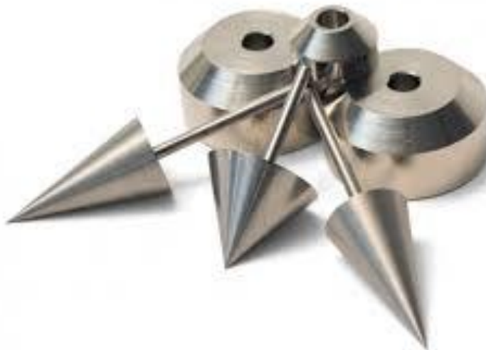
Figure 3.8 Fall cone masses and cones used to determine LL and PL
