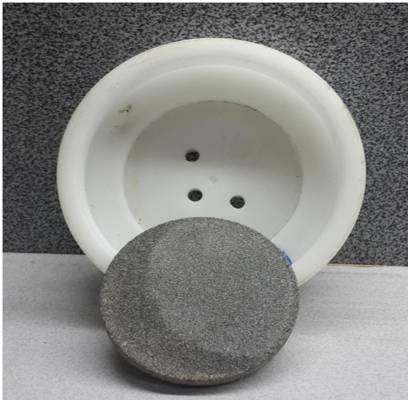
Figure 3.15 The base with ring-shaped porous disk
