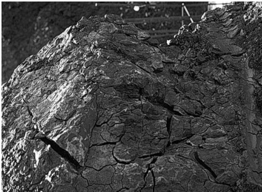
Figure 2.13 Interconnected shrinkage cracks extend from the ground surface into the active zone (Petry, 2000)
