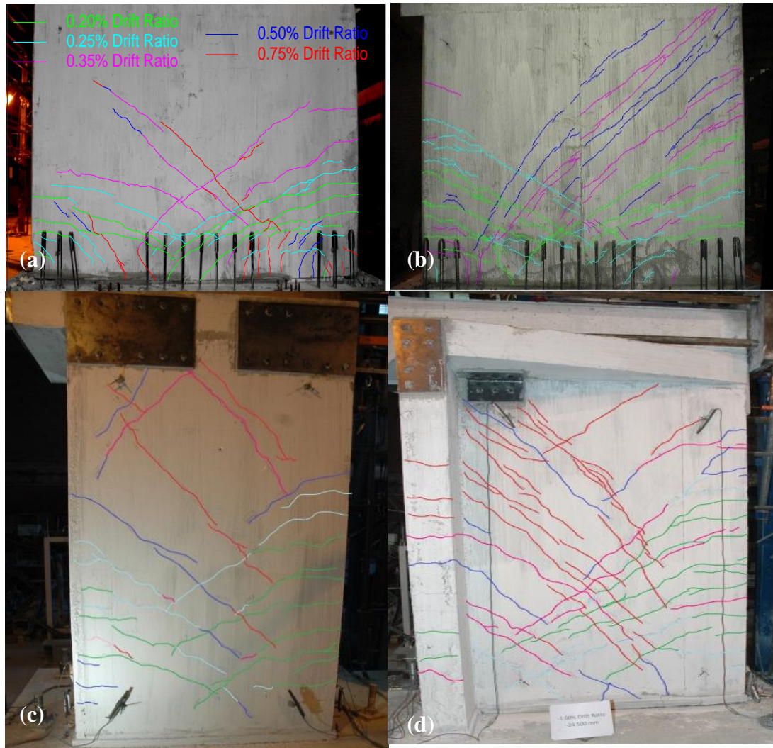
Figure 2-7: Cracks Observed for; (a) Specimen 1; (b) Specimen 2, (c) Specimen 3, (d) Specimen 4 (Binici and Canbay, 2014)
