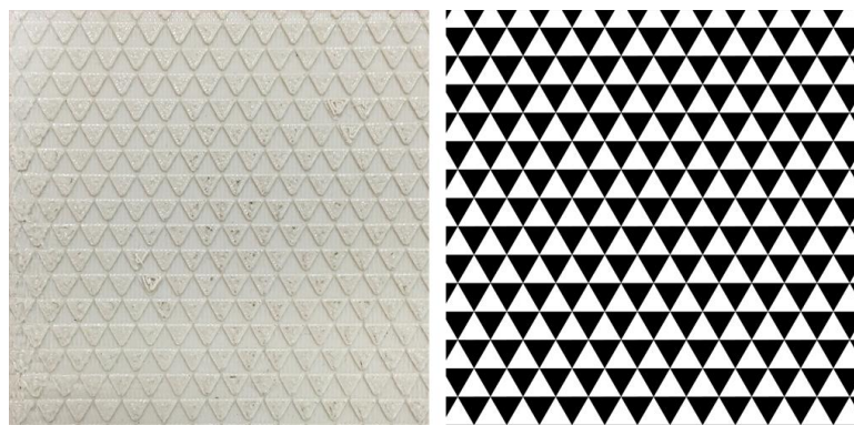
Figure 5.14 Left: Manufactured Surface Texture of YD-09, Right: Bitmap Representation of YD-09.
