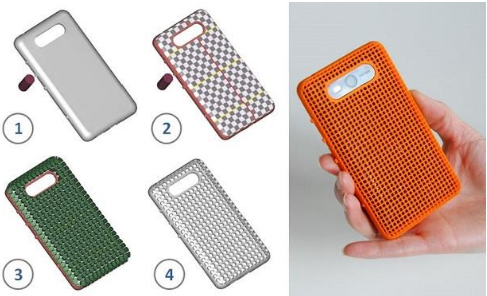
Figure 4.11 3D surface texturing method with the utilization of a 3D texture mesh in 3-matic STL Texturing Module (“3-matic Texturing Module,” n.d.)
