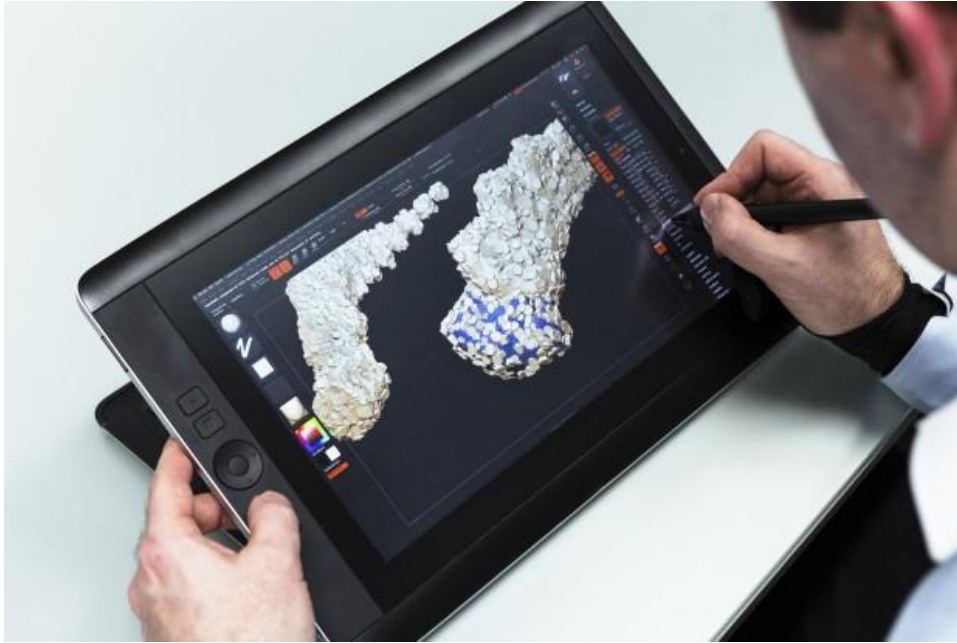
Figure 4.13 Wacom Cintiq Companion Tablet with Pressure Sensitive Stylus for virtual clay modelling in ZBrush (“ZBrush,” n.d.)
