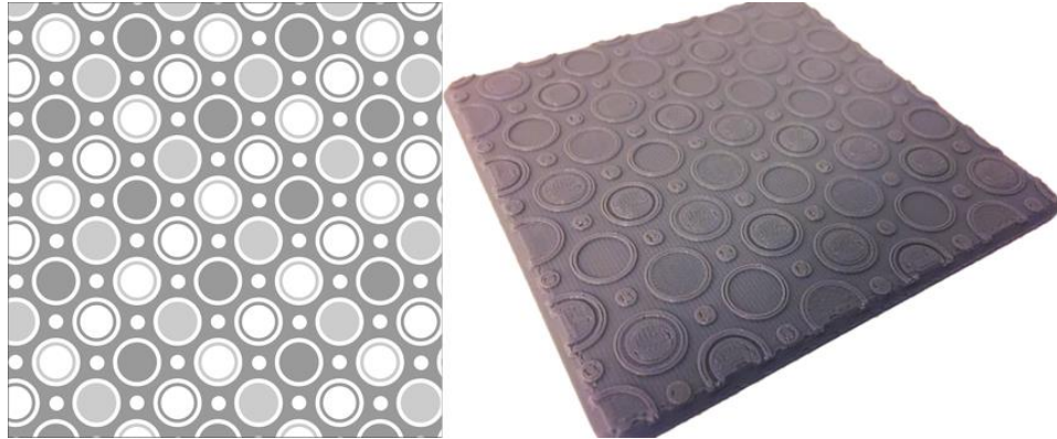
Figure 4.2 Bitmap image is on the left, the 3D surface texture created with the bitmap image is on the right
