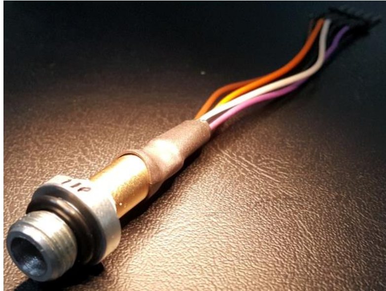
Figure 5.13 - Assembled view of the hydraulic pressure sensor.
