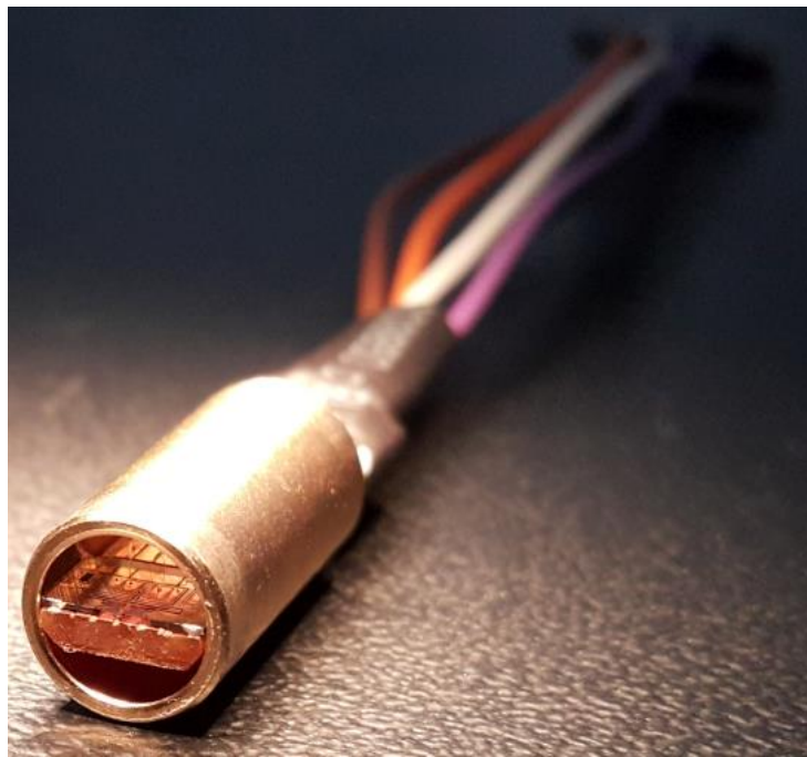
Figure 5.10 - Close up view of a sensor inside the cylinder with its electrical connections completed.
