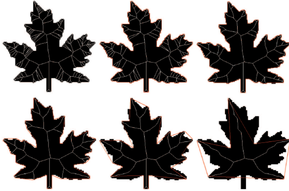
Figure 3.2: Skeleton extraction with respect to the polygonal approximation contour segments obtained by the DCE. (Illustration is taken from [2])
