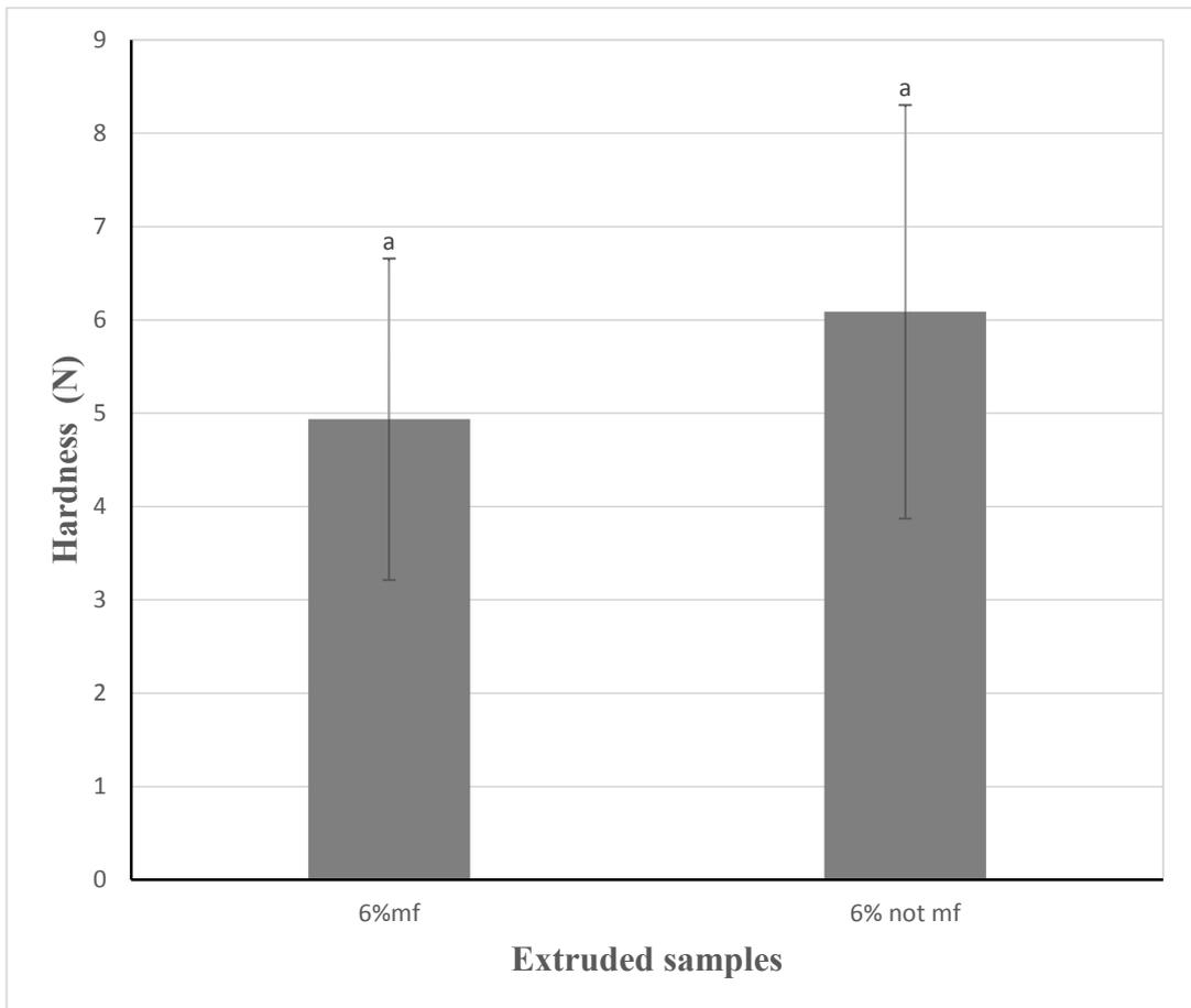
**Figure 16** Comparison of microfluidized onion skin and non - microfluidized onion skin addition on the third highest hardness values of the extruded samples (measured with the puncture probe). Results are means  $\pm$  SD (n=20).
