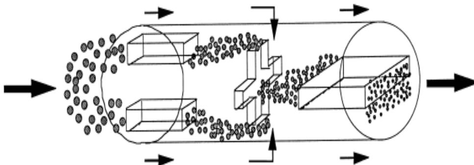
**Figure 1.** Symbolic configuration of the microfluidization process (Lagoueyte & Paquin, 1998).
