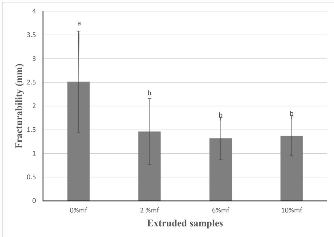
**Figure 7** Effect of microfluidized onion skin addition on fracturability of extruded samples (measured with the sharp blade probe). Results are means  $\pm$  SD (n= 10).
