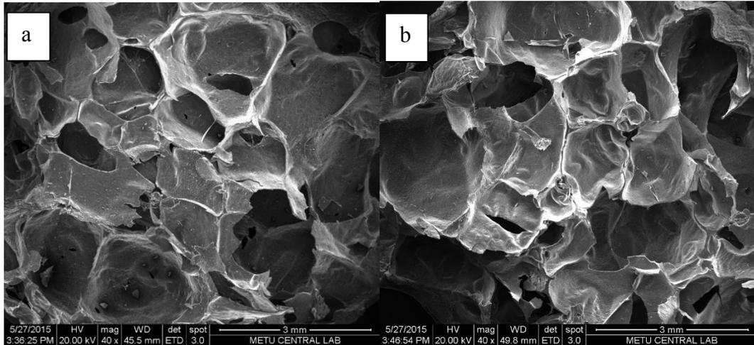
**Figure 5** Scanning electron microscopy images of extrudates with 40X magnification A) 6% microfluidized onion skin added sample B) 6% non microfluidized onion skin added sample.
