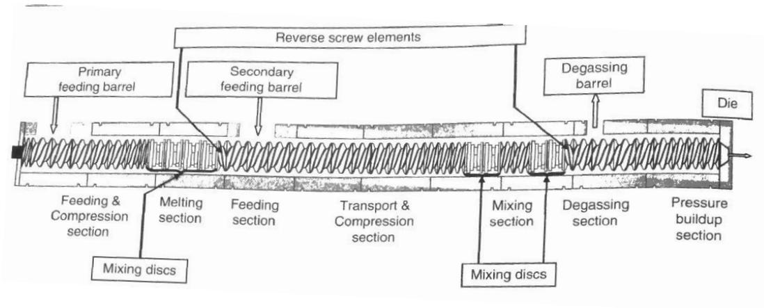
**Figure 3** Screw- barrel assembly of the twin- screw extruder (Bouvier & Campanella, 2014).
