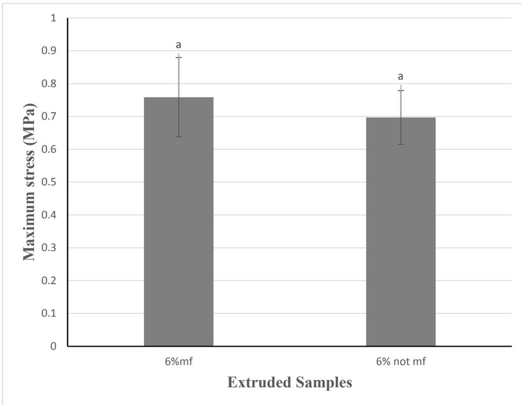
**Figure 8** Comparison of microfluidized onion skin and non - microfluidized onion skin addition on maximum stress of the extruded samples (measured with the sharp blade probe). Results are means  $\pm$  SD (n=10).
