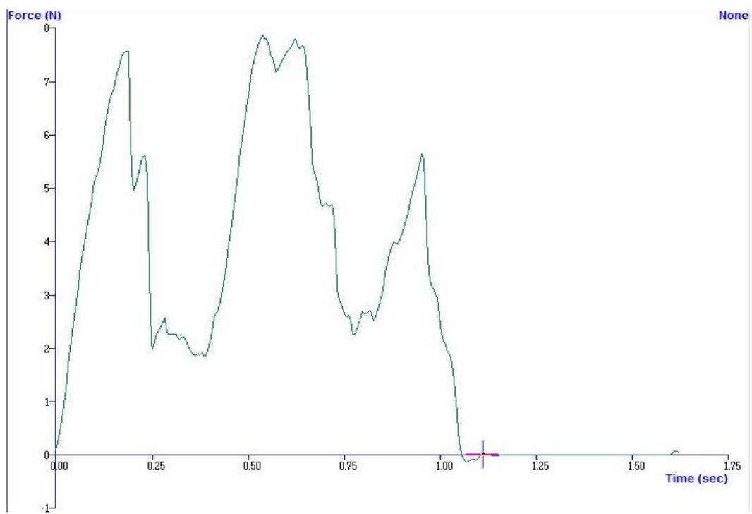
**Figure 28** Sample force time curve of 6%not mf onion skin added sample
