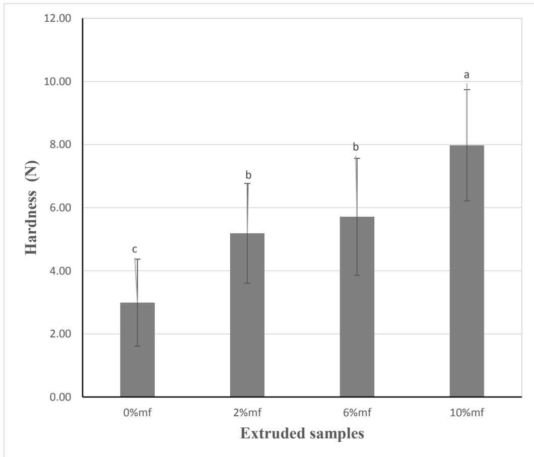
**Figure 11** Effect of microfluidized onion skins addition on the second highest hardness values of extruded samples (measured with the puncture probe). Results are means  $\pm$  SD (n= 20).
