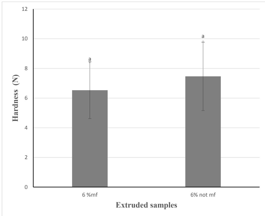
**Figure 14** Comparison of microfluidized onion skin and non - microfluidized onion skin addition on the first highest hardness values of the extruded samples (measured with the puncture probe). Results are means  $\pm$  SD (n=20).
