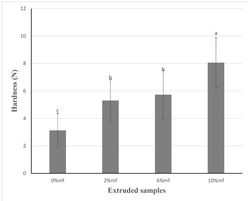
**Figure 13** Effect of microfluidized onion skins addition based on the average of maximum three hardness values of extruded samples (measured with the puncture probe). Results are means  $\pm$  SD (n= 20).
