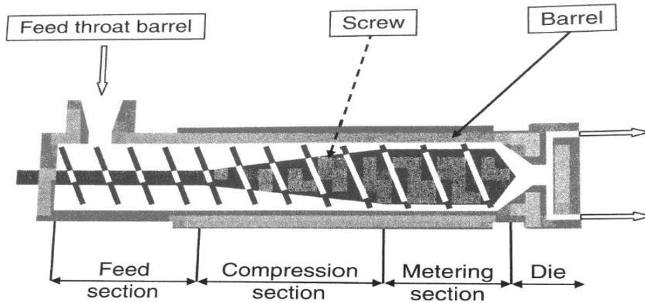
**Figure 2** Monobloc Screw- barrel assembly of the single screw extruder (Bouvier & Campanella, 2014).
