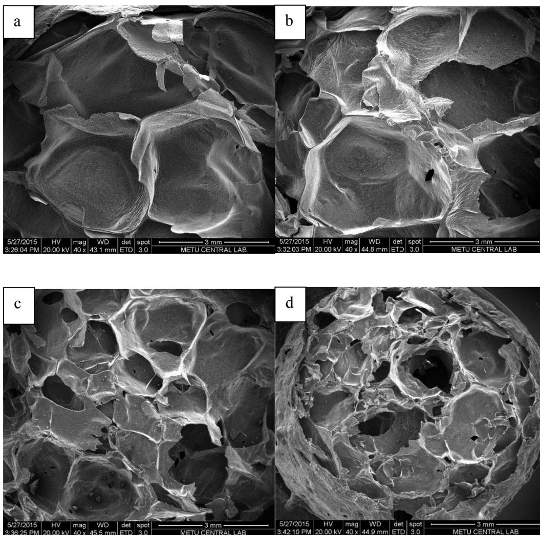
**Figure 4** Scanning electron microscopy images of extrudates with 40X magnification A) Control sample B) 2% microfluidized onion skin added sample C) 6% microfluidized onion skin added sample D) 10% microfluidized onion skin added sample.
