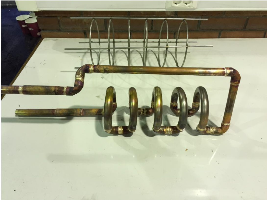
Figure 4.13 HTT of Bed Design 2 after brazing operation
