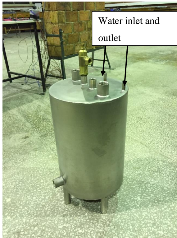
Figure 4.26 Photograph of the cold HTF tank
