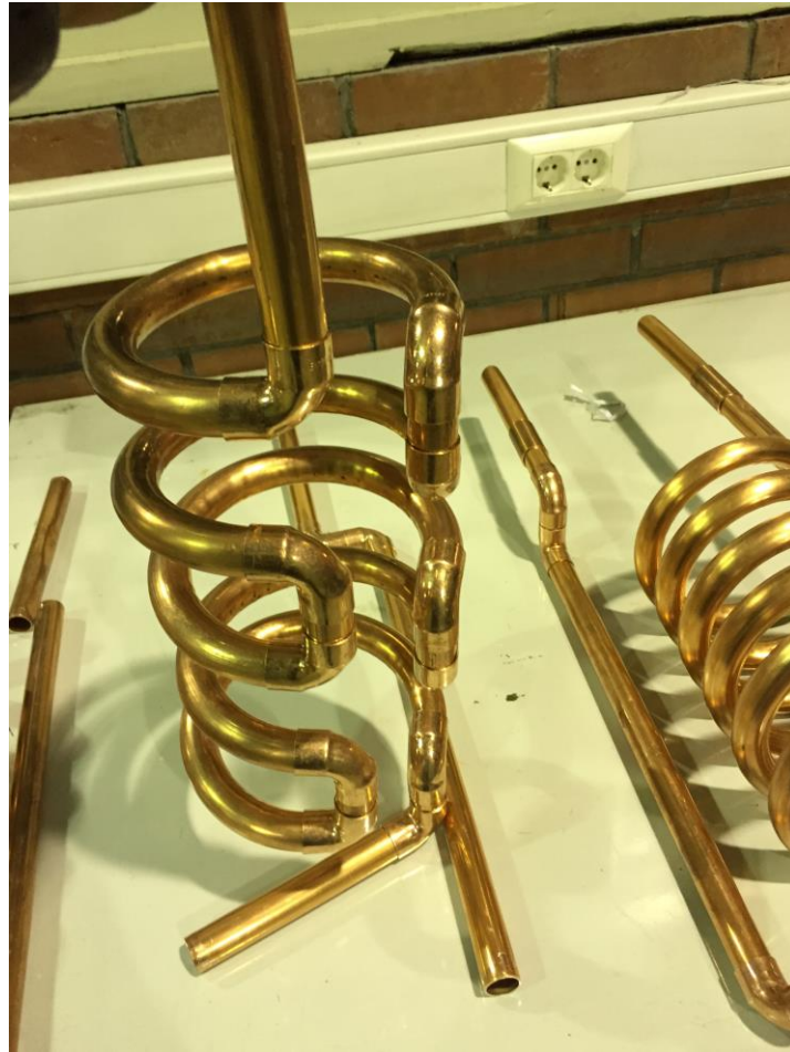
Figure 4.12 The HTT for Bed Design 2 before brazing operation
