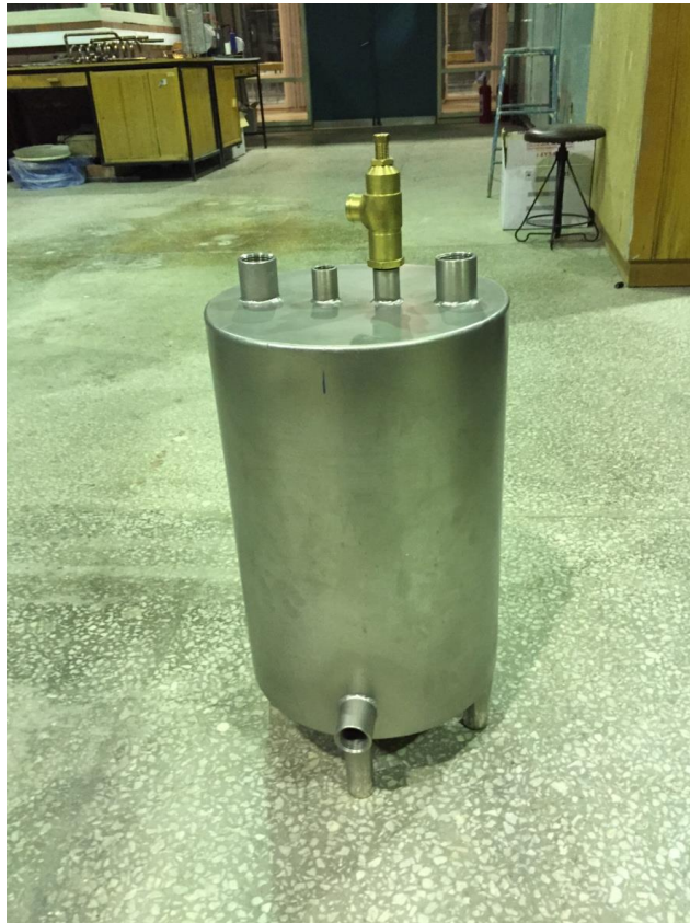
Figure 4.24 Photograph of the hot HTF tank before insulation and installation
