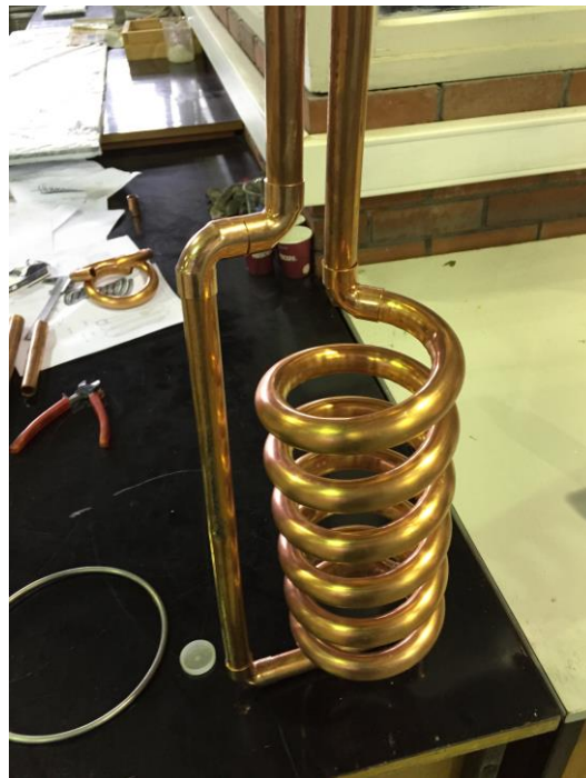
Figure 4.6 The HTT for Bed Design 1 before brazing operation
