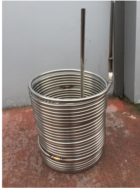
Figure 4.25 Photograph of the cooling coil placed into the cold HTF tank
