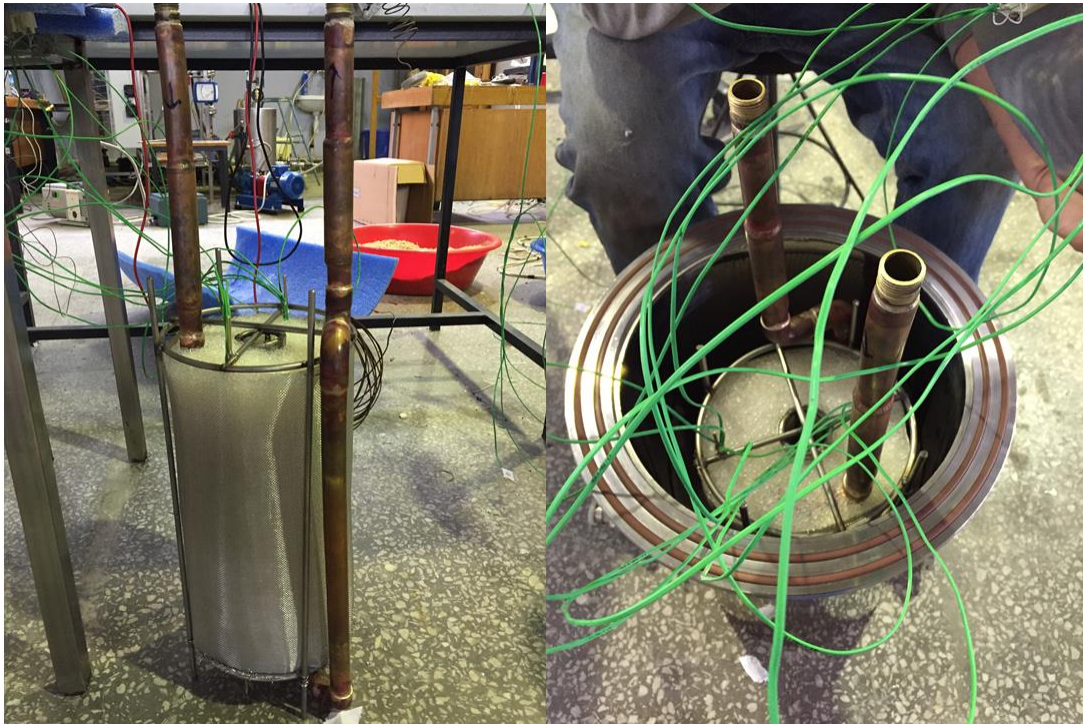
Figure 4.10 The instrumented Bed Design 1 and the placement into vacuum chamber
