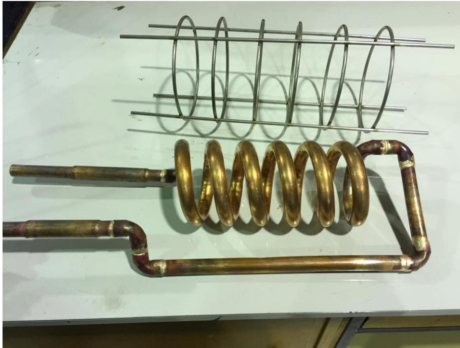
Figure 4.7 HTT of Bed Design 1 after brazing operation
