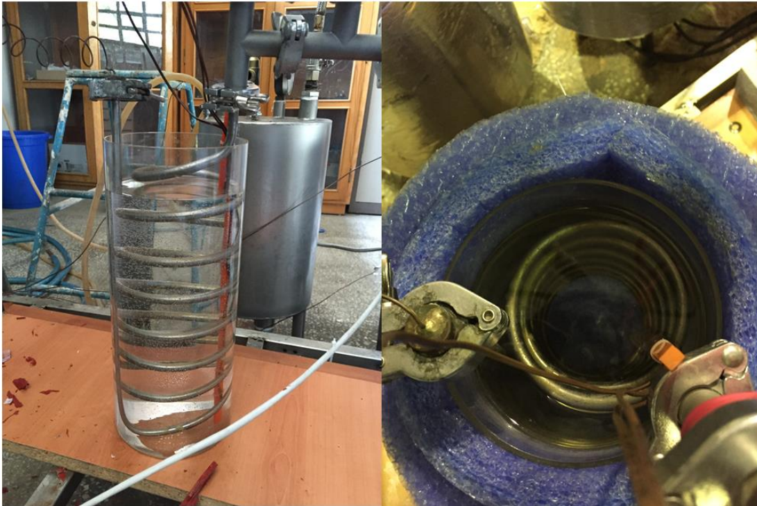
Figure 4.18 The evaporator placed in to the cooling space-without and with insulation
