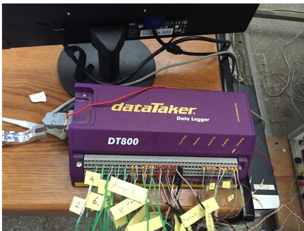
Figure 4.31 The photograph of the data logger (dataTaker DT800) used in the experiments
