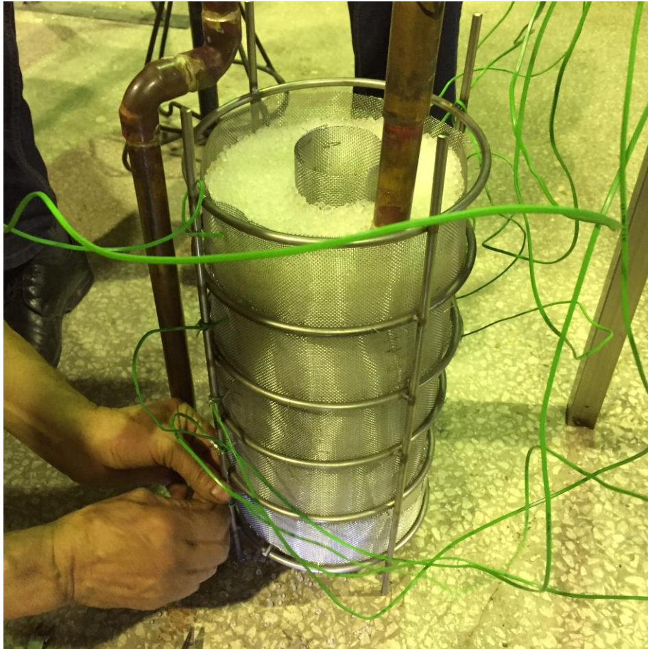
Figure 4.16 The instrumented Bed Design 2 before placement into the vacuum chamber
