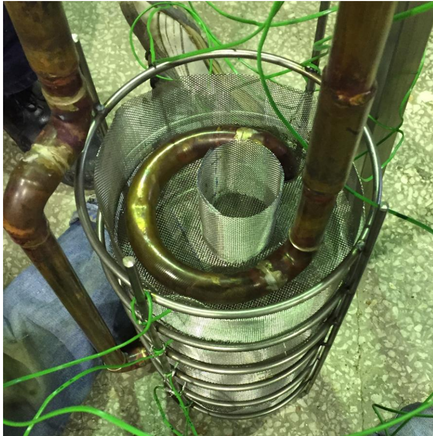
Figure 4.14 HTT of Bed Design 2 metallic net forming the annulus shaped slices around the HTT
