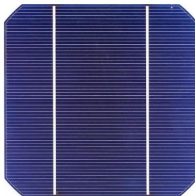
**Figure 19: Front surface metallization design**
