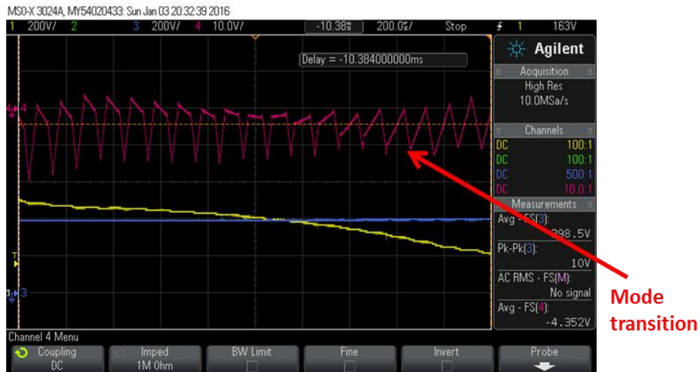
Figure 6-41 Phase A Voltage(yellow), DC link Voltage(blue) and Phase A Inductor Current(magenta) obtained by Test Results
