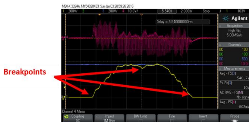
Figure 6-3 Phase A Voltage(yellow), DC link Voltage(blue) and Phase A Inductor Current(magenta) obtained by Test Results
