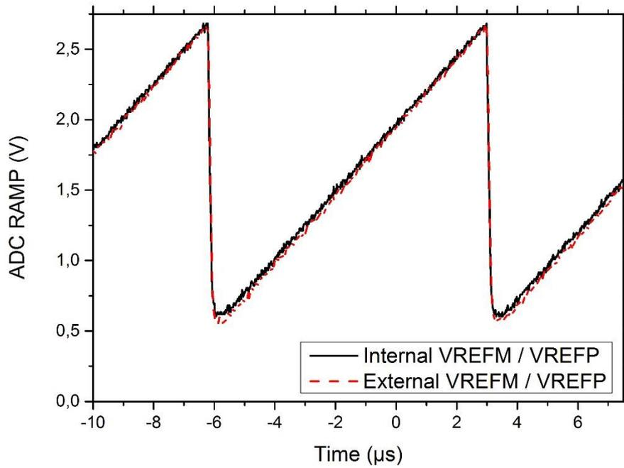
Figure 5.10 Ramp Generator Measured Waveform
