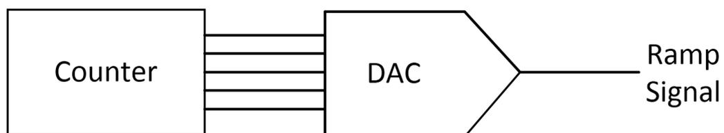
Figure 3.6 DAC Based Ramp Generator
