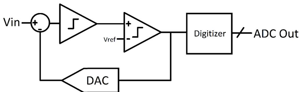
Figure 2.9 Sigma Delta ADC block diagram [23]
