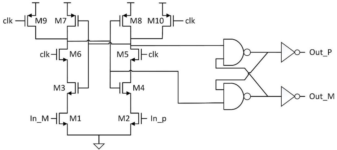
Figure 4.4 Comparator Latch Stage
