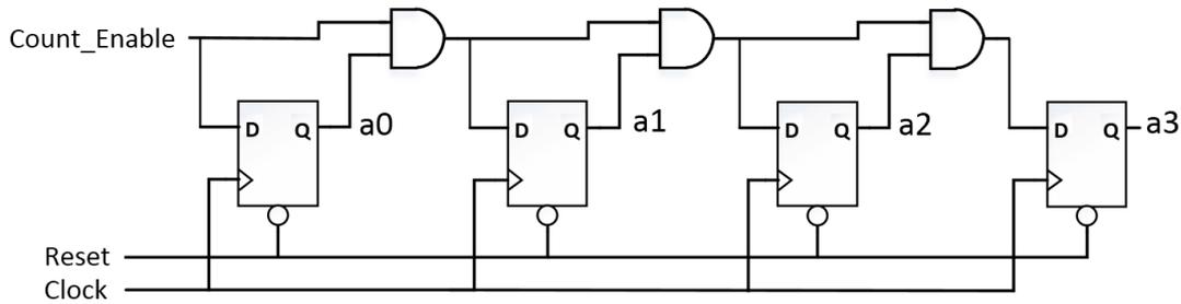
Figure 3.8 4-bit Synchronous Counter example using D Flip Flops
