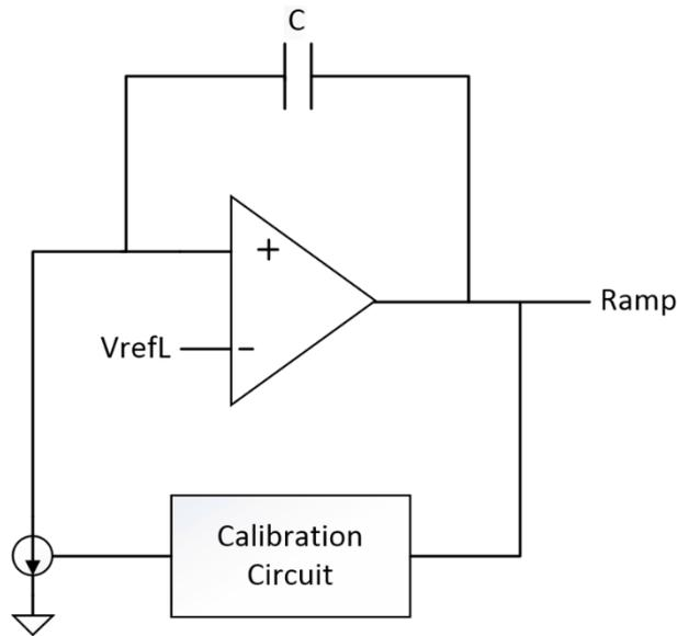
Figure 3.7 Integrator Based Ramp Generator
