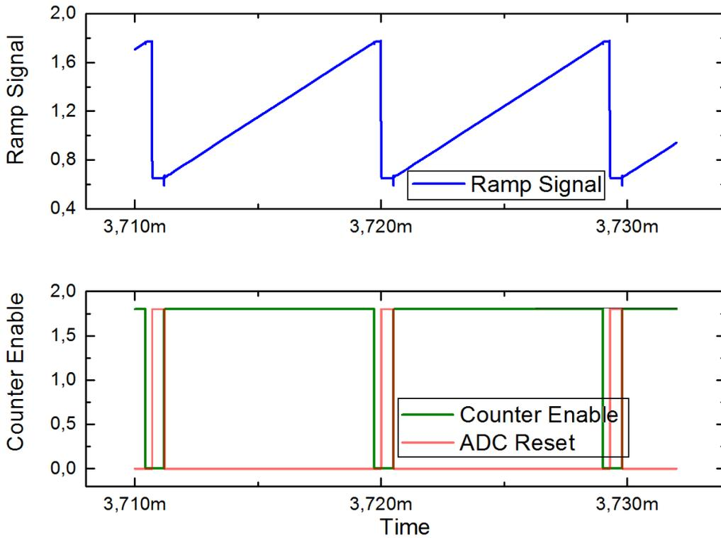
Figure 4.9 Operation of Ramp Generator with respect to reset and enable signal
