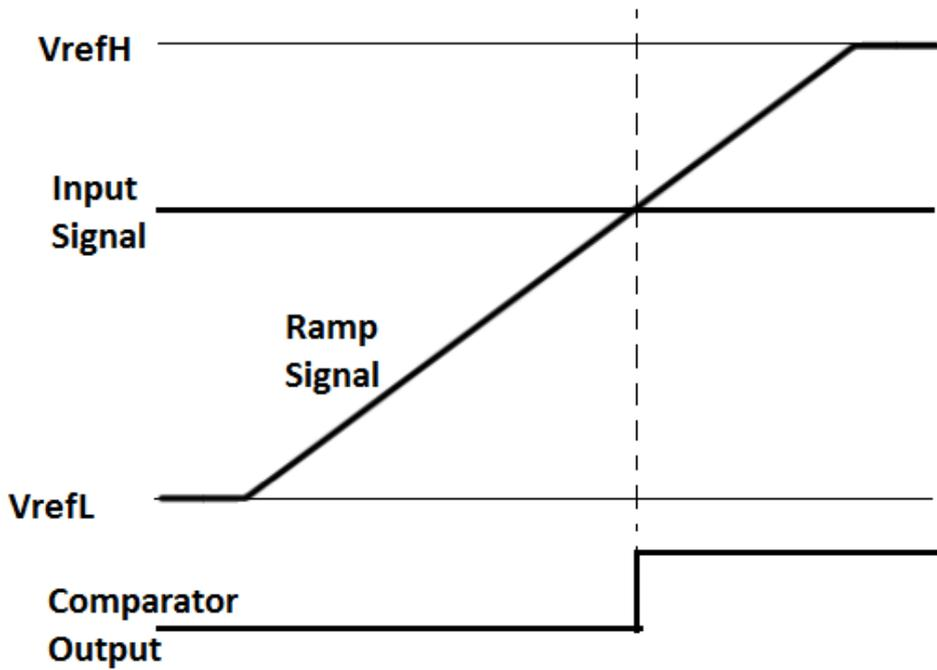
Figure 3.1 Single Slope ADC Operation Principle
