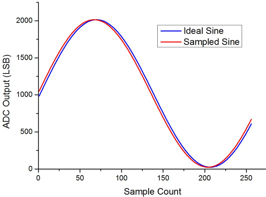
Figure 5.16 Sine wave distortion regarding input stage
