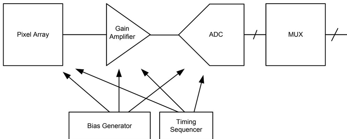
Figure 1.1 ROIC Readout Channel
