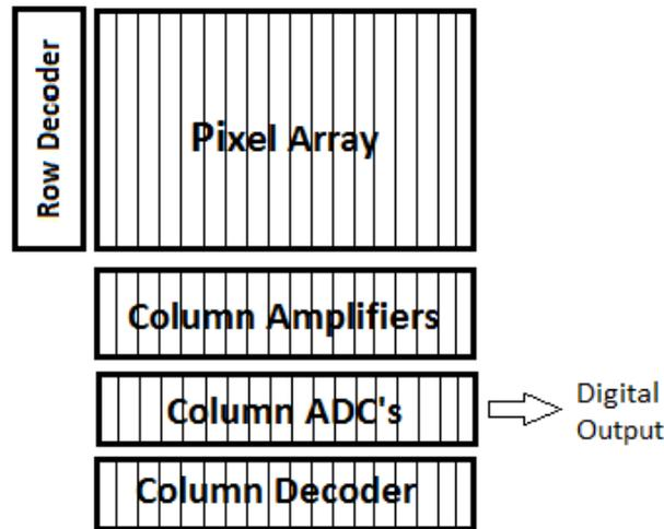
Figure 2.5 Column Level ADC
