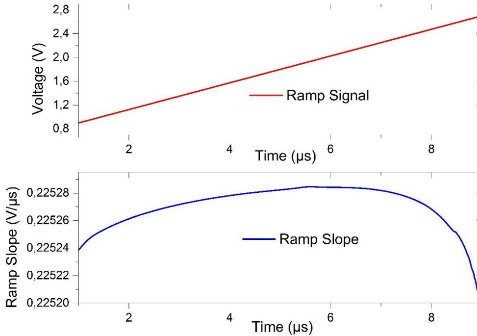
Figure 4.12 Ramp Generator linearity response with the derivative of ramp signal
