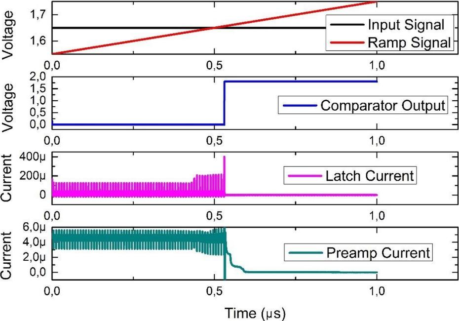
Figure 4.19 Power Down operation of the comparator after crossing of the ramp
