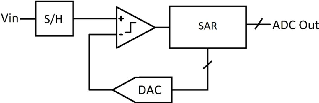
Figure 2.8 SAR ADC Block Diagram [23]
