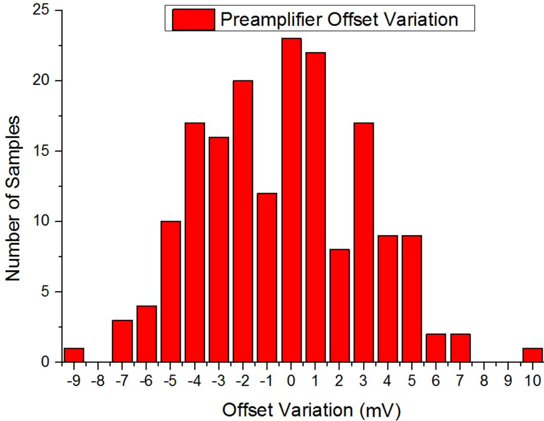
Figure 4.3 Preamplifier Monte-Carlo Analysis Offset Histogram
