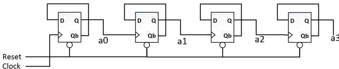
Figure 3.9 4-bit Asynchronous Counter example using D Flip Flops
