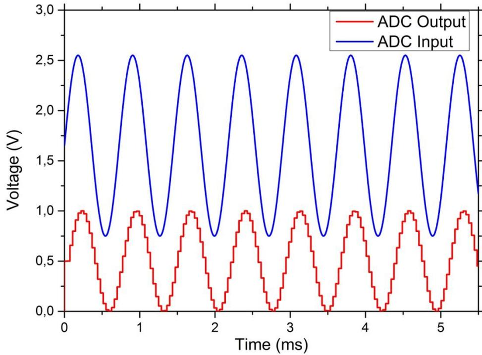
Figure 5.3 ADC output response with respect to applied sine wave
