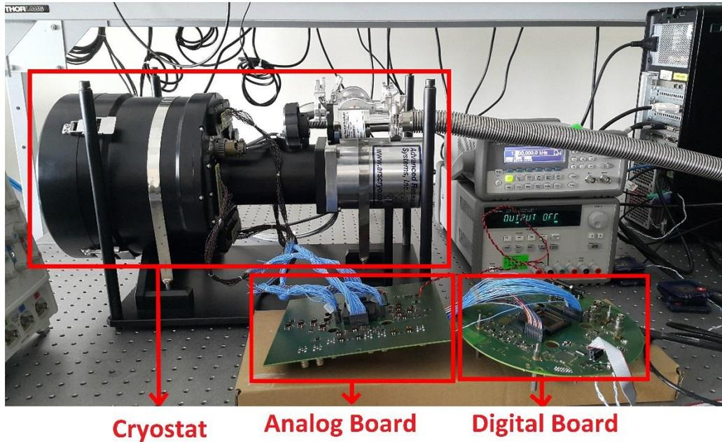
Figure 5.8 Test setup consisting of cryostat, analog and digital interface board
