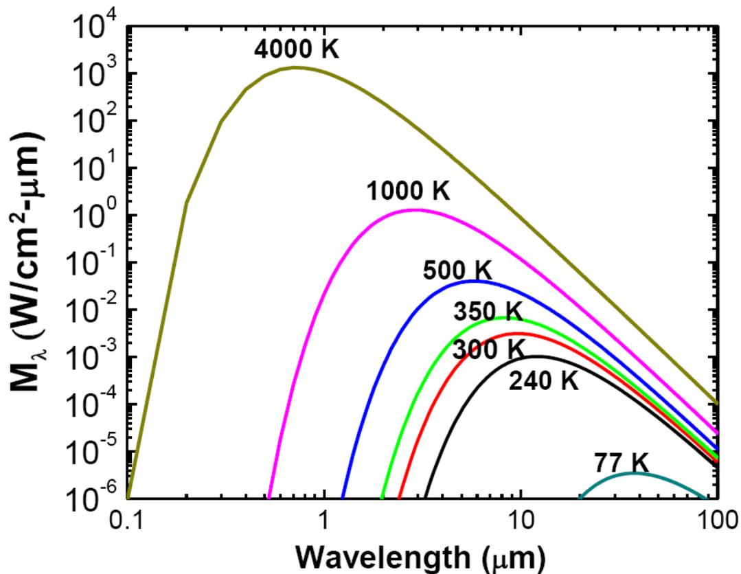
Figure 2.2 Blackbody spectral exitance with respect to wavelength for various temperatures from 77K to 4000K [7]
