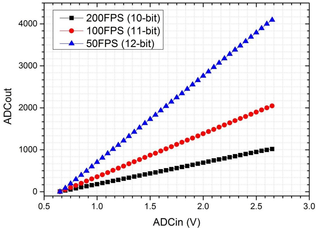
Figure 5.14 ADC Output Response with respect to injected input voltage for various ADC resolution
