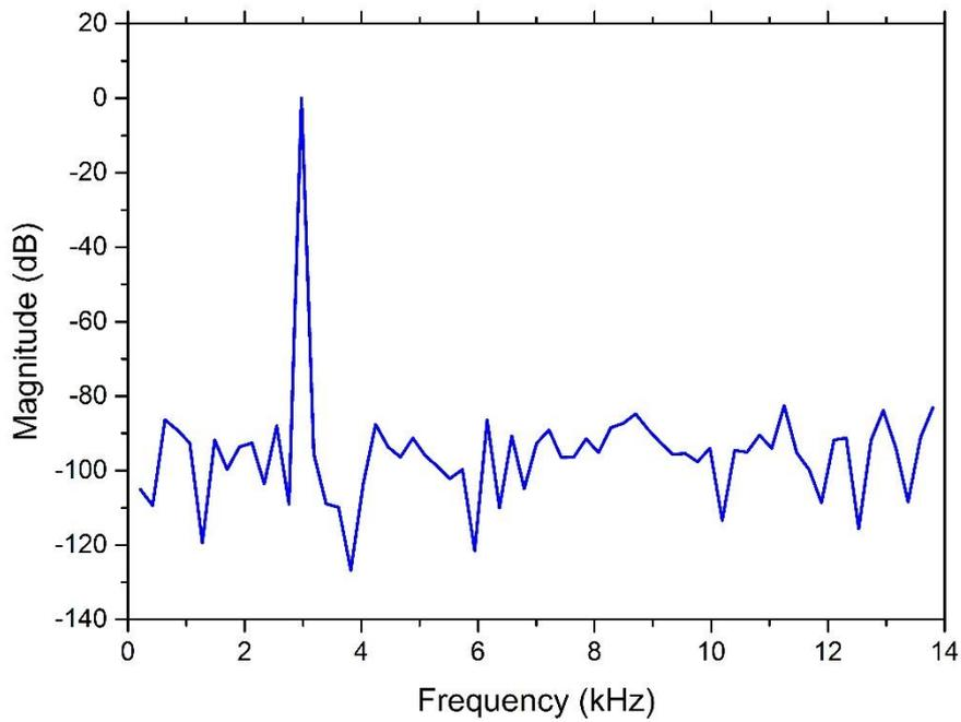
Figure 5.4 128 point FFT Result of the ADC for 77 K temperature
