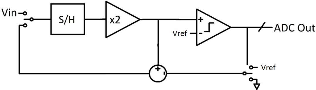
Figure 2.10 Cyclic ADC block diagram [34]
