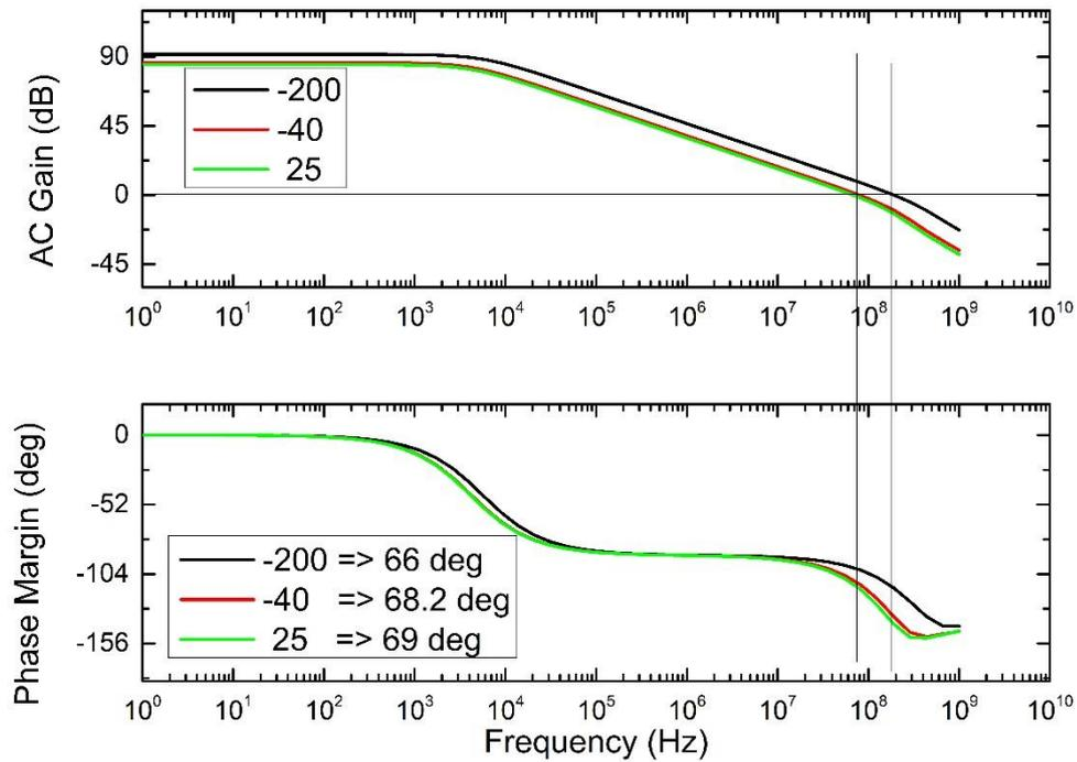
Figure 4.10 AC Frequency Response of Ramp Generator Integrator Amplifier
