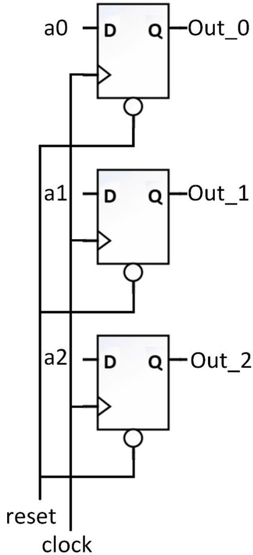
Figure 4.6 3 bit Register Circuit consisted of D-Flip-Flops
