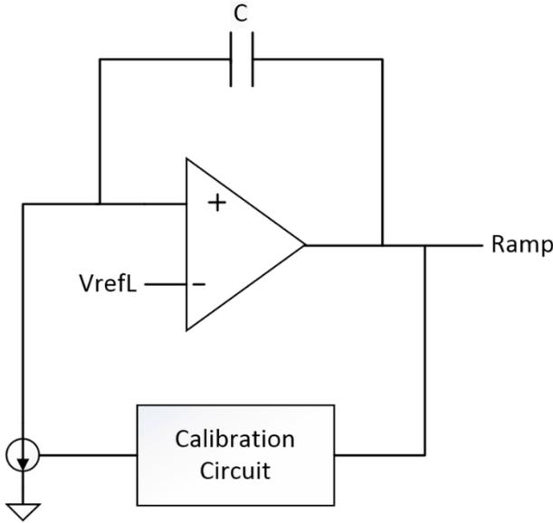
Figure 4.7 Ramp Generator Circuit Topology
