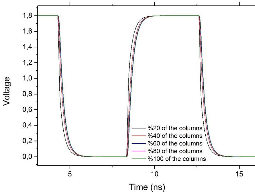
Figure 4.17 Settling behavior of counter outputs as received from various column circuits from near side to far side of the counter circuit
