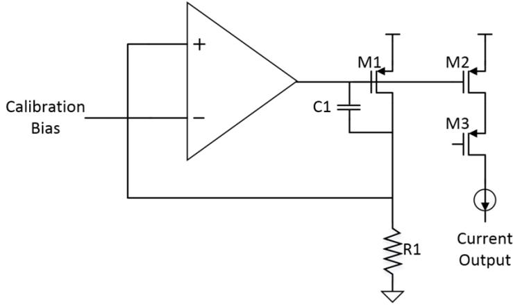
Figure 4.11 Ramp Generator Current Source Circuit
