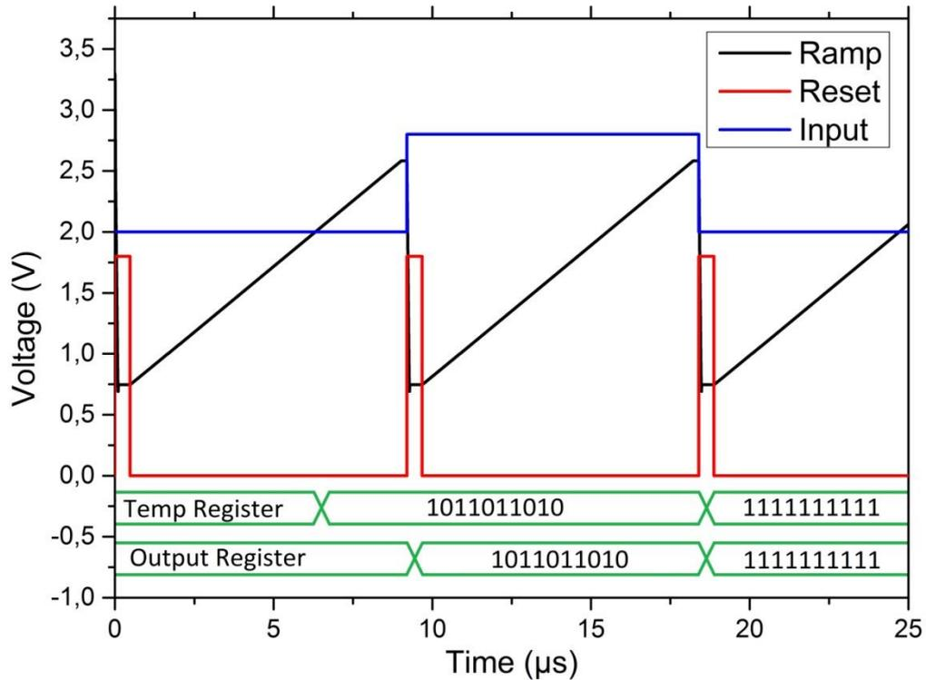
Figure 4.18 Out-of-range simulation and behavior of the memory output
