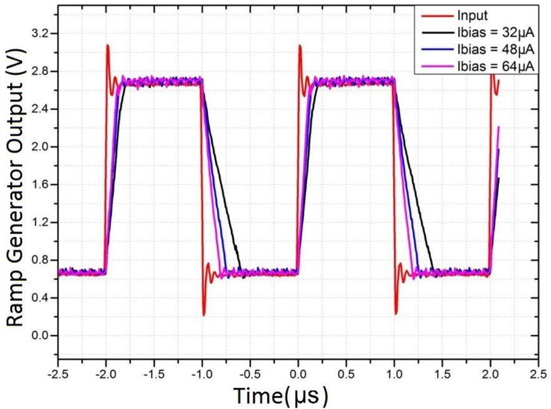
Figure 5.9 Integrator Amplifier's response to the pulse signal for various input bias currents
