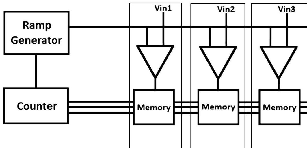
Figure 2.7 Main blocks of a Single Slope ADC [10]
