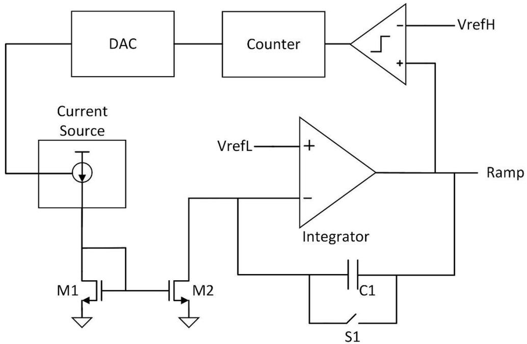
Figure 4.14 Ramp Generator Calibration Feedback
