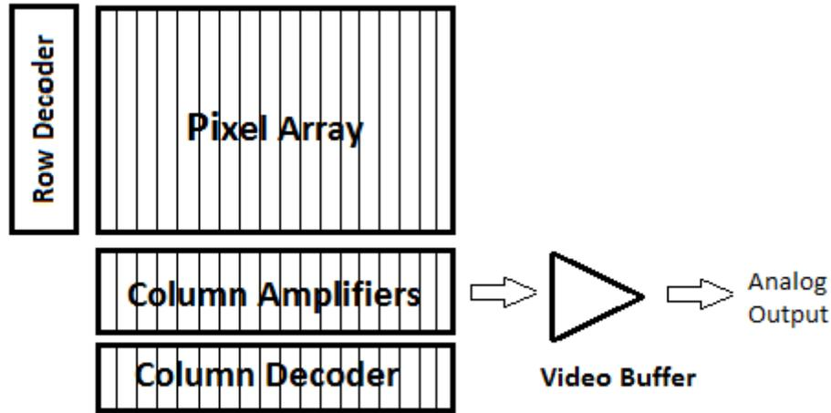
Figure 2.3 Main circuit blocks placement of an Analog Output ROIC
