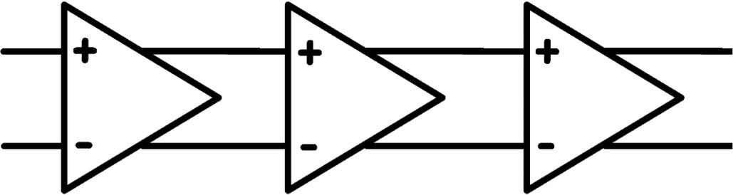
Figure 3.3 Cascaded Gain Stages
