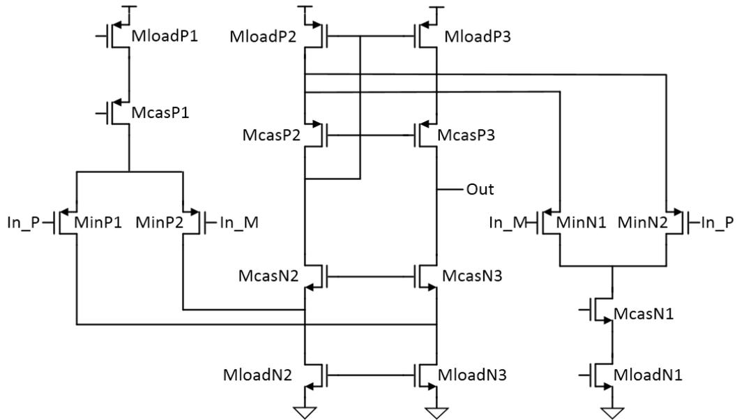
Figure 4.8 Rail-to-Rail Folded Cascode Amplifier
