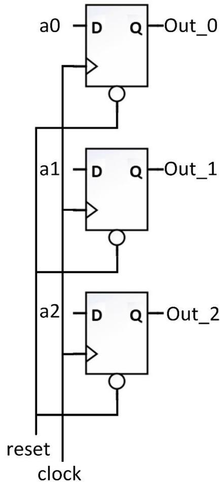
Figure 3.5 D Flip Flop based memory circuit
