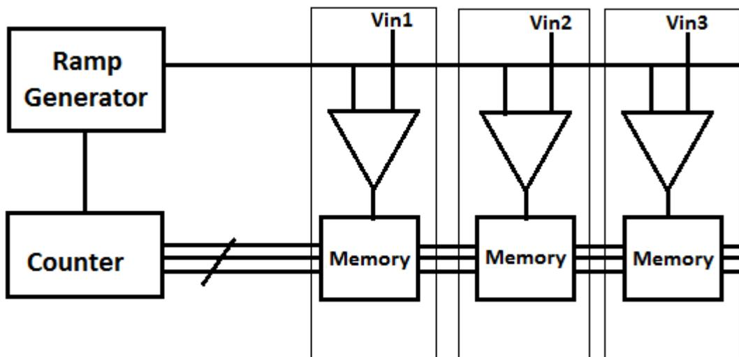
Figure 3.2 Single Slope ADC shared and column circuit blocks placement
