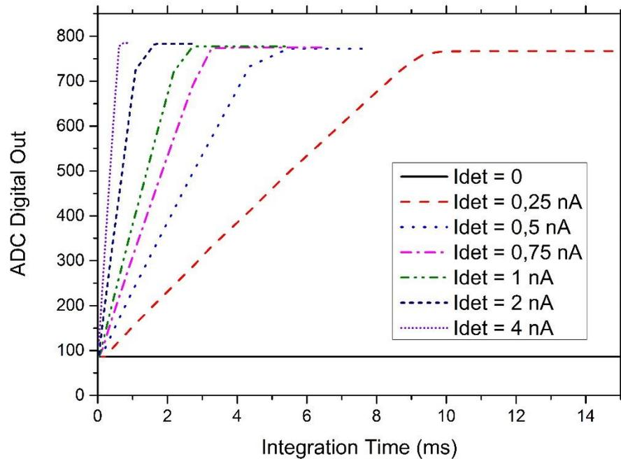
Figure 5.13 ADC Digital Response with respect to integration time for various injected detector currents
