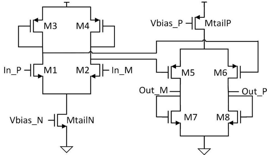
Figure 4.2 Preamplifier Circuit
