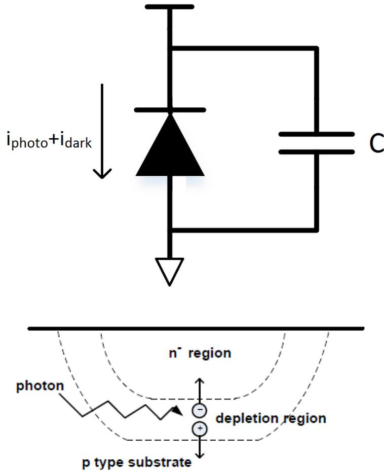
Figure 2.1 Photodiode model and electron hole pair generation mechanism [1]
