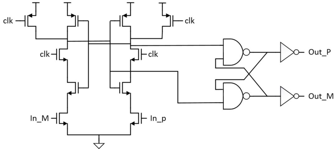
Figure 3.4 Latch Comparator
