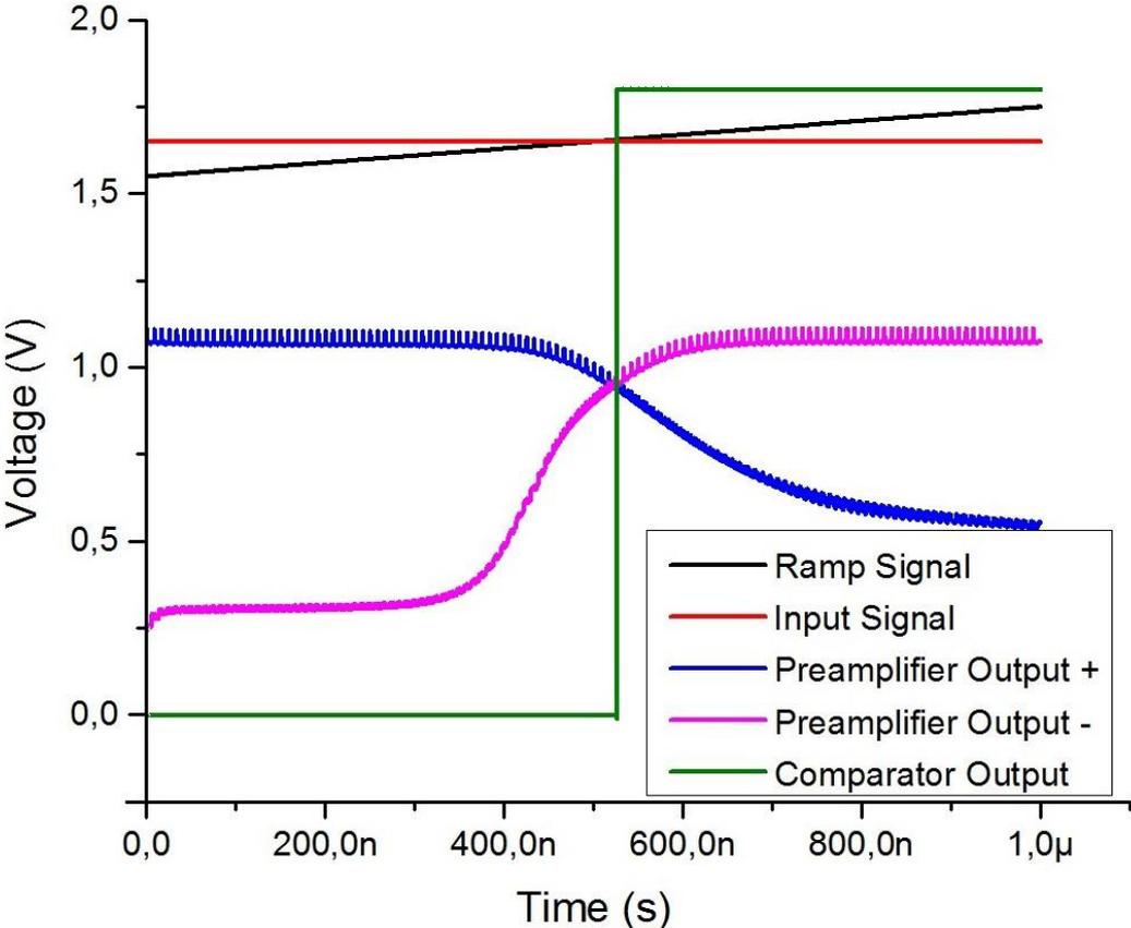
Figure 5.2 Single Slope ADC operation
