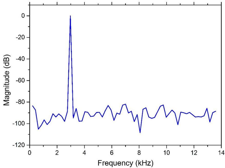
Figure 5.5 128 point FFT Result of the ADC for 300 K temperature
