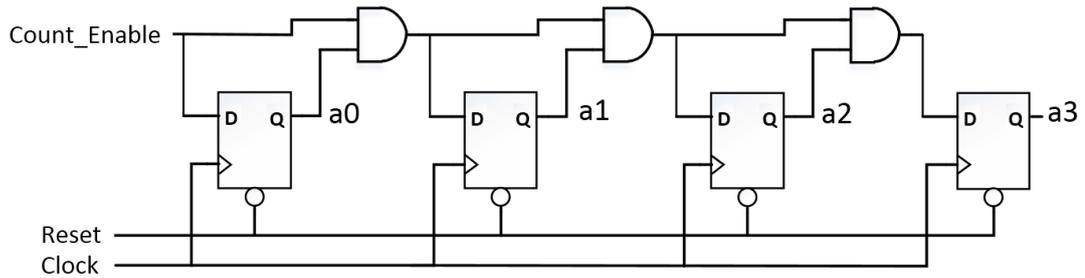
Figure 4.16 4-bit synchronous counter
