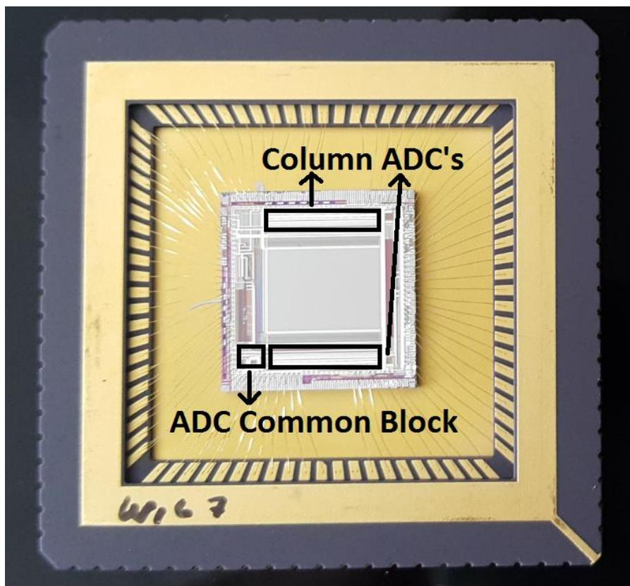
Figure 5.1 Fabricated digital output ROIC
