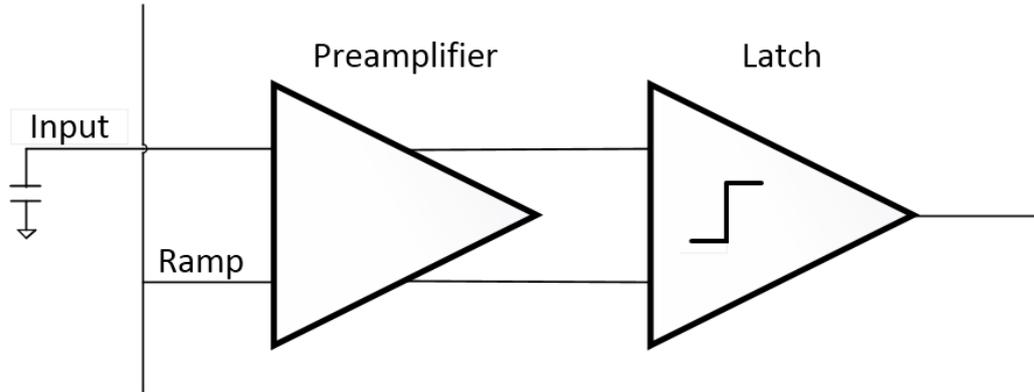
Figure 4.1 Single Slope ADC Comparator Sub-Blocks
