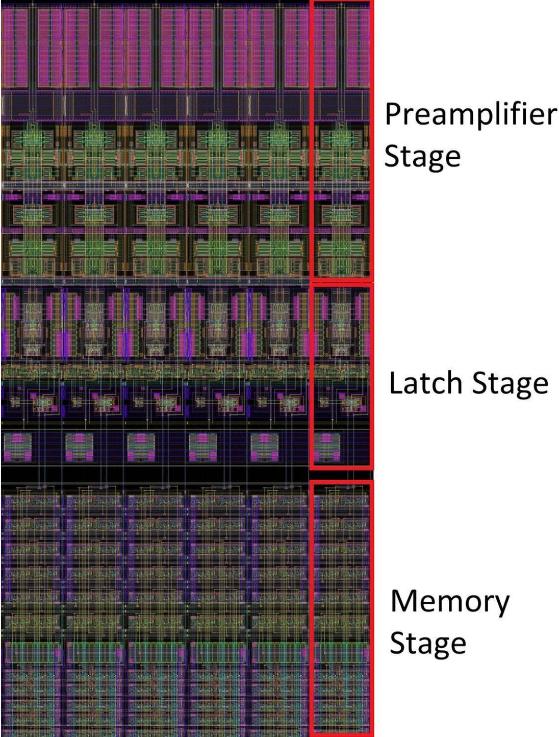
Figure 5.6 Layout of 6 column ADC placed side by side
