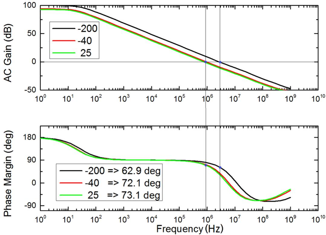
Figure 4.13 AC Frequency Response of the Current Source Feedback Amplifier
