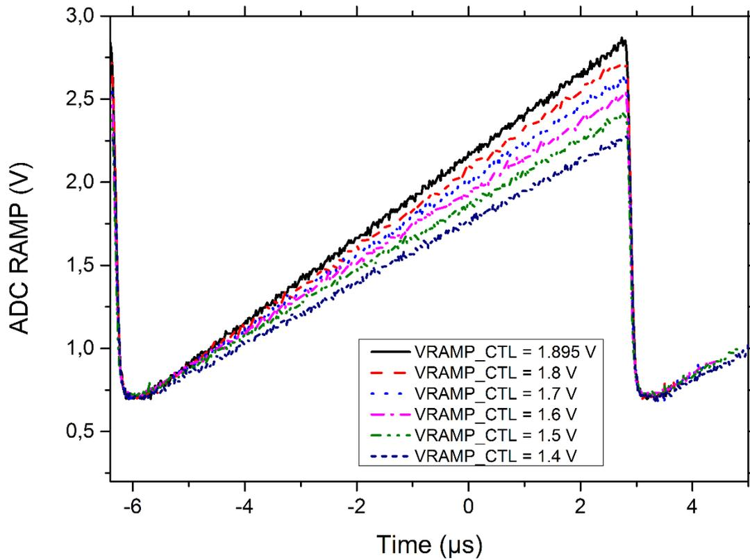
Figure 5.12 Ramp Slope change for various calibration voltages
