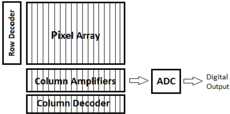
Figure 2.4 Chip Level ADC
