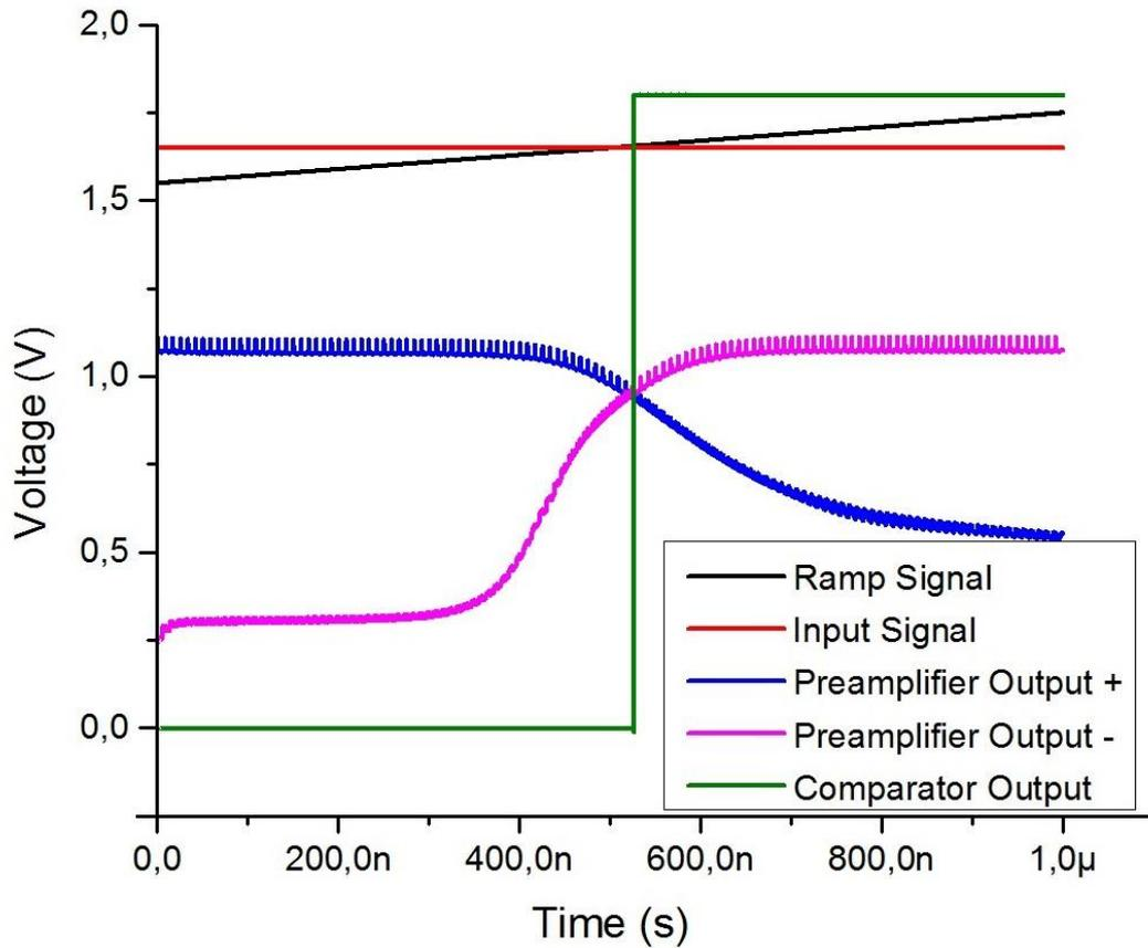
Figure 4.5 Preamplifier and Latch stage output with respect to ramp signal and DC image signal
