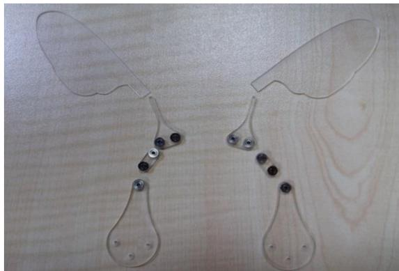
Figure 6.9 Plexi Parts and Bearings used in 4-bar mechanisms and Plexi Calliphora Wing
