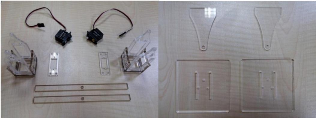
Figure 6.11 Parts used in Rolling Mechanism
