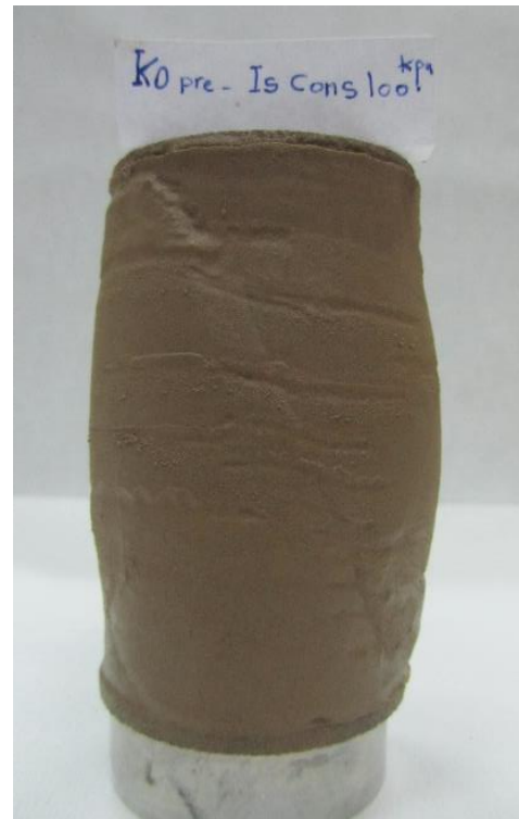
Figures C.7 Failure mode of ORS specimen at saturated condition, \sigma'_3 = 100 kPa.
