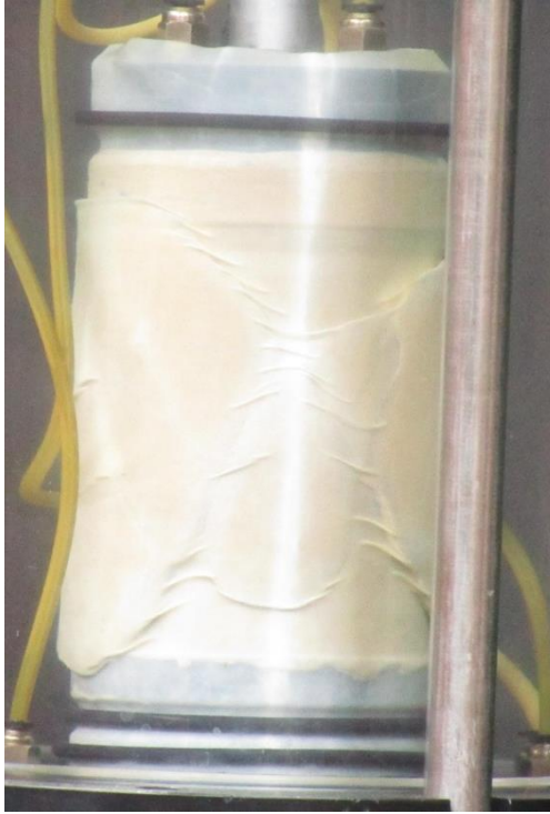
Figures C.27 Failure mode of IRS specimen at unsaturated condition s = 400 kPa, (\sigma_3 - u_a) = 25 kPa
