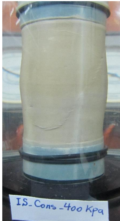
Figures C.4 Failure mode of IRS specimen at saturated condition, \sigma'_3 = 400 kPa.
