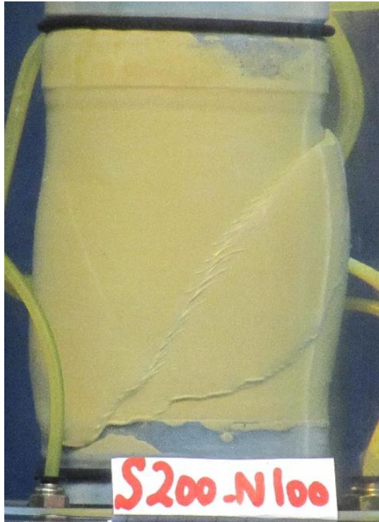
Figures C.25 Failure mode of IRS specimen at unsaturated condition s = 200 kPa, (\sigma_3 - u_a) = 100 kPa
