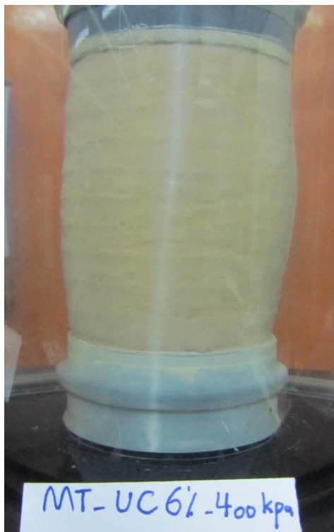
Figures C.16 Failure mode of MT specimen at saturated condition ( w\% = 17.5 , e = 0.72 ), \sigma'_3 = 400 kPa.
