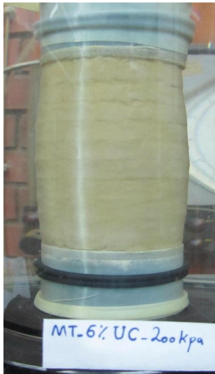
Figures C.19 Failure mode of MT specimen at saturated condition ( w\% = 17.5 , e = 0.82 ), \sigma'_3 = 200 kPa.
