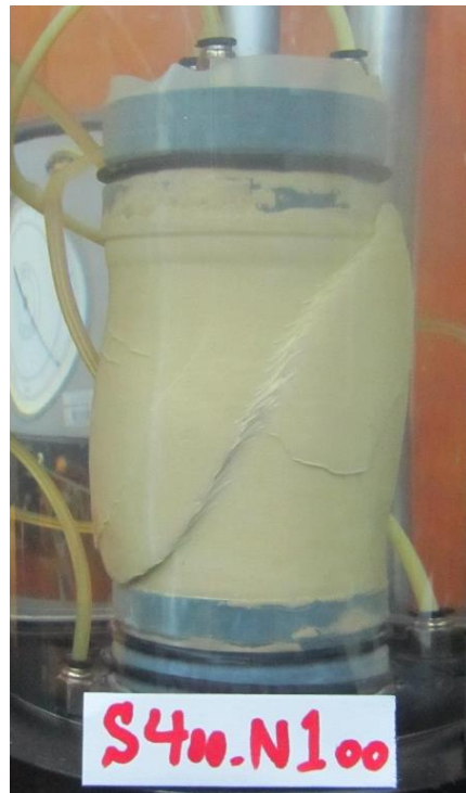
Figures C.28 Failure mode of IRS specimen at unsaturated condition s = 400 kPa, (\sigma_3 - u_a) = 100 kPa
