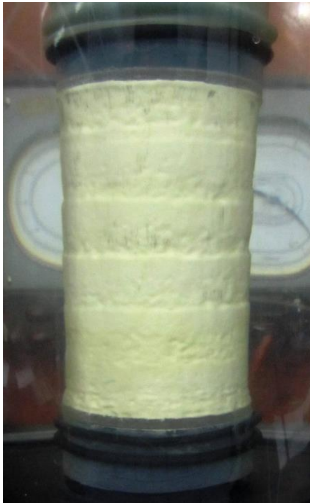
Figure 6.1 Deviations in the cross sectional area after consolidation stage.
