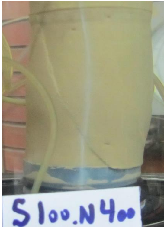
Figures C.23 Failure mode of IRS specimen at unsaturated condition s = 100 kPa, (\sigma_3 - u_a) = 400 kPa
