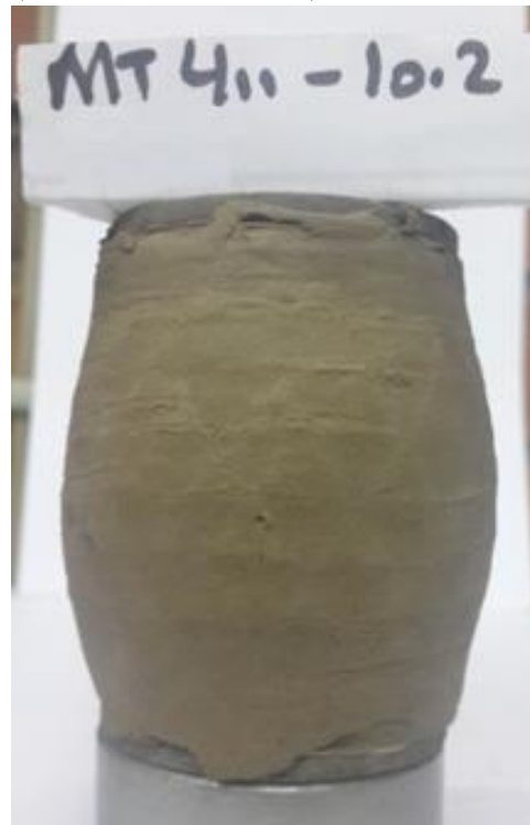
Figures C.11 Failure mode of MT specimen at saturated condition ( w\% = 10.2 , e = 0.72 ), \sigma'_3 = 100 kPa.
