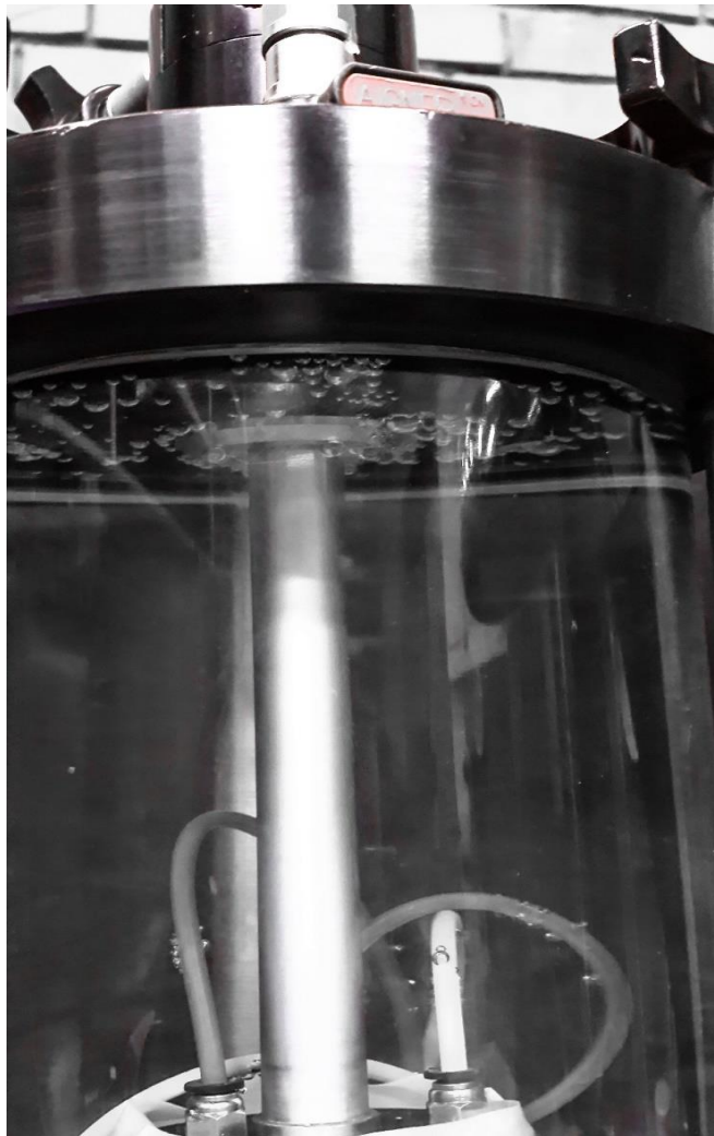
Figure 7.3 Photograph of air bubbles accumulated in triaxial cell after decreasing cell pressure.
