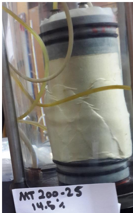
Figures C.40 Failure mode of MT specimen at unsaturated condition, s = 200 kPa, (\sigma_3 - u_a) = 25 kPa
