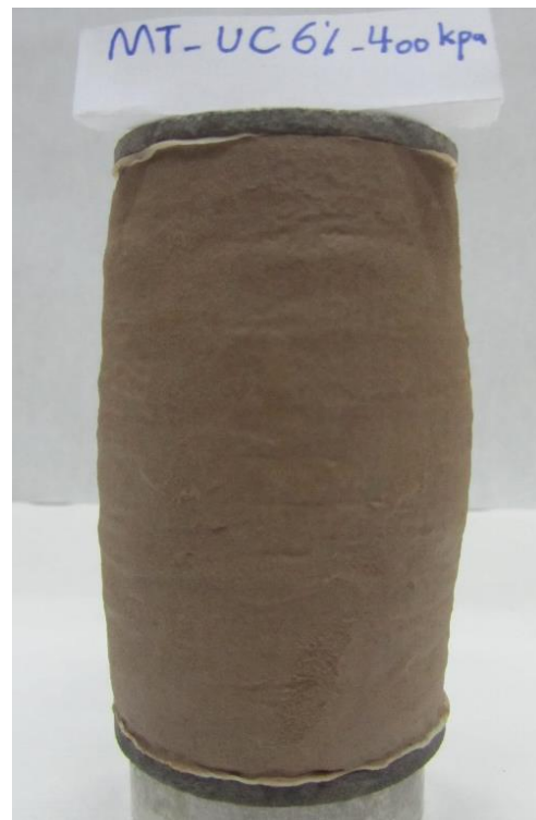
Figures C.16 Failure mode of MT specimen at saturated condition ( w\% = 17.5 , e = 0.72 ), \sigma'_3 = 400 kPa.
