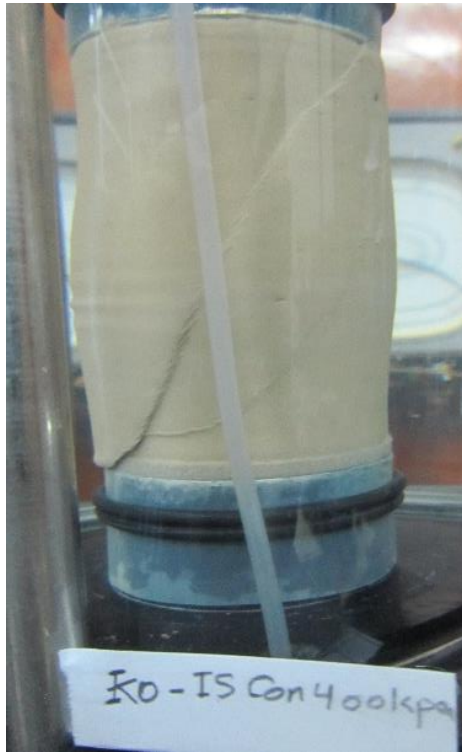
Figures C.9 Failure mode of ORS specimen at saturated condition, \sigma'_3 = 400 kPa.
