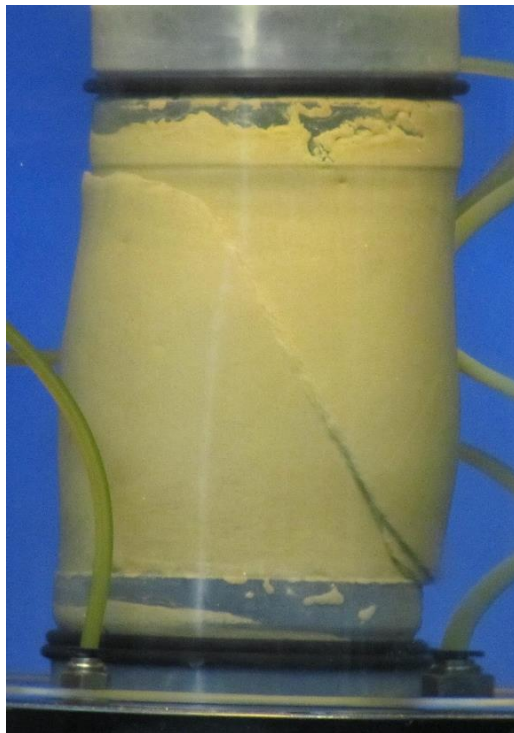
Figures C.26 Failure mode of IRS specimen at unsaturated condition s = 200 kPa, (\sigma_3 - u_a) = 400 kPa
