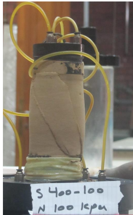
Figures C.33 Failure mode of IRS specimen at unsaturated condition with drying- wetting, s = 400 - 100 kPa, (\sigma_3 - u_a) = 100 kPa
