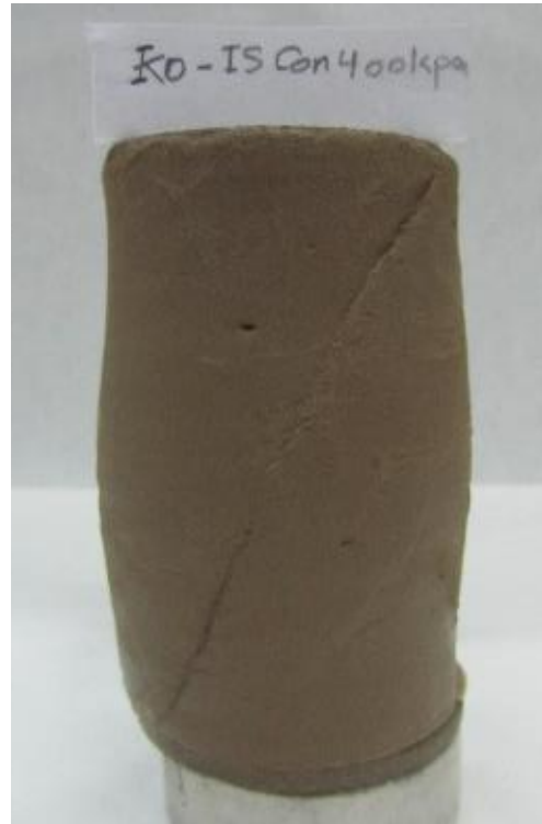
Figures C.9 Failure mode of ORS specimen at saturated condition, \sigma'_3 = 400 kPa.
