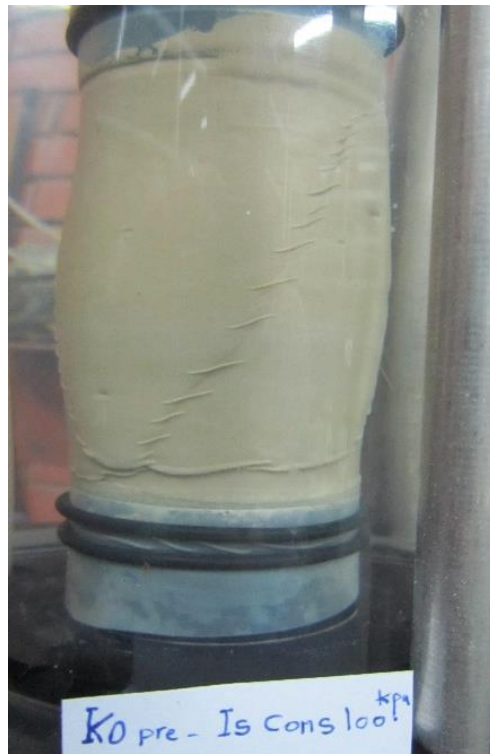
Figures C.7 Failure mode of ORS specimen at saturated condition, \sigma'_3 = 100 kPa.
