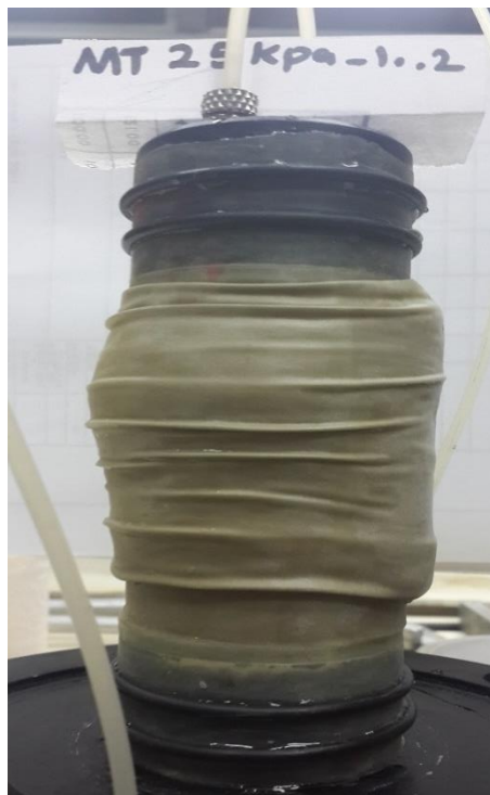
Figures C.10 Failure mode of MT specimen at saturated condition ( w\% = 10.2 , e = 0.72 ), \sigma'_3 = 25 kPa.
