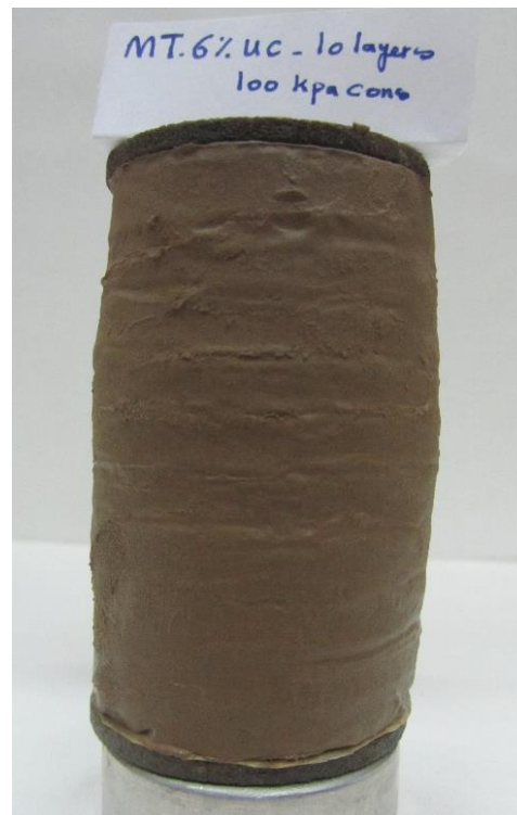
Figures C.18 Failure mode of MT specimen at saturated condition ( w\% = 17.5 , e = 0.82 ), \sigma'_3 = 100 kPa.
