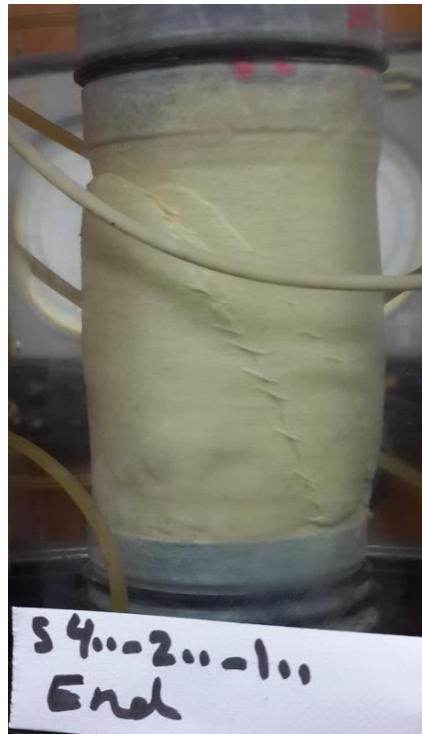
Figures C.36 Failure mode of IRS specimen at unsaturated condition with drying- wetting, s = 400 - 200 kPa, (\sigma_3 - u_a) = 100 kPa
