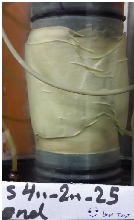
Figures C.35 Failure mode of IRS specimen at unsaturated condition with drying- wetting, s = 400 - 200 kPa, (\sigma_3 - u_a) = 25 kPa
