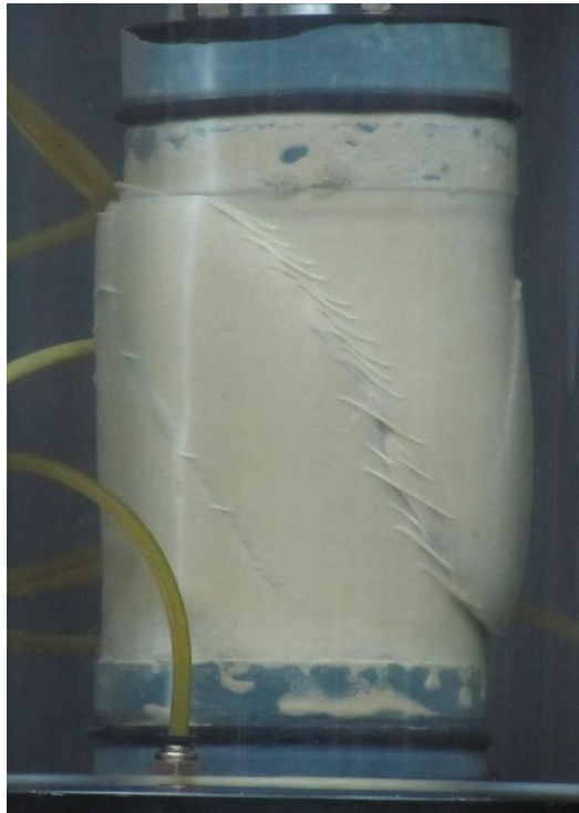
Figures C.32 Failure mode of IRS specimen at unsaturated condition with drying- wetting, s = 400 - 100 kPa, (\sigma_3 - u_a) = 25 kPa
