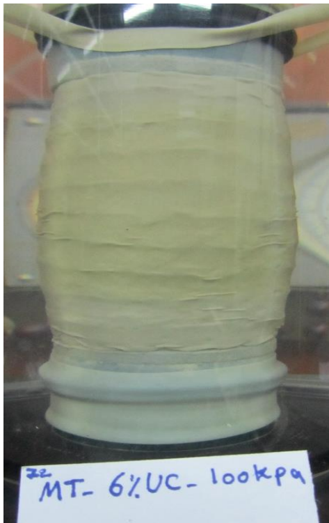
Figures C.14 Failure mode of MT specimen at saturated condition ( w\% = 17.5 , e = 0.72 ), \sigma'_3 = 100 kPa.
