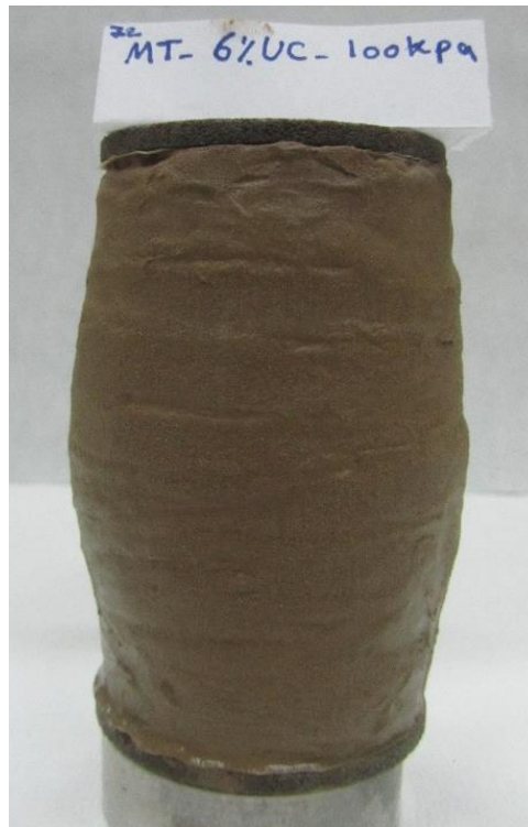
Figures C.14 Failure mode of MT specimen at saturated condition ( w\% = 17.5 , e = 0.72 ), \sigma'_3 = 100 kPa.
