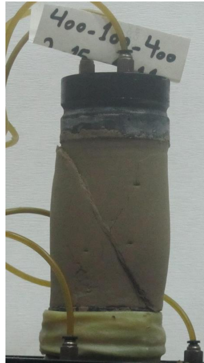
Figures C.34 Failure mode of IRS specimen at unsaturated condition with drying- wetting, s = 400 - 100 kPa, (\sigma_3 - u_a) = 400 kPa
