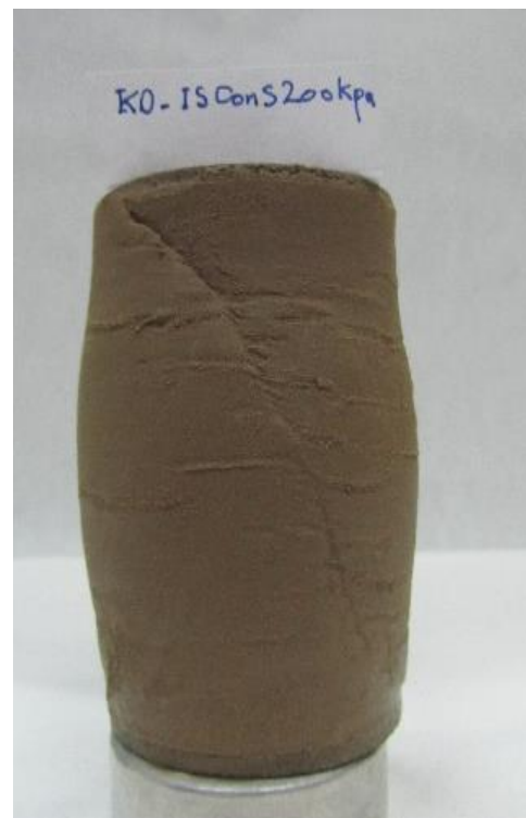
Figures C.8 Failure mode of ORS specimen at saturated condition, \sigma'_3 = 200 kPa.
