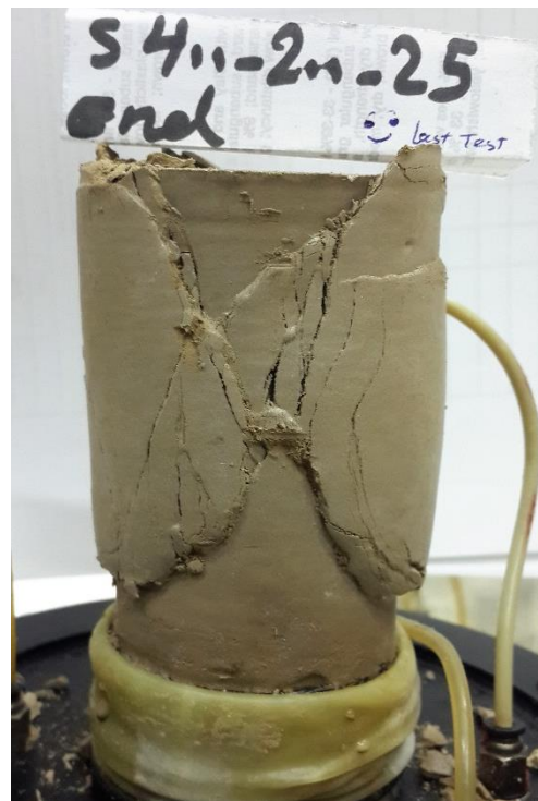
Figures C.35 Failure mode of IRS specimen at unsaturated condition with drying- wetting, s = 400 - 200 kPa, (\sigma_3 - u_a) = 25 kPa
