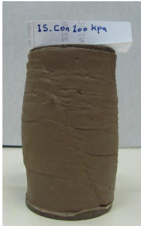
Figures C.2 Failure mode of IRS specimen at saturated condition, \sigma'_3 = 100 kPa.
