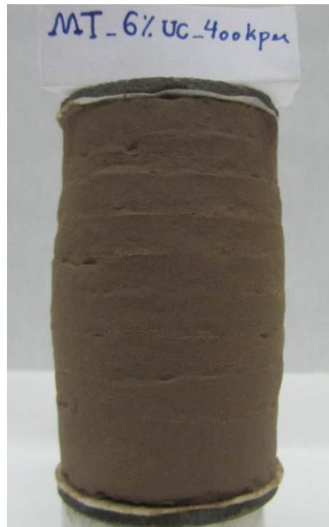
Figures C.20 Failure mode of MT specimen at saturated condition ( w\% = 17.5 , e = 0.82 ), \sigma'_3 = 400 kPa.
