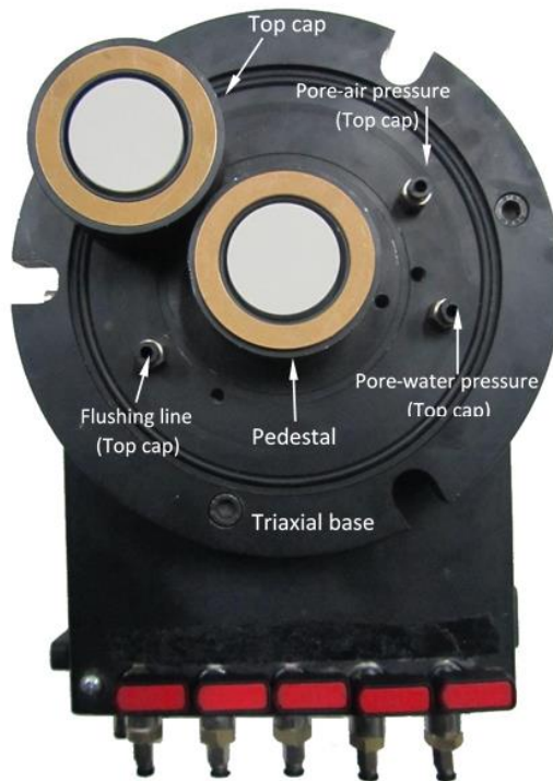
Figure 4.3 New triaxial base with top-cap and pedestal.
