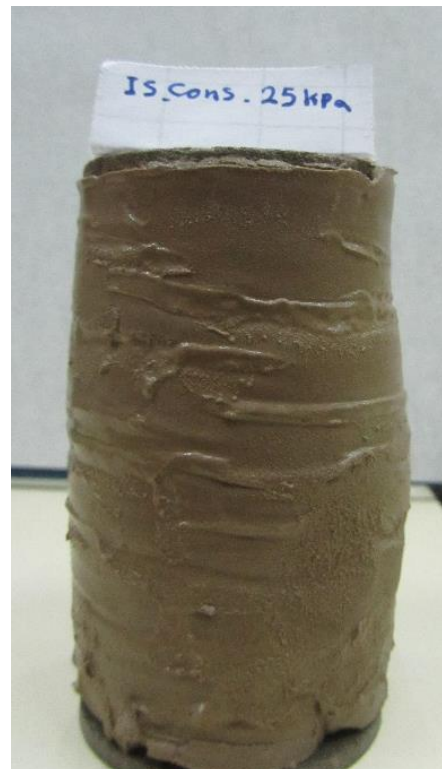
Figures C.1 Failure mode of IRS specimen at saturated condition, \sigma'_3 = 25 kPa.
