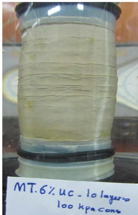
Figures C.18 Failure mode of MT specimen at saturated condition ( w\% = 17.5 , e = 0.82 ), \sigma'_3 = 100 kPa.
