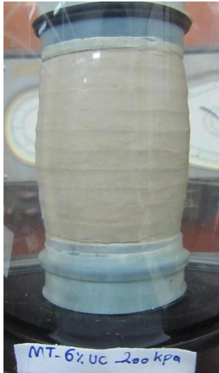
Figures C.15 Failure mode of MT specimen at saturated condition ( w\% = 17.5 , e = 0.72 ), \sigma'_3 = 200 kPa.
