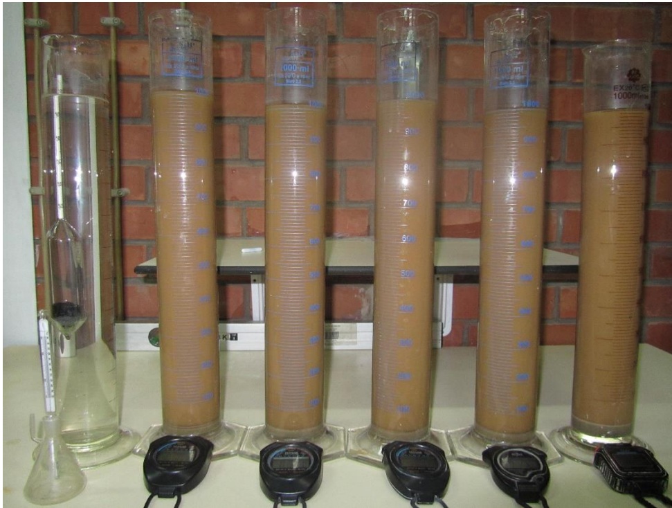
Figure 6.3 Hydrometer test on five divided horizontal slices.
