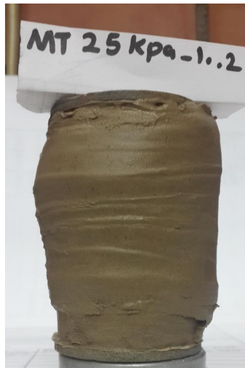
Figures C.10 Failure mode of MT specimen at saturated condition ( w\% = 10.2 , e = 0.72 ), \sigma'_3 = 25 kPa.
