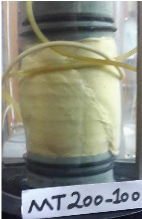
Figures C.41 Failure mode of MT specimen at unsaturated condition, s = 200 kPa, (\sigma_3 - u_a) = 100 kPa
