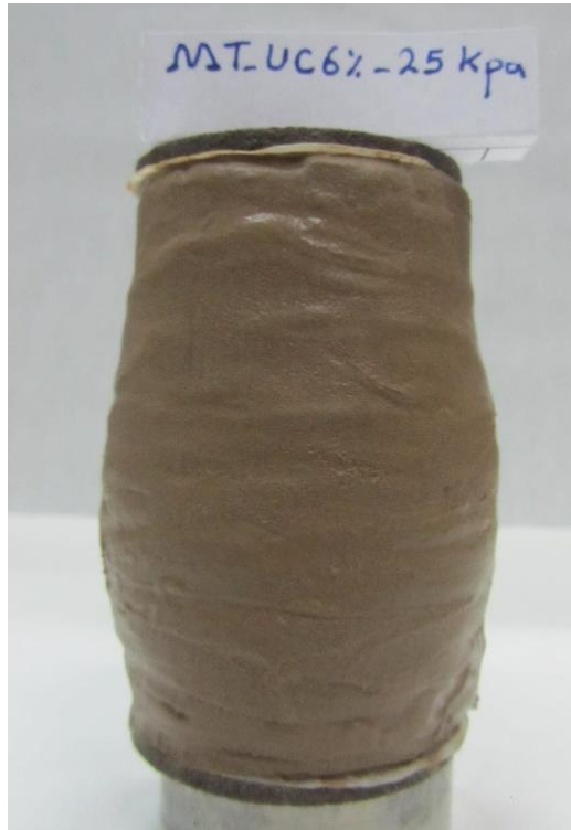
Figures C.13 Failure mode of MT specimen at saturated condition ( w\% = 17.5 , e = 0.72 ), \sigma'_3 = 25 kPa.
