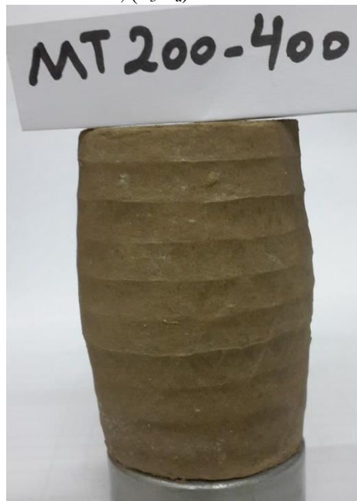
Figures C.42 Failure mode of MT specimen at unsaturated condition, s = 200 kPa, (\sigma_3 - u_a) = 400 kPa
