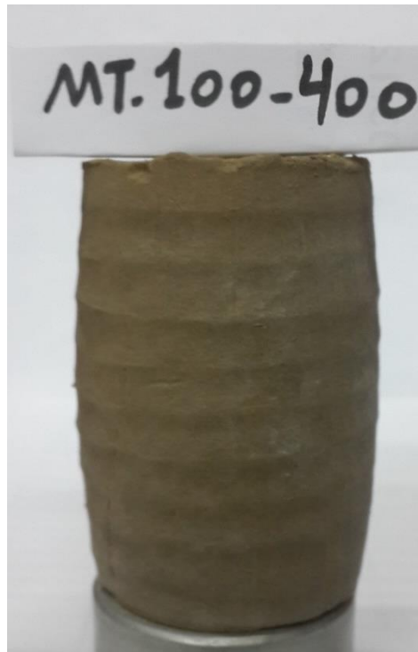
Figures C.39 Failure mode of MT specimen at unsaturated condition, s = 100 kPa, (\sigma_3 - u_a) = 400 kPa
