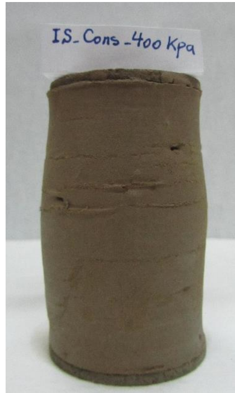
Figures C.4 Failure mode of IRS specimen at saturated condition, \sigma'_3 = 400 kPa.
