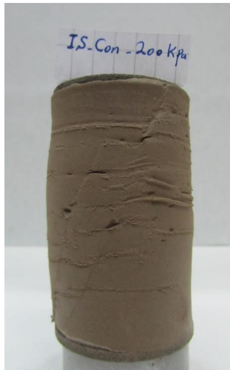
Figures C.3 Failure mode of IRS specimen at saturated condition, \sigma'_3 = 200 kPa.
