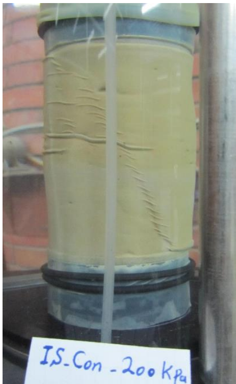
Figures C.3 Failure mode of IRS specimen at saturated condition, \sigma'_3 = 200 kPa.
