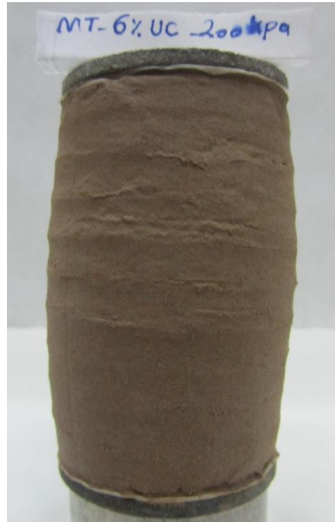
Figures C.15 Failure mode of MT specimen at saturated condition ( w\% = 17.5 , e = 0.72 ), \sigma'_3 = 200 kPa.
