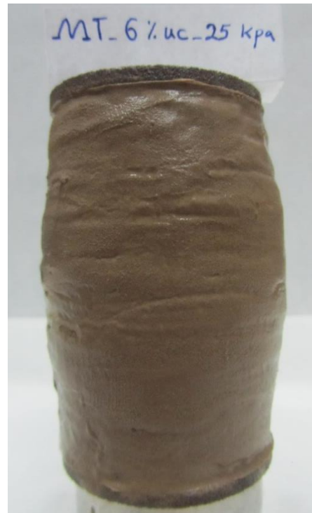
Figures C.17 Failure mode of MT specimen at saturated condition ( w\% = 17.5 , e = 0.82 ), \sigma'_3 = 25 kPa.
