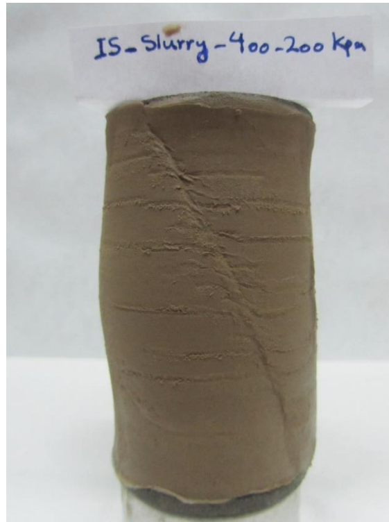
Figures C.5 Failure mode of IRS specimen at saturated condition with loading-unloading, \sigma'_3 = 400-200 kPa (OCR = 2).
