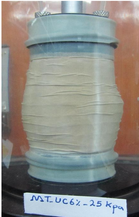
Figures C.13 Failure mode of MT specimen at saturated condition ( w\% = 17.5 , e = 0.72 ), \sigma'_3 = 25 kPa.
