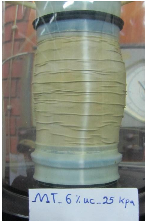
Figures C.17 Failure mode of MT specimen at saturated condition ( w\% = 17.5 , e = 0.82 ), \sigma'_3 = 25 kPa.
