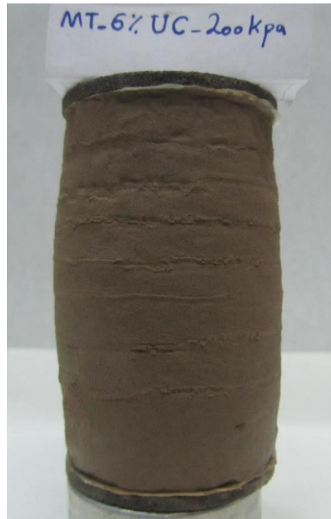
Figures C.19 Failure mode of MT specimen at saturated condition ( w\% = 17.5 , e = 0.82 ), \sigma'_3 = 200 kPa.
