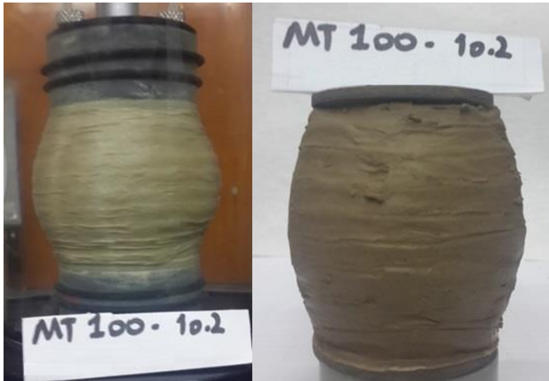
Figures C.11 Failure mode of MT specimen at saturated condition ( w\% = 10.2 , e = 0.72 ), \sigma'_3 = 100 kPa.
