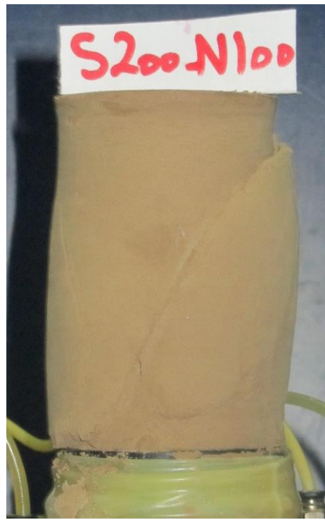
Figures C.25 Failure mode of IRS specimen at unsaturated condition s = 200 kPa, (\sigma_3 - u_a) = 100 kPa
