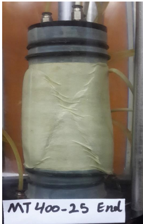
Figures C.43 Failure mode of MT specimen at unsaturated condition, s = 400 kPa, (\sigma_3 - u_a) = 25 kPa
