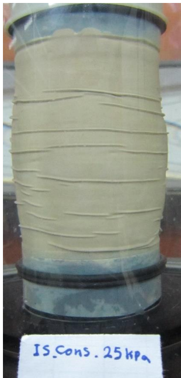
Figures C.1 Failure mode of IRS specimen at saturated condition, \sigma'_3 = 25 kPa.
