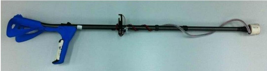
Figure 3.2: ErgoTech model forearm crutch after modifications, which is called as the smart crutch.
