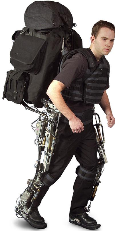
Figure 2.2: BLEEX platform worn on the body (Reproduced from [15]).
