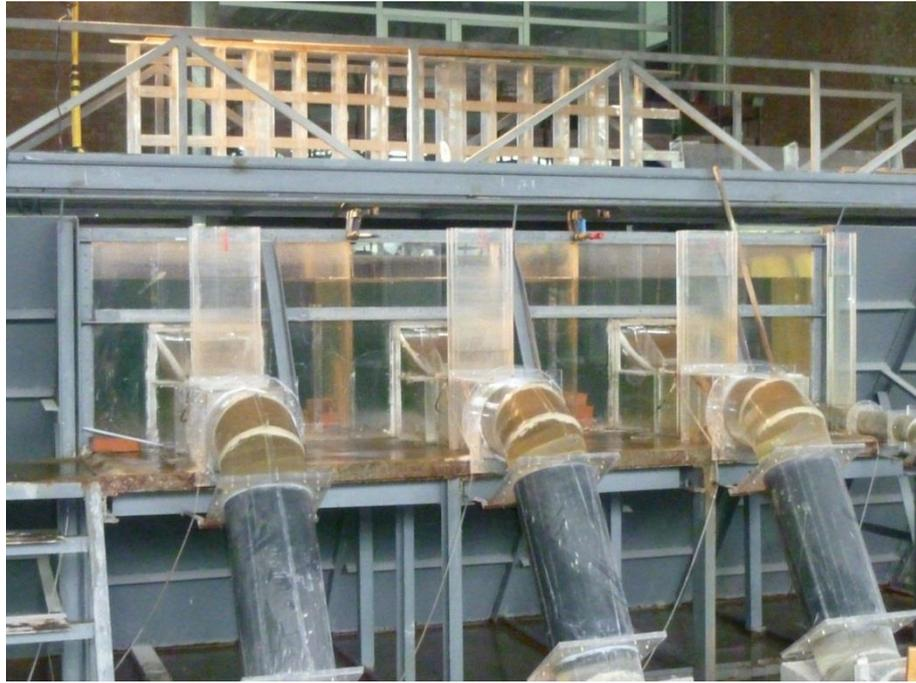
Figure 4.3 Close view of the triple water intake structure from downstream
