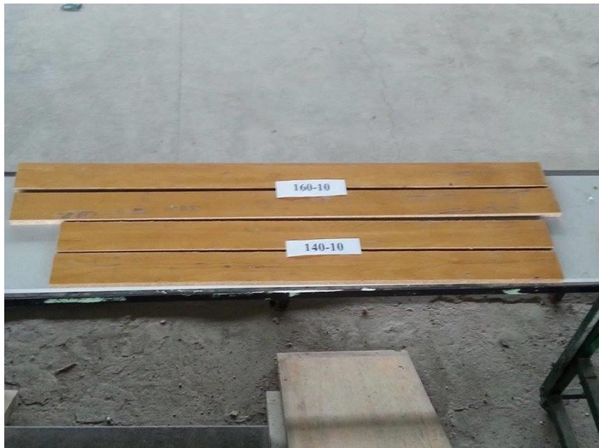
Figure 4.16 Top view of floating rafts which is used at vortex prevention during experiments (dimensions are in cm)
