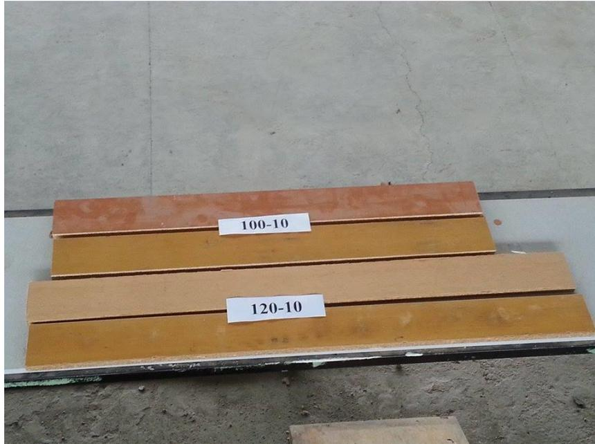
Figure 4.15 Top view of floating rafts which is used at vortex prevention during experiments (dimensions are in cm)
