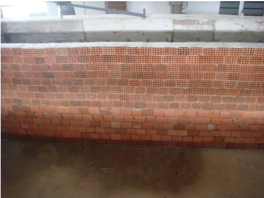
Figure 4.2 Hollow bricks and coarse screens which are located at the entrance of the model
