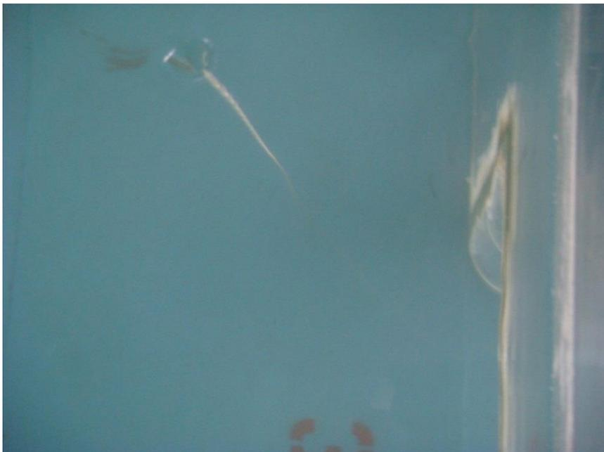
Figure 4.14 Vortex formation in front of triple water intake structure ( $Q=96.20$
