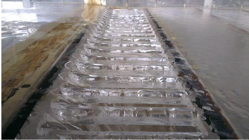
Figure 2.3 Flow passing through a grate inlet
