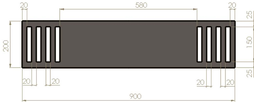
Figure 3.15 Grated bars on both sides with full middle part (All dimensions are in mm)
