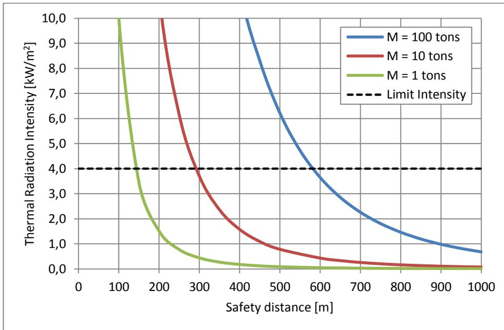
Figure 37 Variation Safety Distance with Propellant Weight (Thermal Effects)
