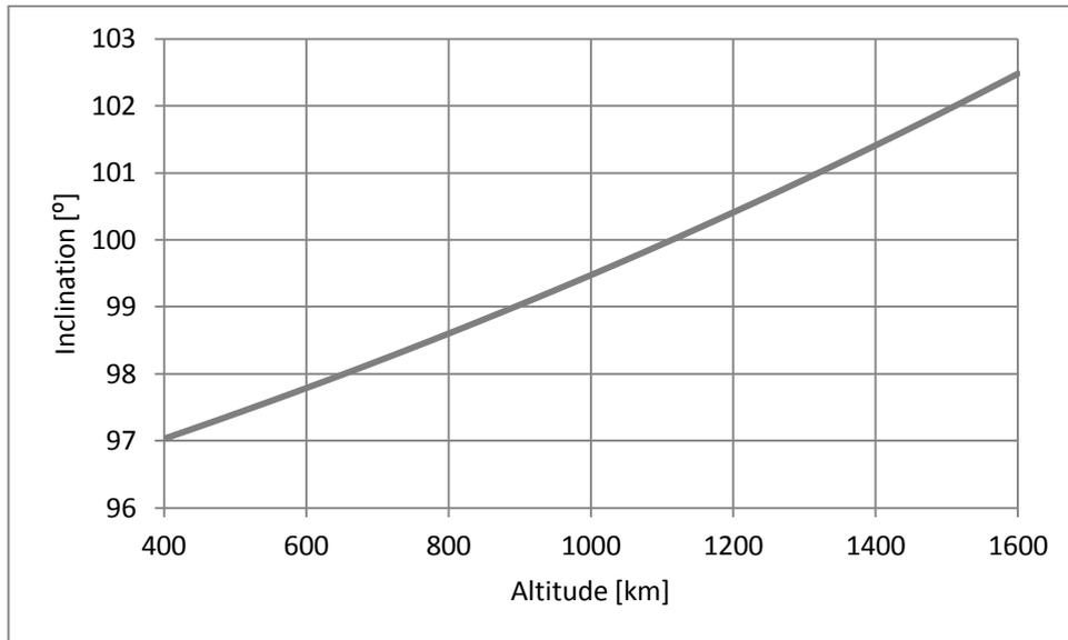
Figure 17 Variation of Inclination for SSO
