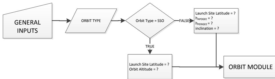
Figure 64 Orbital Parameters for the Operation of Orbit Module
