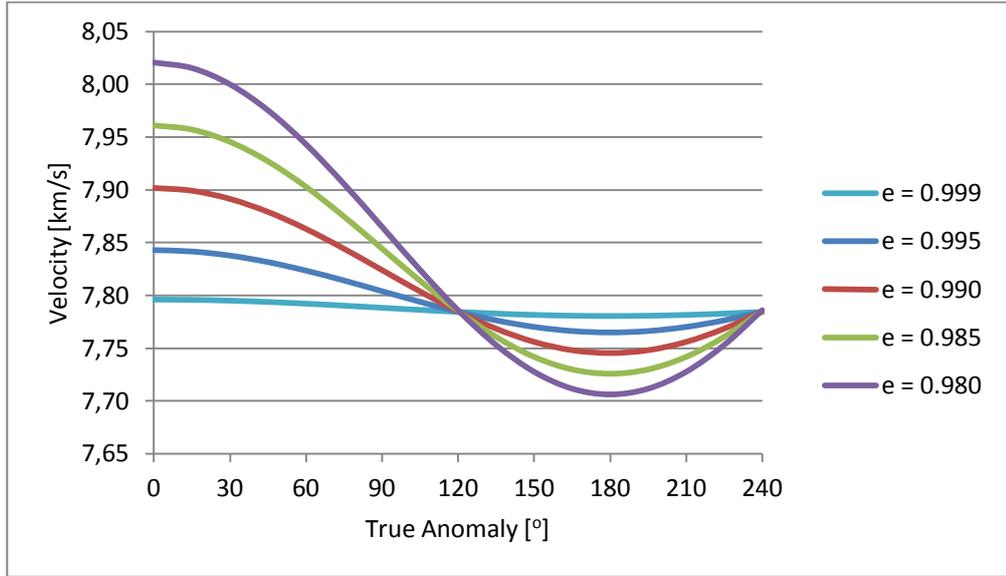
Figure 16 Variation of Orbital Velocity w.r.t. True Anomaly (Elliptic Orbits)
