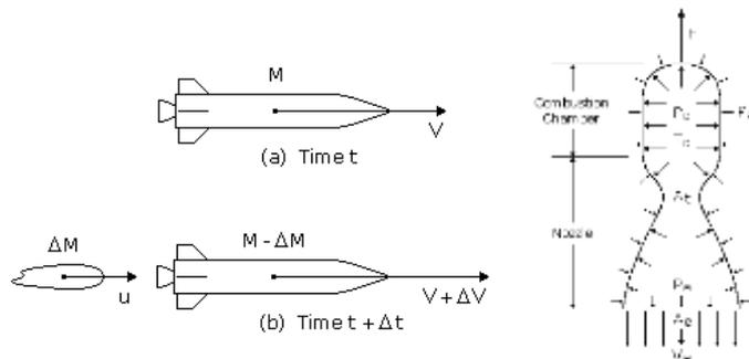
Figure 10 Conservation of Momentum and Derivation of Thrust
