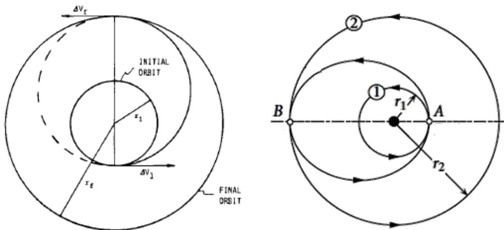
Figure 14 Hohmann Transfer (Chobotov, 2002)
