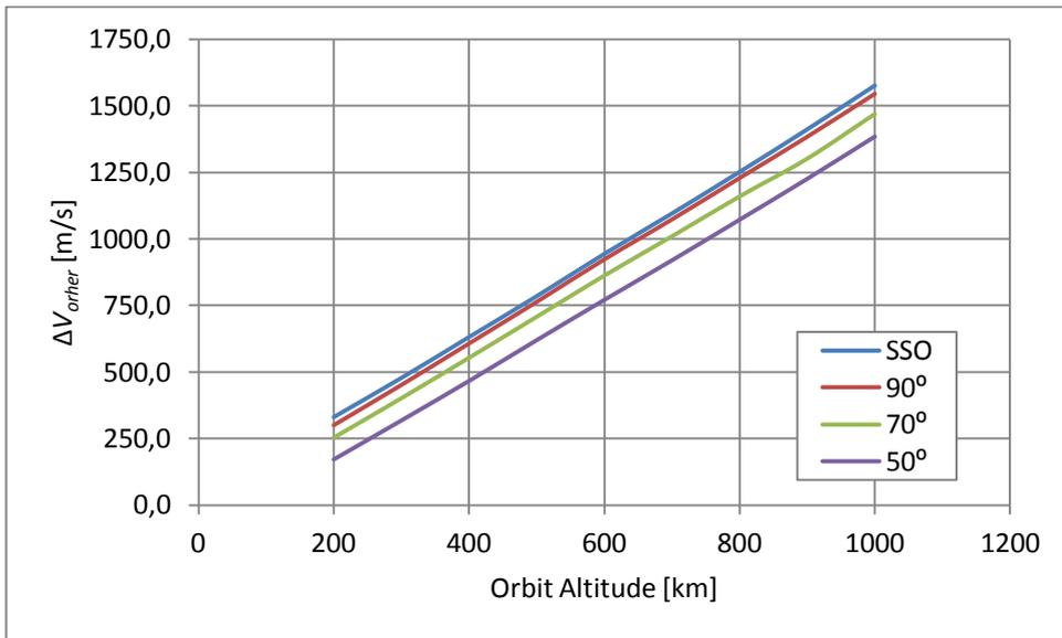
Figure 21 Variation of  $\Delta V_{other}$  for Different Inclinations
