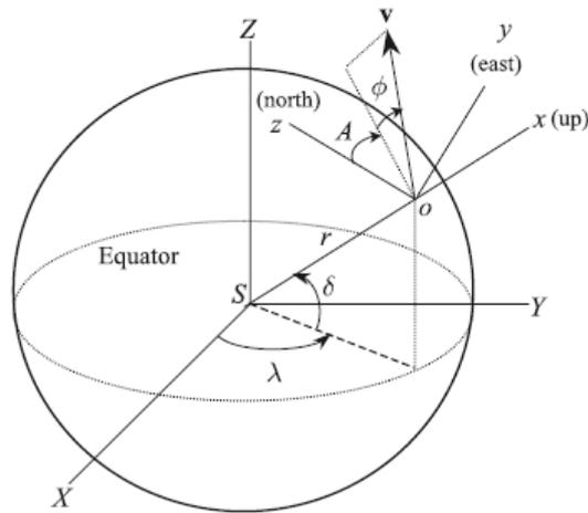
Figure 42 Earth-fixed Reference Frame for Atmospheric Flight (Tewari)
