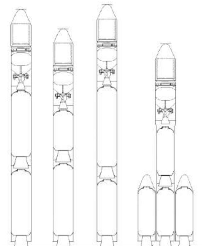
Figure 65 Three Stage Launch Vehicle Alternatives
