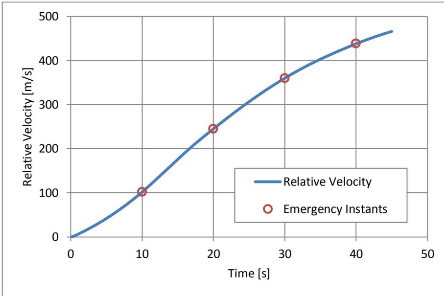
Figure 47 Variation of Relative Velocity on Nominal Trajectory
