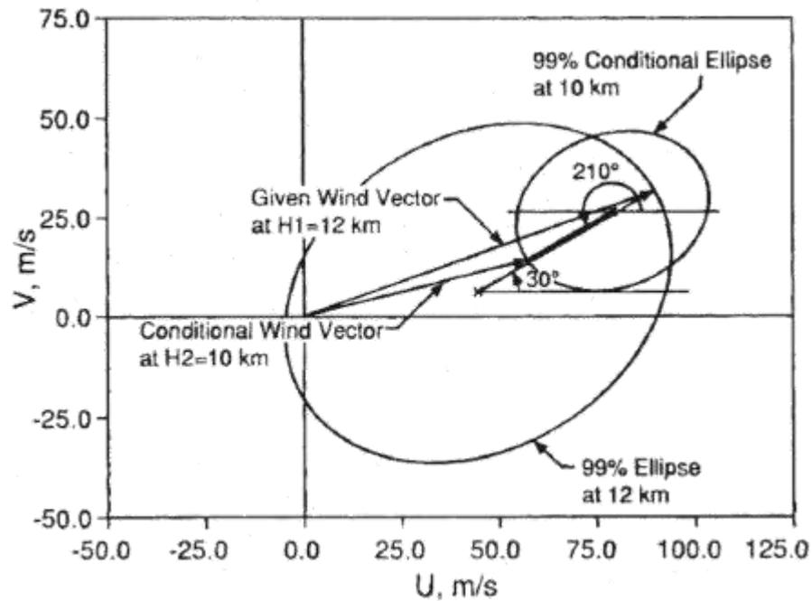
Figure 31 Schematic of Wind Profile Construction (NASA)
