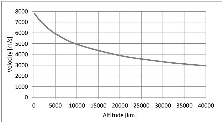
Figure 15 Variation of Orbital Velocity w.r.t. Altitude (Circular Orbit)
