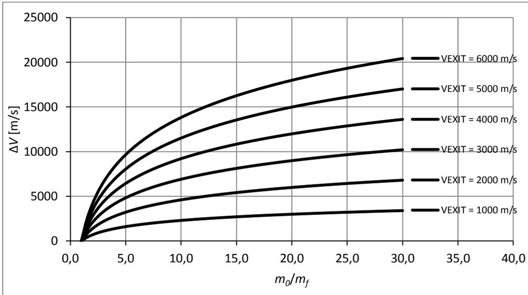
Figure 11 Total Attainable Velocity w.r.t. Mass Fraction
