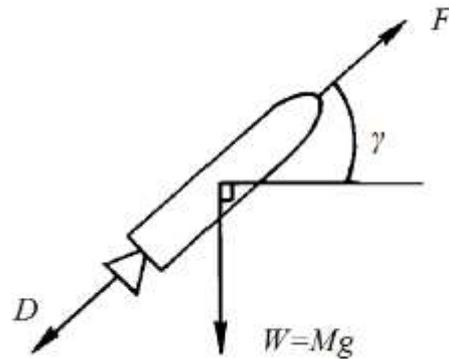
Figure 19 Simple Force Balance on a Launch Vehicle
