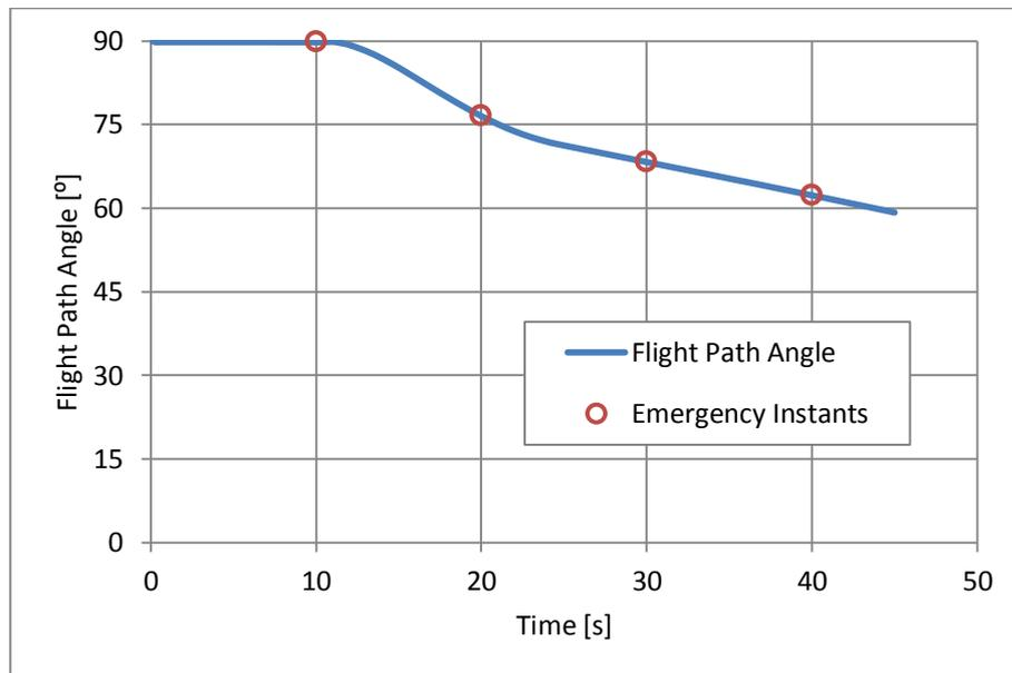
Figure 46 Variation of Flight Path Angle on Nominal Trajectory
