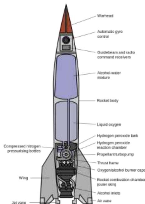
Figure 1 German V-2 Rocket Diagram (NASA)
