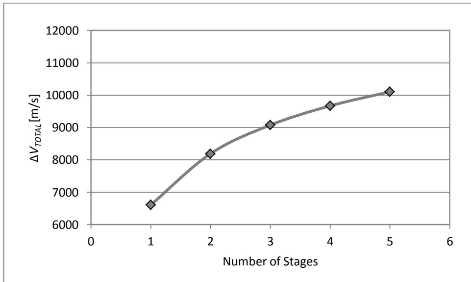
Figure 12 Effect of Staging on Total  $\Delta V_{TOTAL}$
