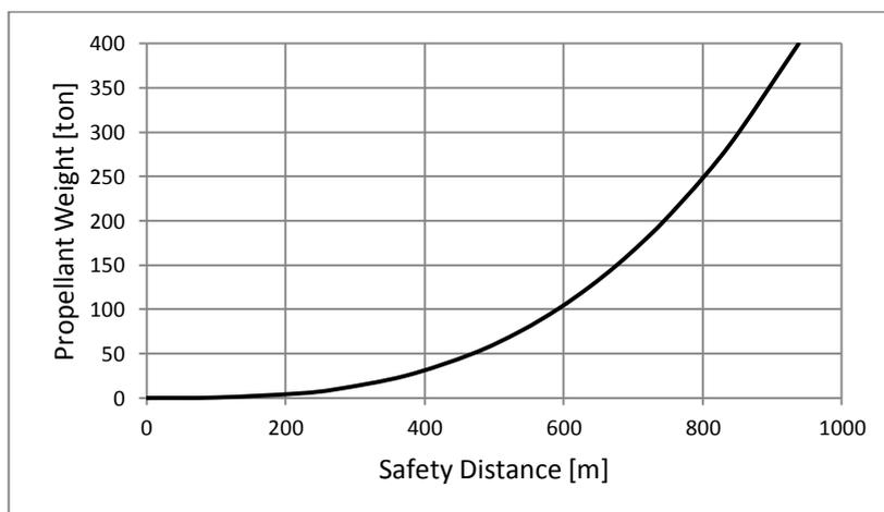
Figure 36 Variation Safety Distance with Propellant Weight
