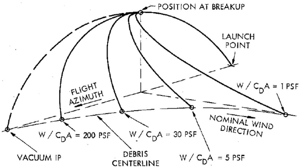
Figure 34 Ballistic Coefficient and Wind Influence on Trajectory (Collins)
