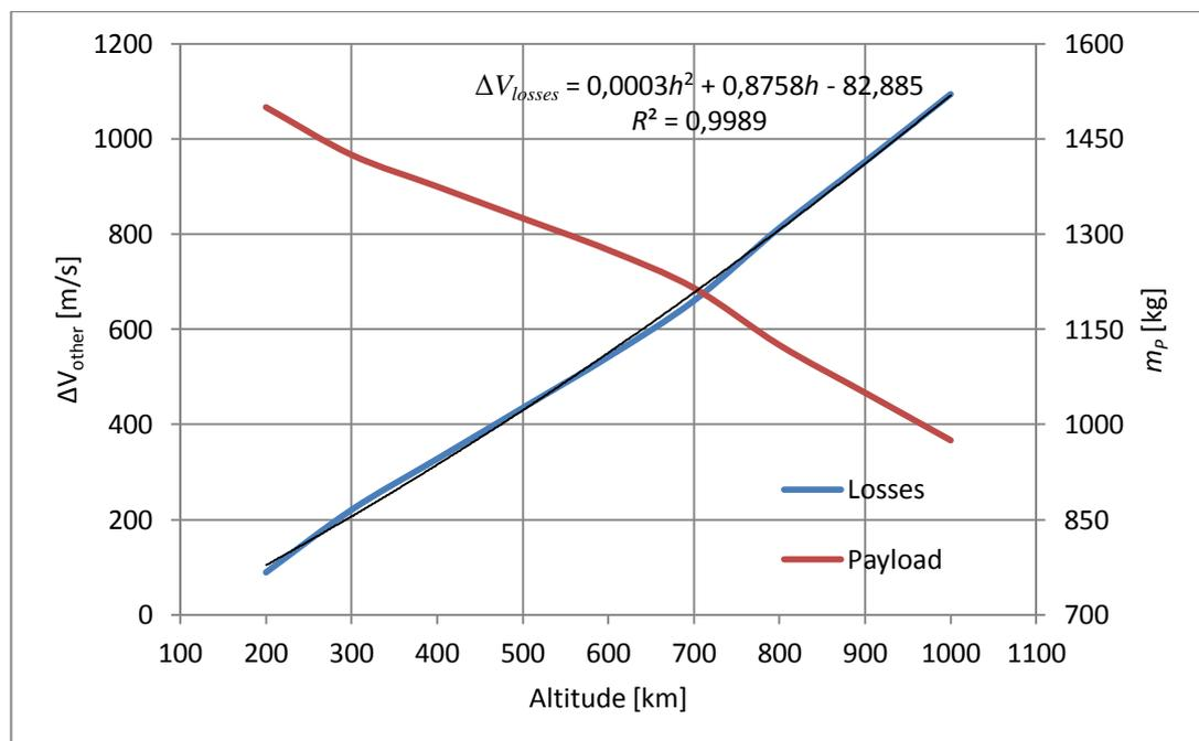
Figure 20 Athena II Launch Vehicle Losses
