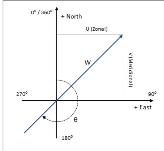
Figure 29 The Meteorological Coordinate System
