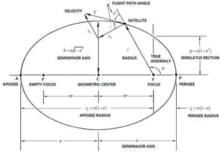
Figure 13 Orbital Parameters on Ellipse Geometry (Chobotov, 2002)
