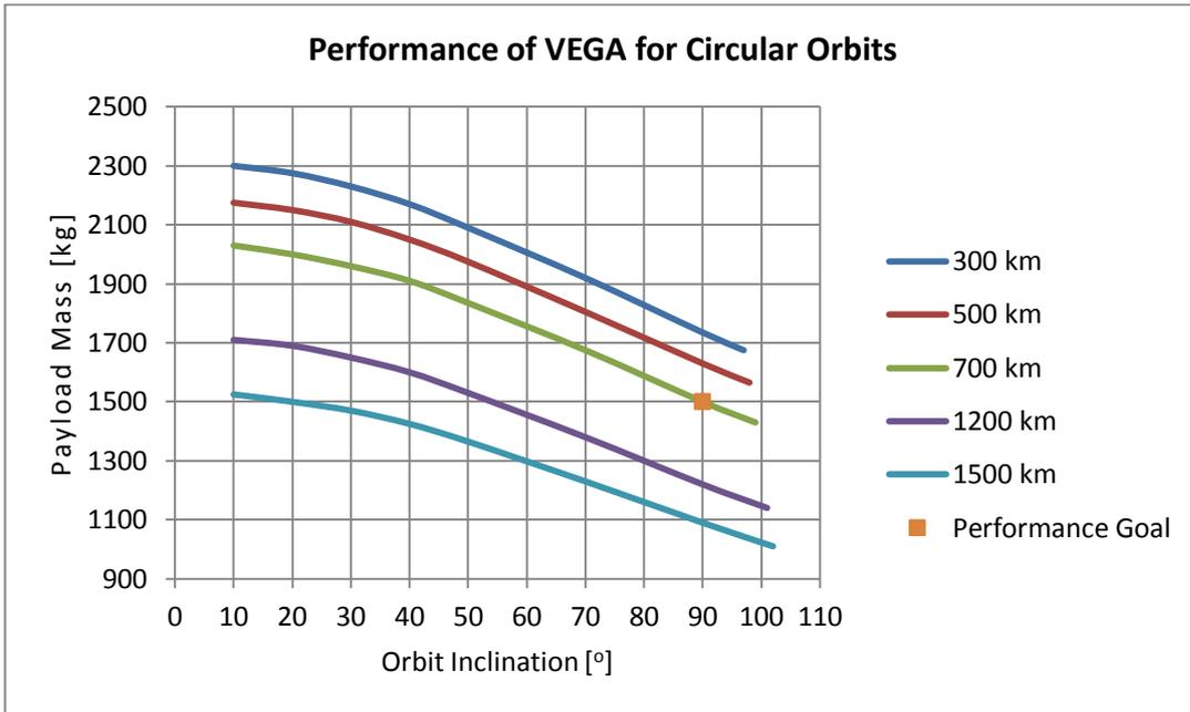
Figure 9 Performance of VEGA Launch Vehicle for Circular Orbits
