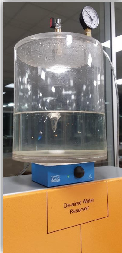
Figure 25: De-Airing Water Tank
