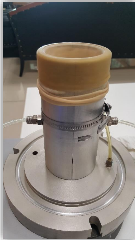
Figure 38: Sample Preparation - Split mould with membrane installed on the base
