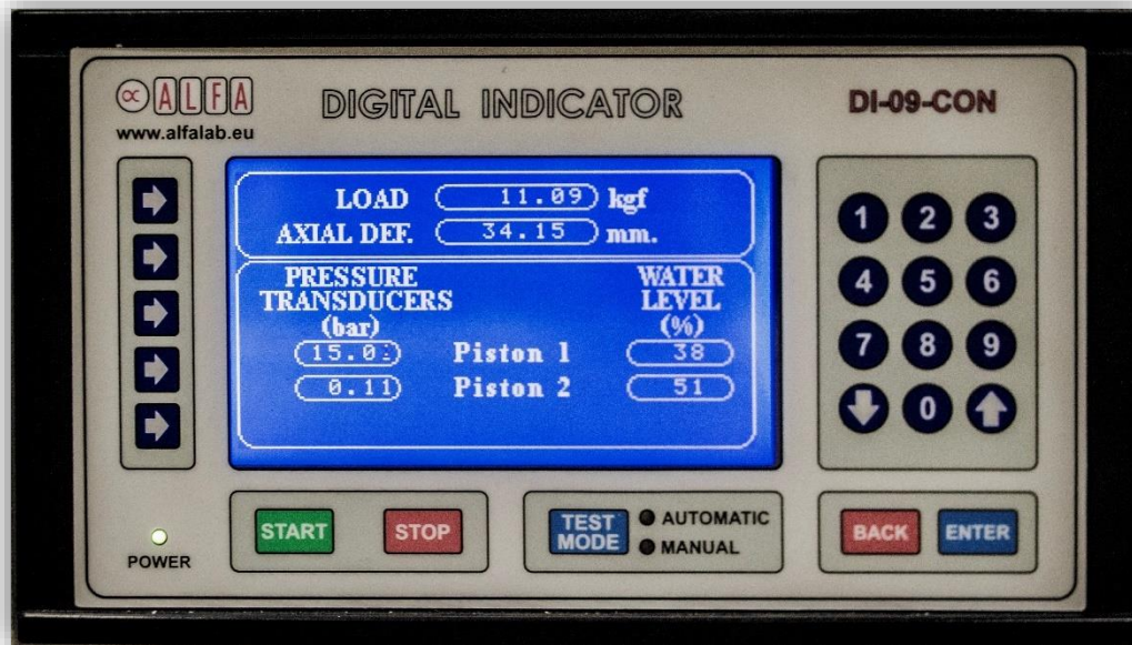
Figure 20: Data Acquisition and Control System - LCD Monitor
