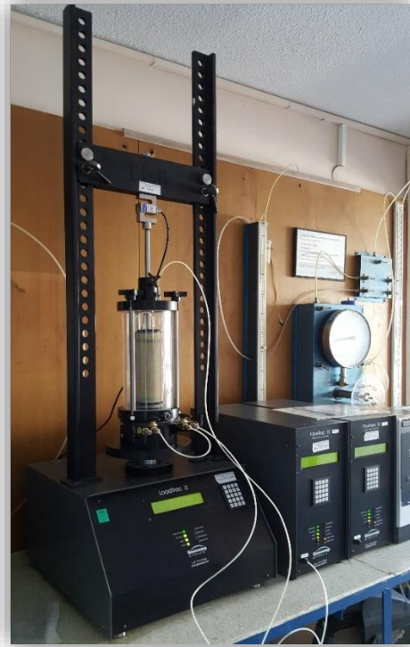
Figure 41: Geocomp's Triaxial Test Setup at Toker Laboratory (Private Laboratory)
