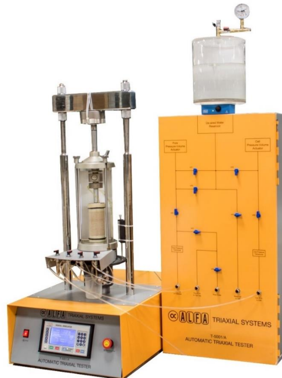
Figure 42: ALFA's Triaxial Test Setup at ALFA Research and Development Department
