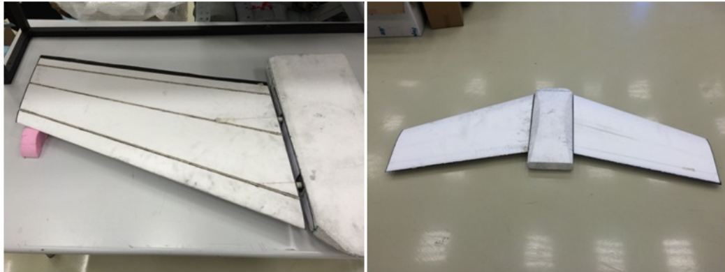
Figure 3.21: Checking the fitting of connection spars of Wing Piece 1 to fuselage
