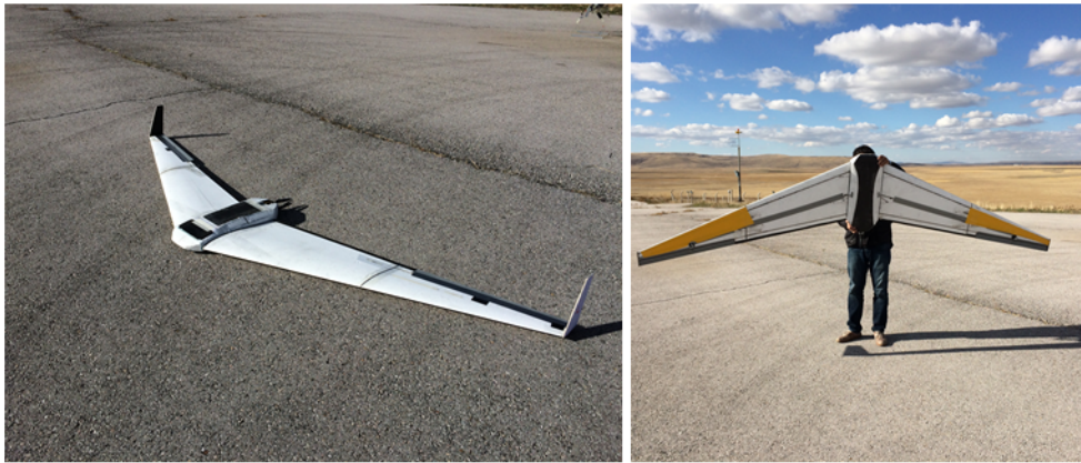
Figure 4.13: Fully assembled UAV prototype ready for RC maiden flight
