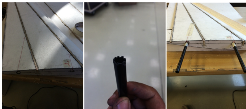
Figure 3.14: Drawing guide lines, shaping one side of the spar as teeth and integration of spars
