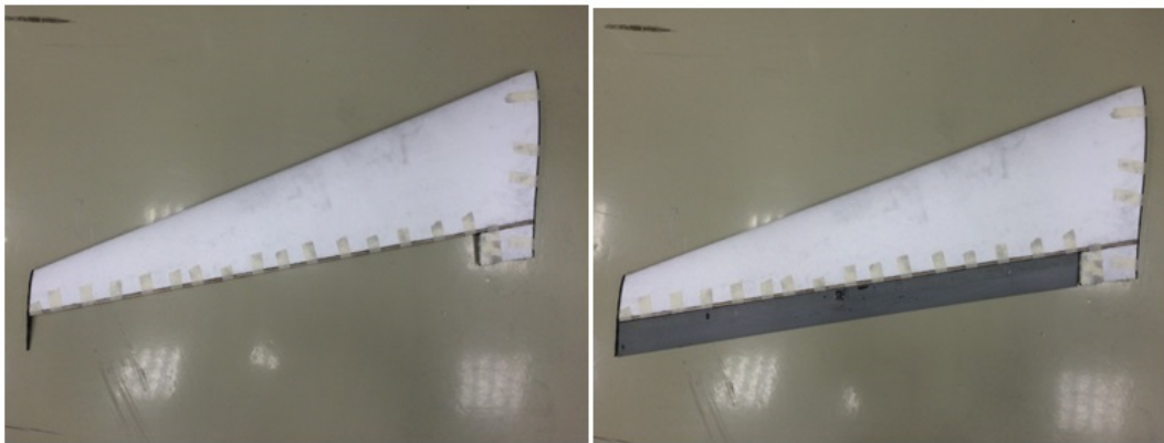
Figure 3.12: Gluing of rear spar and control surface production
