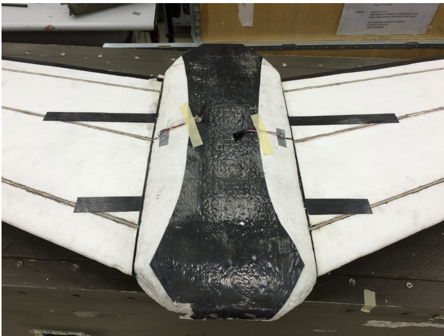
Figure 4.16: Addition of Carbon layer and adhesive to root spars of the wings
