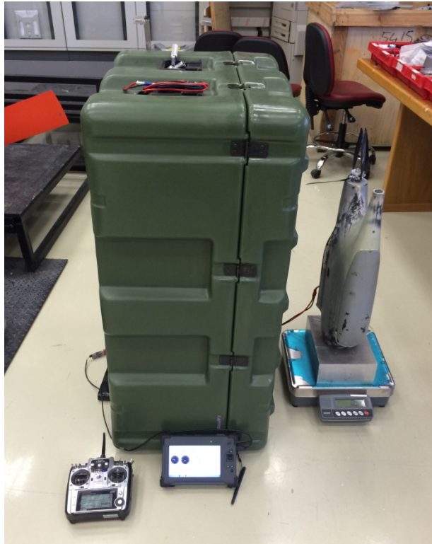
Figure 4.1: Motor Thrust Test setup
