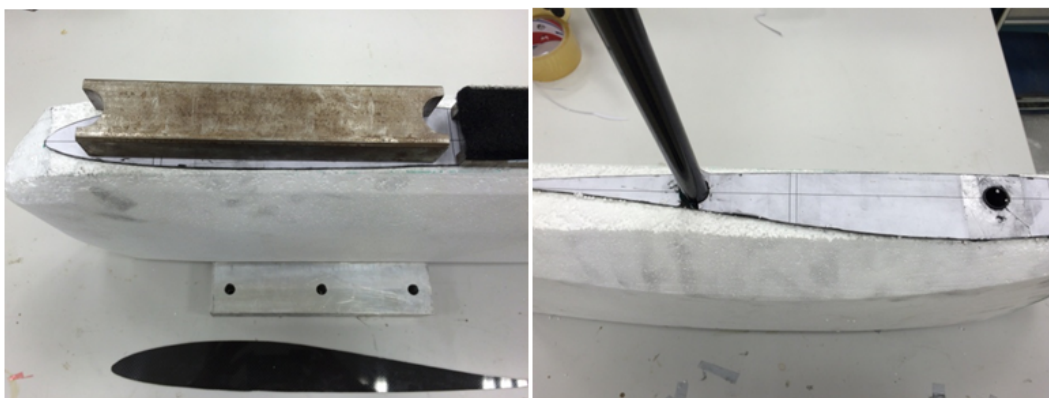
Figure 3.20: Gluing of end ribs to the fuselage and integration of main spars
