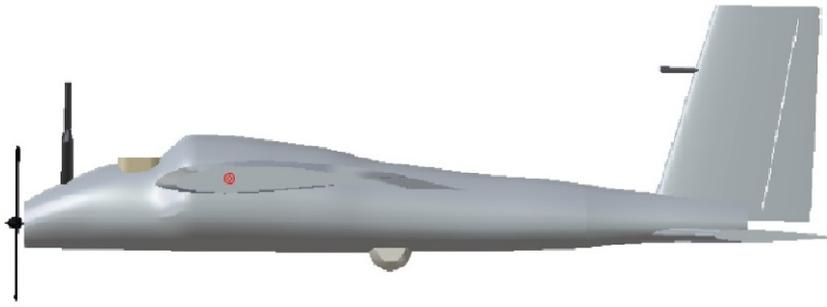
Figure A.9: Centre of gravity location of the UAV from the side view
