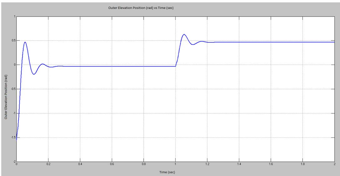
**Figure 5.20:** Outer Elevation Position Step Response with SMC
