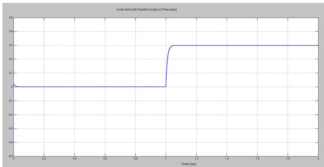
**Figure 5.16:** Inner Azimuth Step Response with Automatically Tuned PID Controller to 0.3 rad Step Input
