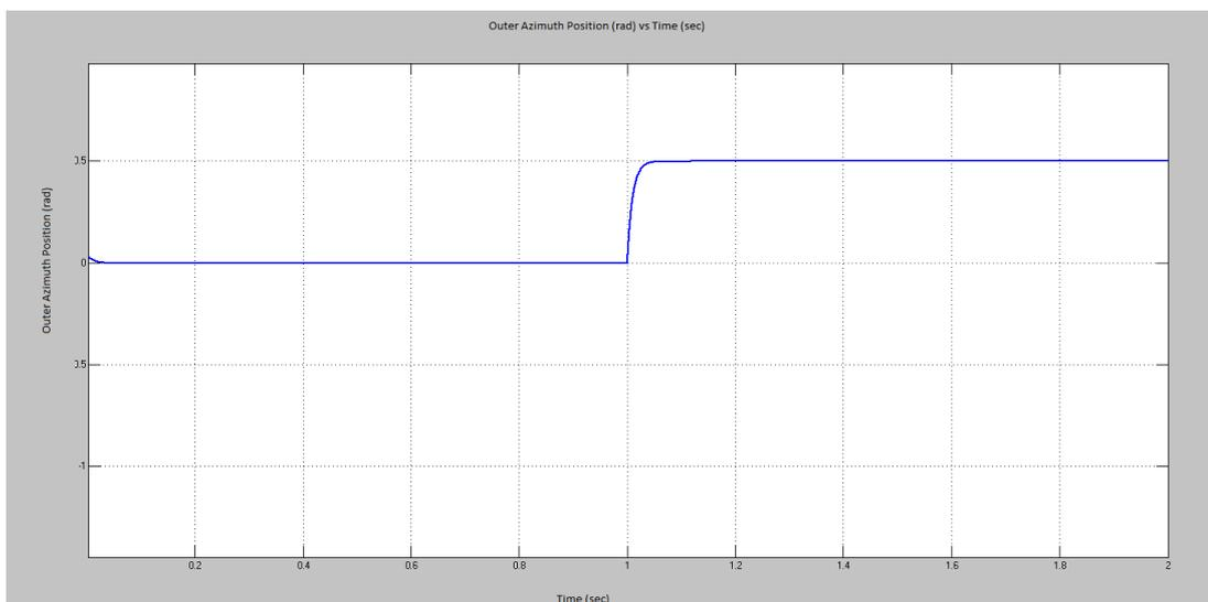
**Figure 5.9:** Outer Azimuth Step Response with Automatically Tuned PID Controller to 0.5 rad Step Input
