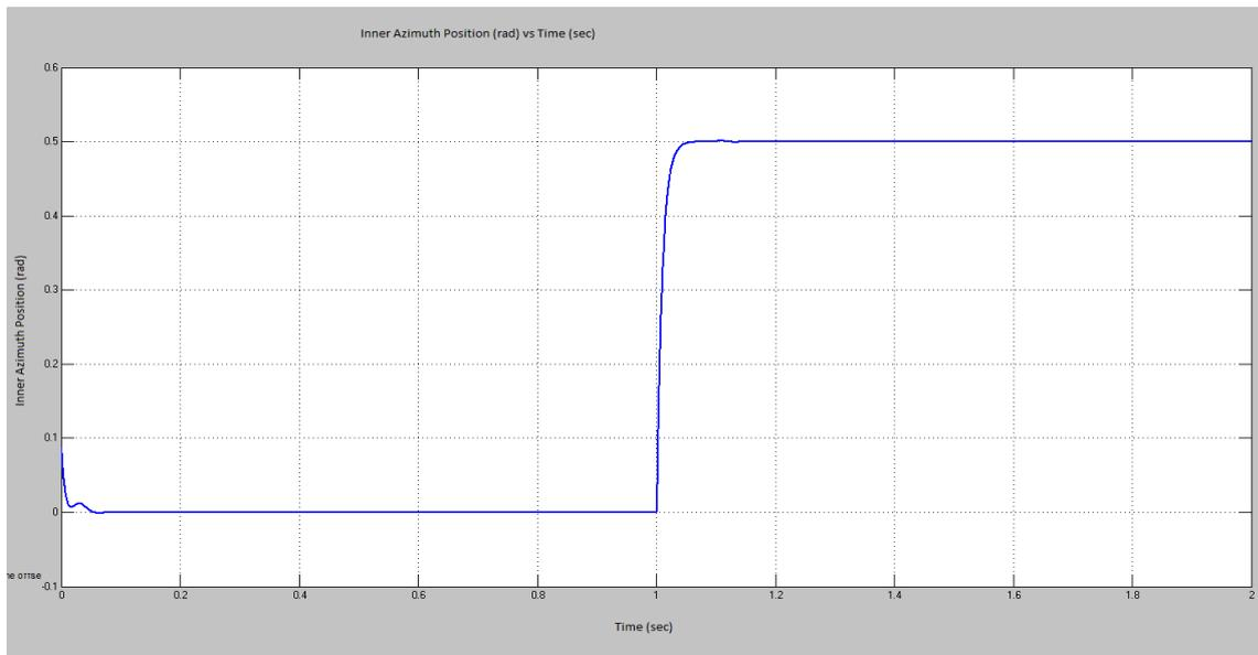
**Figure 5.22:** Inner Azimuth Position Step Response with SMC
