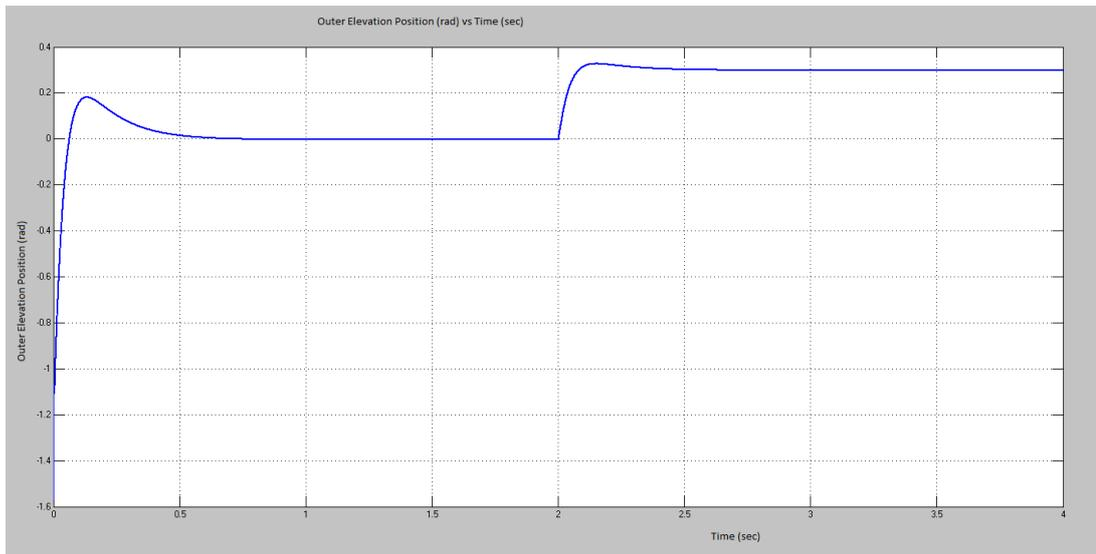
**Figure 5.4:** Outer Elevation Step Response with PID Controller to 0.3 rad Step Input
