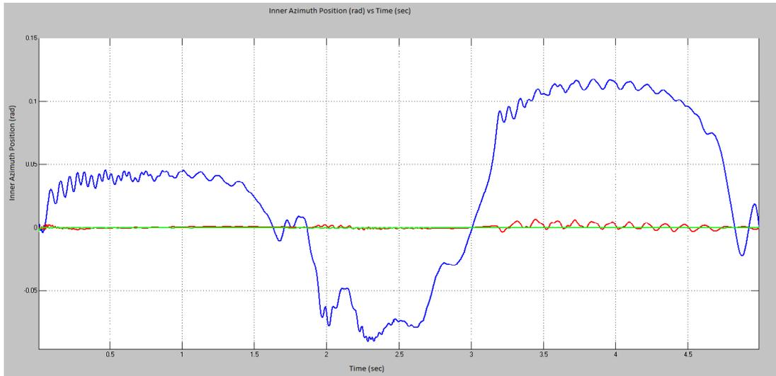
**Figure 5.33:** Stabilization with Automatically Tuned PID on Disturbance 1
