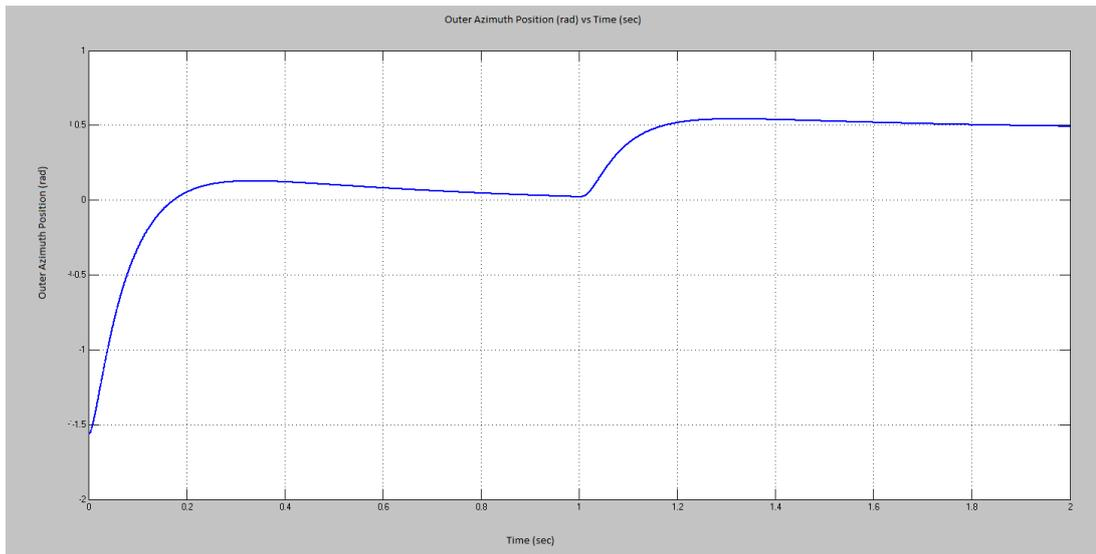
**Figure 5.1:** Outer Azimuth Step Response with PID Controller to 0.5 rad Step Input
