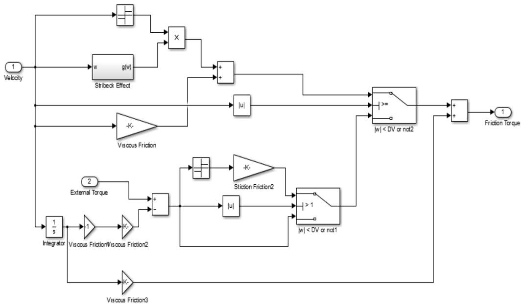
**Figure 4.3:** Karnopp Friction Simulation Model
