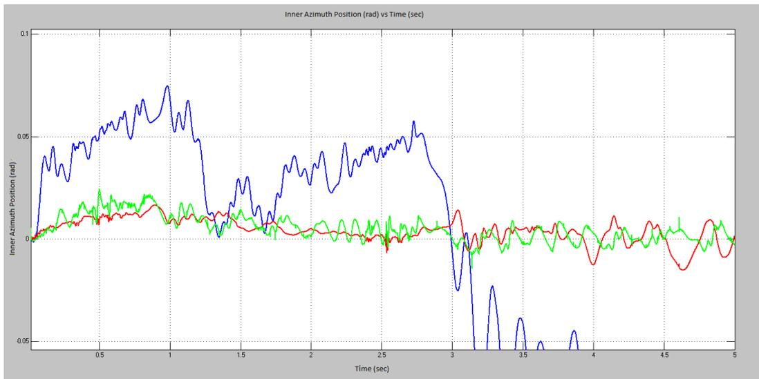
**Figure 5.30:** Stabilization with PID on Disturbance 3
