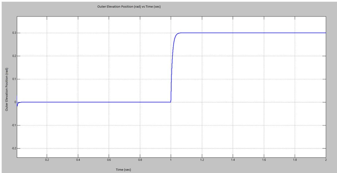
**Figure 5.12:** Outer Elevation Step Response with Automatically Tuned PID Controller to 0.3 rad Step Input
