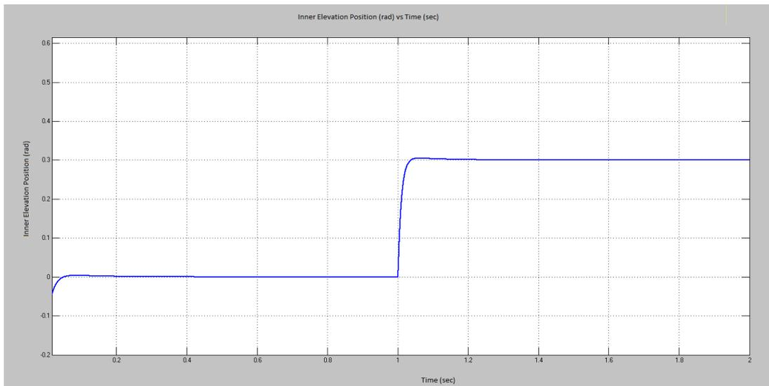
**Figure 5.14:** Inner Elevation Step Response with Automatically Tuned PID Controller to 0.3 rad Step Input
