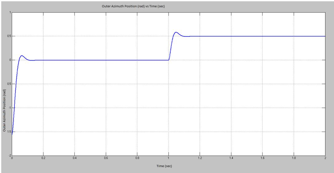
**Figure 5.19:** Outer Azimuth Position Step Response with SMC
