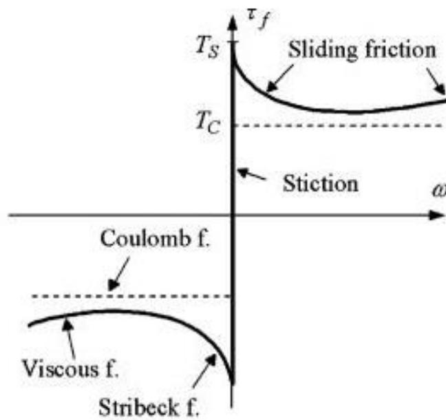
**Figure 2.3:** Coulomb, viscous and Stribeck Model of Friction [13]
