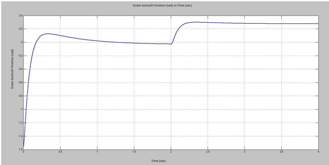
**Figure 5.2:** Outer Azimuth Step Response with PID Controller to 0.3 rad Step Input
