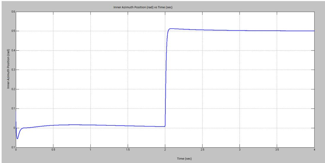
**Figure 5.7:** Inner Azimuth Step Response with PID Controller to 0.5 rad Step Input
