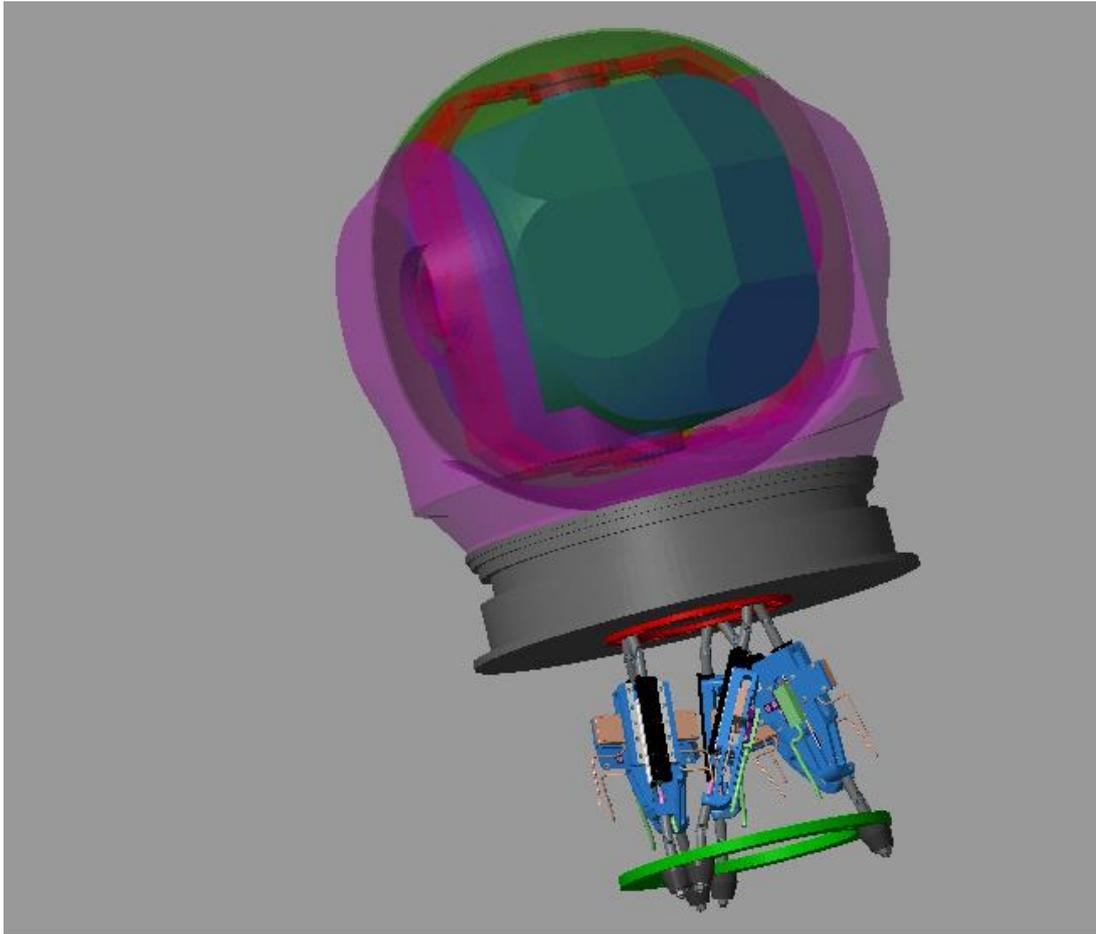
**Figure 4.9:** 4-DOF Platform Placed on the Stewart Platform
