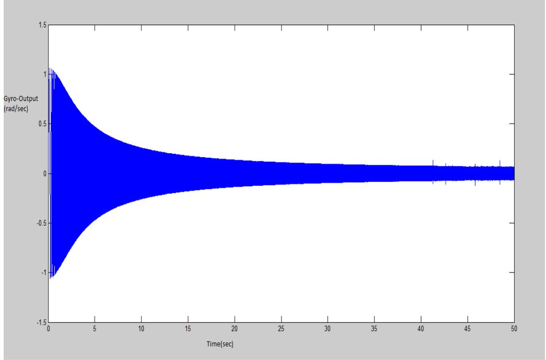
**Figure 3.4:** Gyro Output Data with 1Hz-to-1kHz Chirp Input
