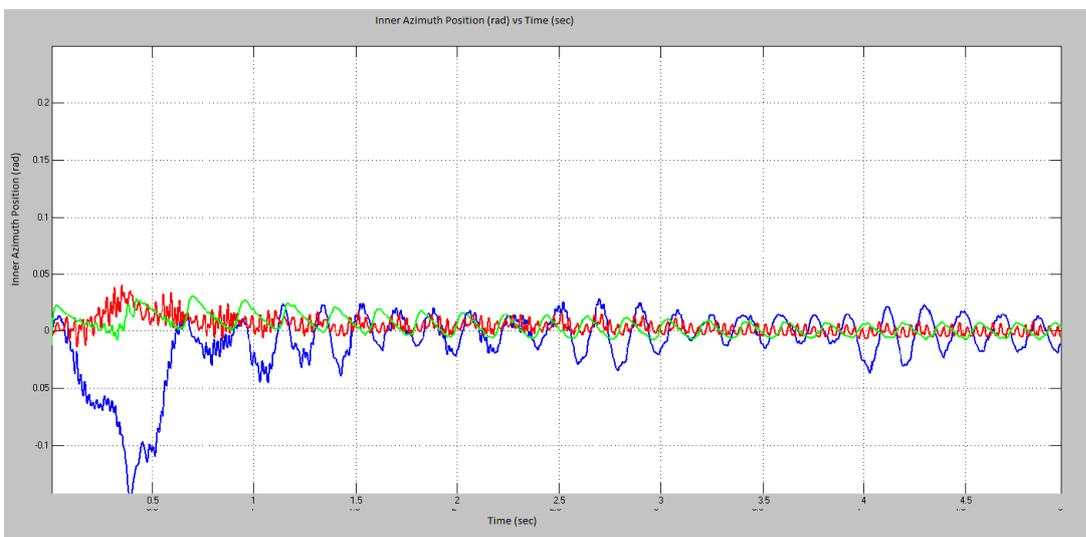
**Figure 5.32:** Stabilization with PID on Disturbance 5
