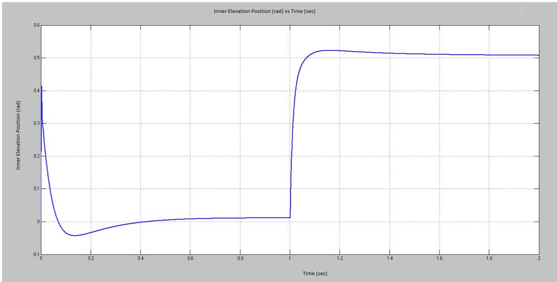
**Figure 5.5:** Inner Elevation Step Response with PID Controller to 0.5 rad Step Input
