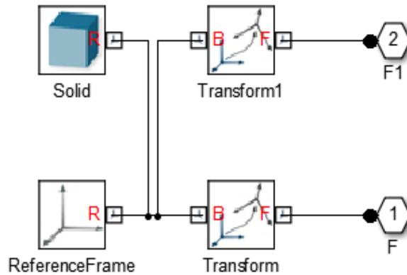
**Figure 4.2:** A Rigid Body Simulation Block
