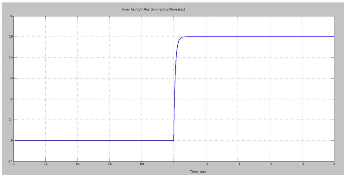
**Figure 5.15:** Inner Azimuth Step Response with Automatically Tuned PID Controller to 0.5 rad Step Input
