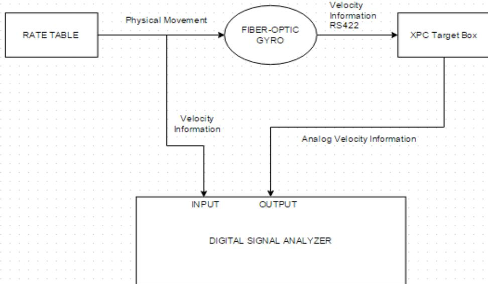
**Figure 3.2:** Gyroscope Test Setup Block Diagram
