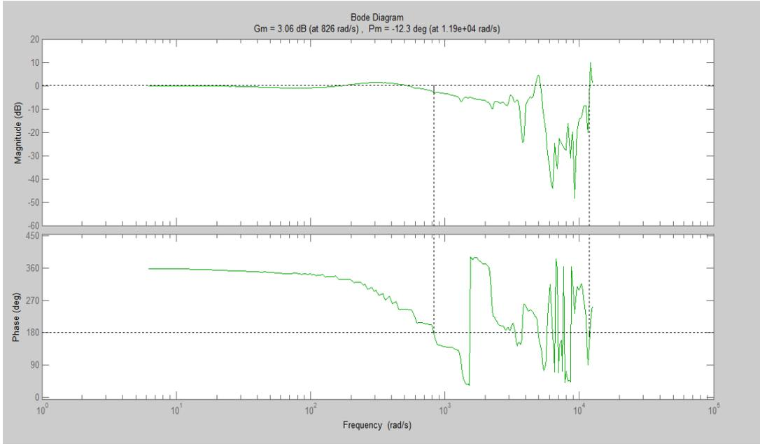
**Figure 3.3:** Gyroscope Frequency Domain Data
