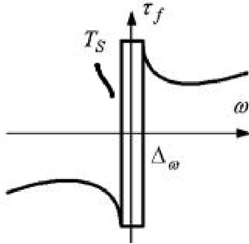
**Figure 2.4:** Karnopp Friction Model Containing Hysteresis Loop [13]
