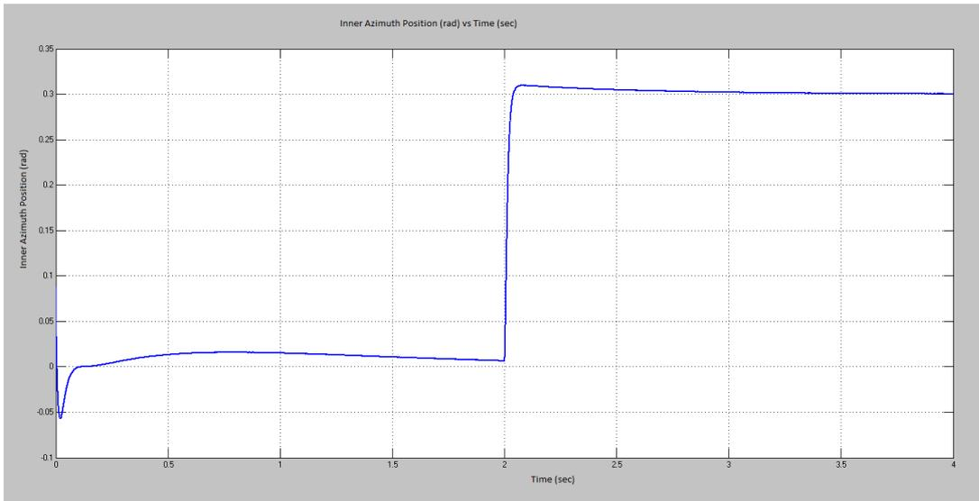
**Figure 5.8:** Inner Azimuth Step Response with PID Controller to 0.3 rad Step Input
