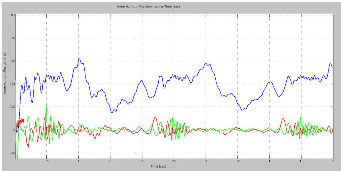
**Figure 5.40:** Stabilization with SMC on Disturbance 3
