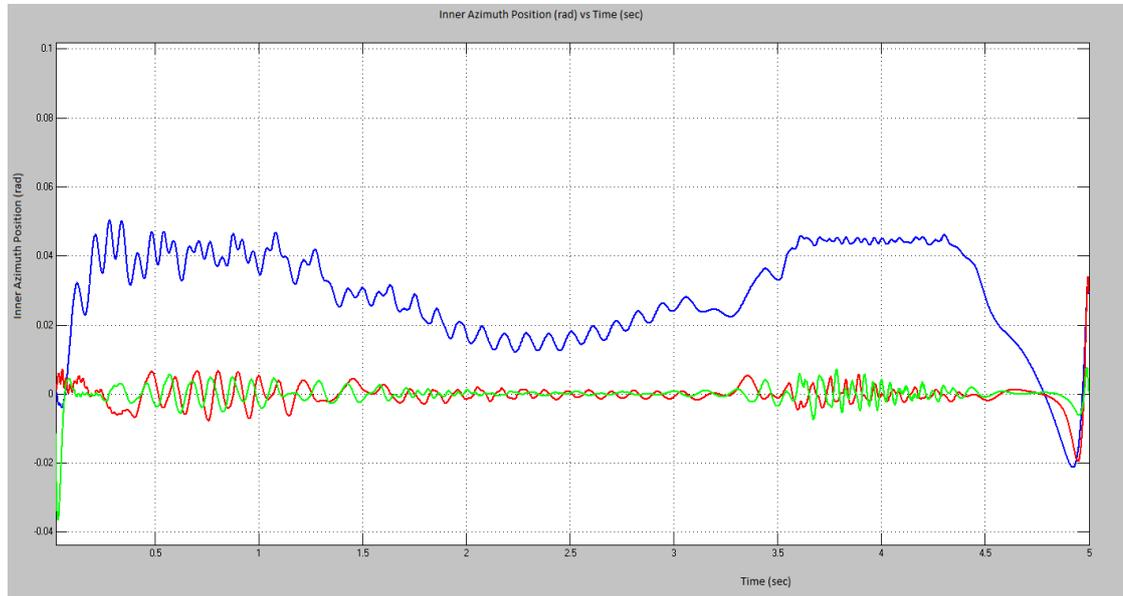
**Figure 5.38:** Stabilization with SMC on Disturbance 1
