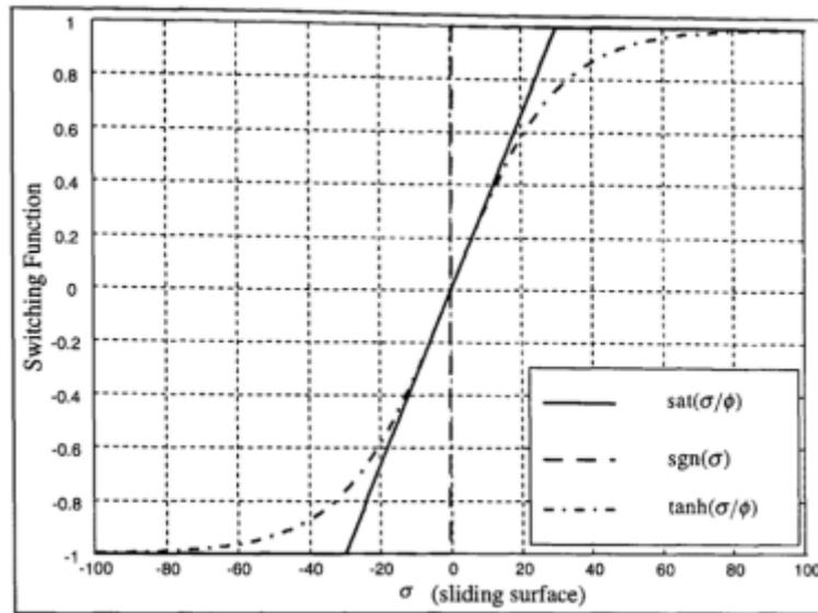
**Figure 5.18:** Switching Function vs. Sliding Surface [31]
