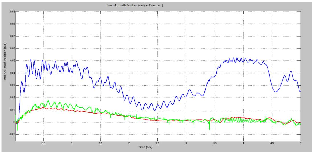
**Figure 5.28:** Stabilization with PID on Disturbance 1
