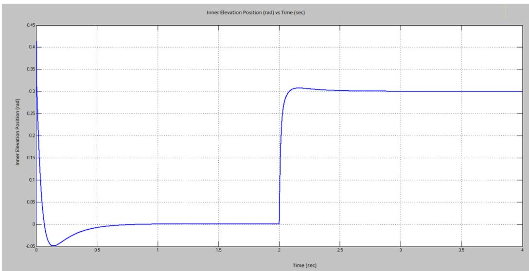
**Figure 5.6:** Inner Elevation Step Response with PID Controller to 0.3 rad Step Input
