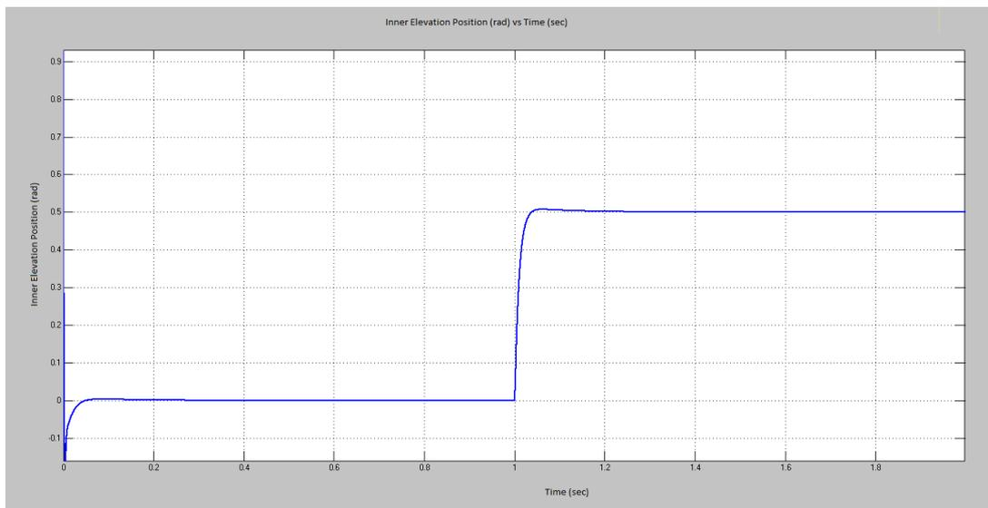
**Figure 5.13:** Inner Elevation Step Response with Automatically Tuned PID Controller to 0.5 rad Step Input
