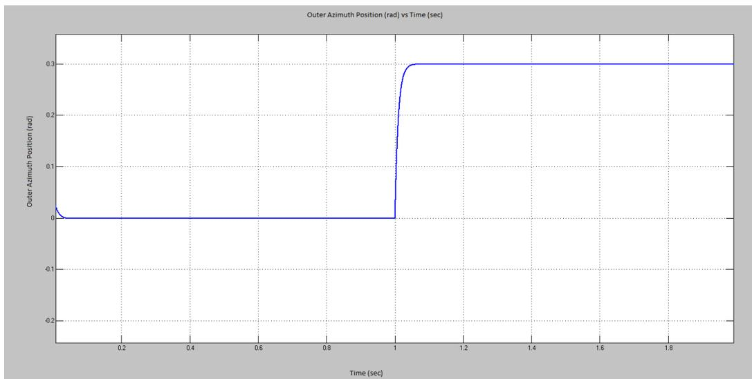
**Figure 5.10:** Outer Azimuth Step Response with Automatically Tuned PID Controller to 0.3 rad Step Input
