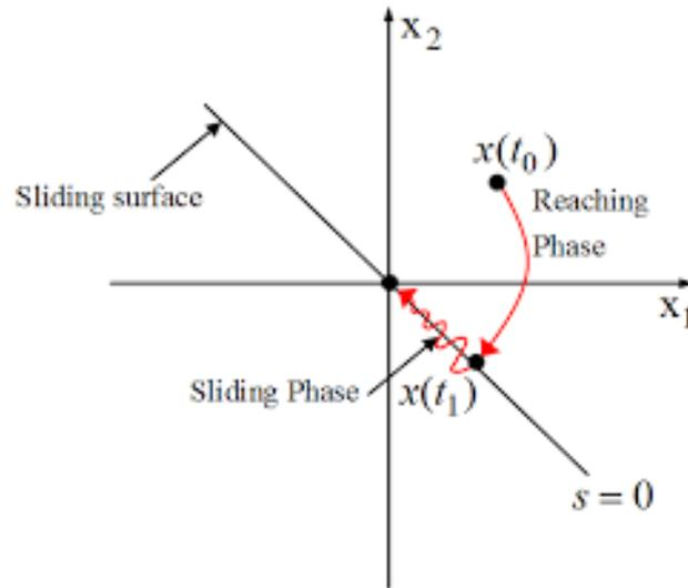
**Figure 5.17:** Sliding Surface and the State Trajectory [27]
