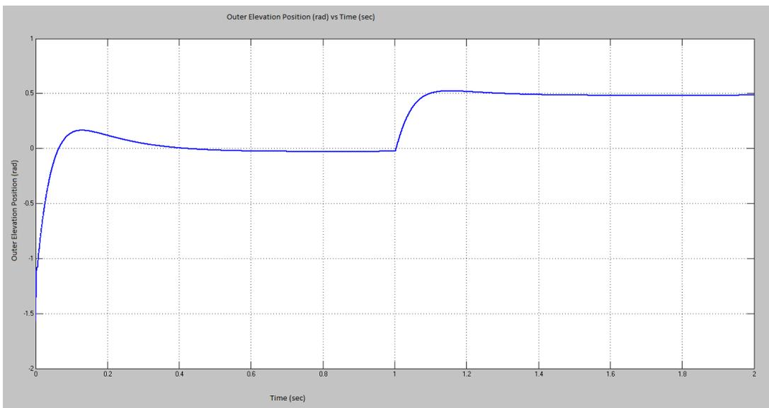
**Figure 5.3:** Outer Elevation Step Response with PID Controller to 0.5 rad Step Input
