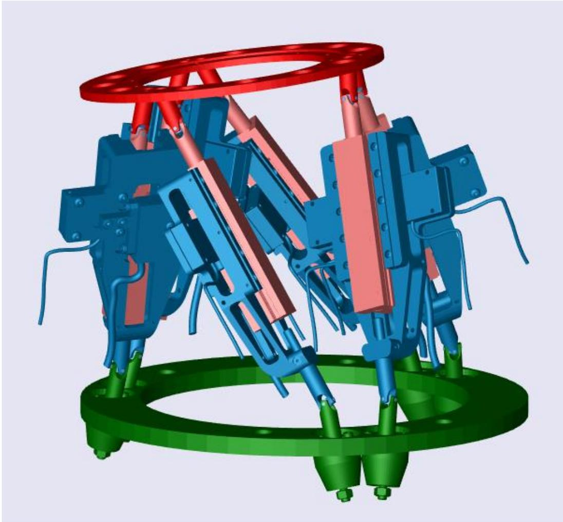
**Figure 4.7:** 3-D Simulation View of Stewart Platform
