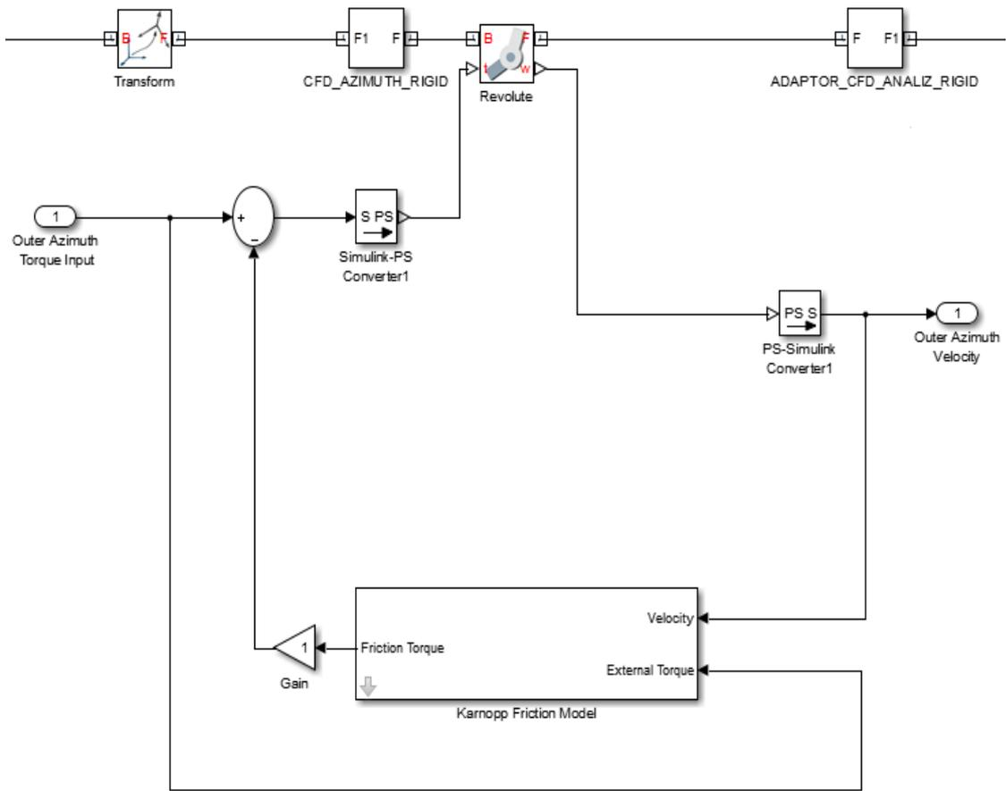
**Figure 4.4:** Friction Model Inserted into the Simulation Model
