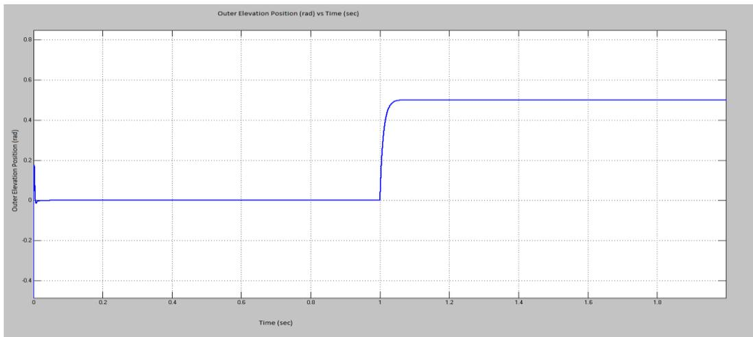
**Figure 5.11:** Outer Elevation Step Response with Automatically Tuned PID Controller to 0.5 rad Step Input
