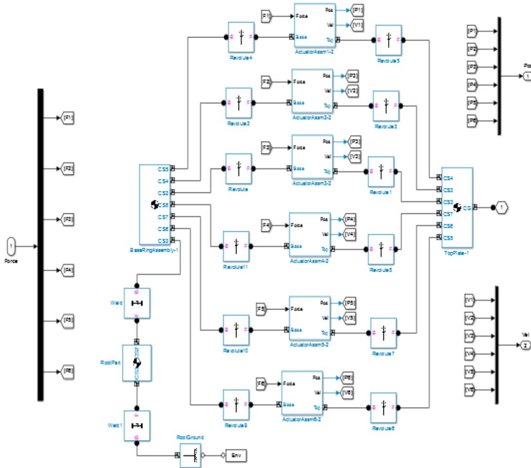
**Figure 4.6:** Simulation Blocks for the Stewart Platform
