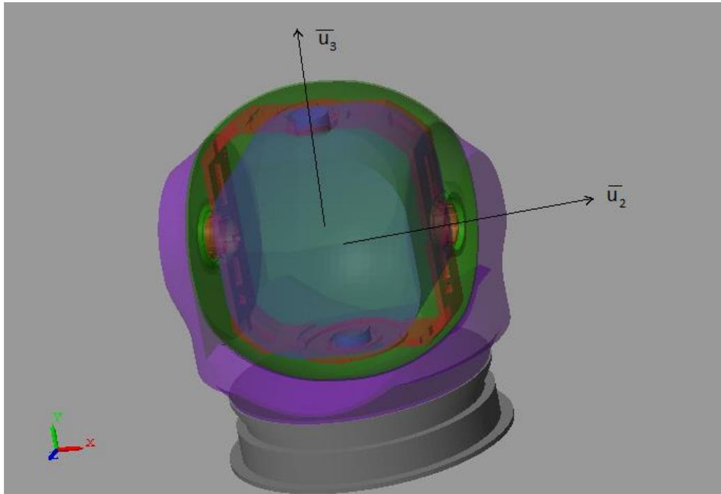
**Figure 2.2:** Unit Directions on the 4-DOF Gimbal
