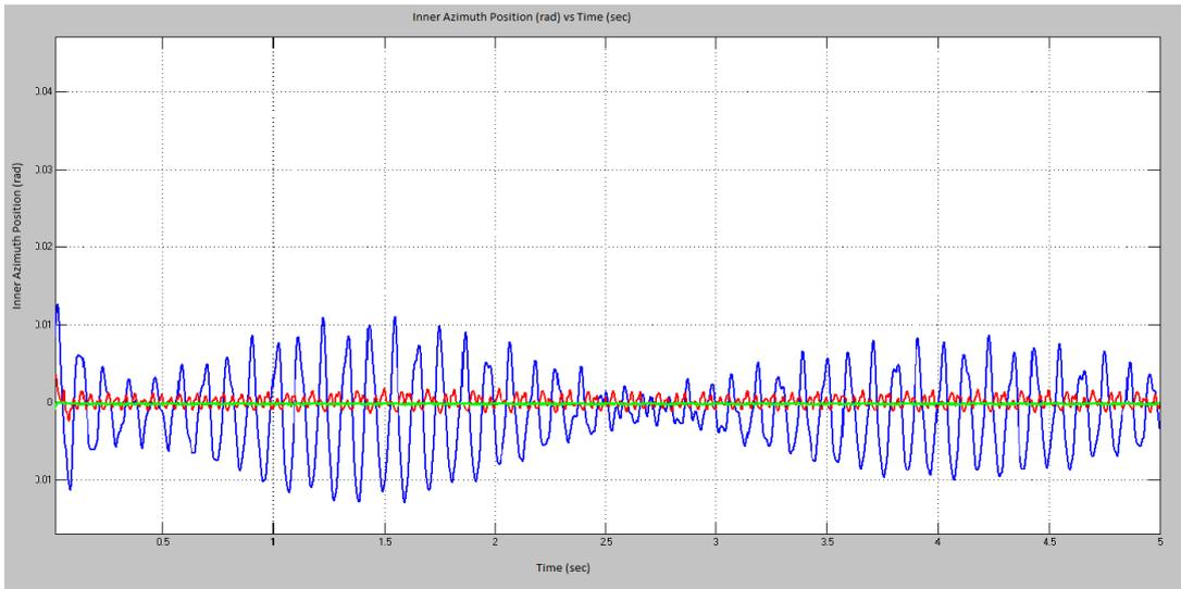
**Figure 5.37:** Stabilization with Automatically Tuned PID on Disturbance 5
