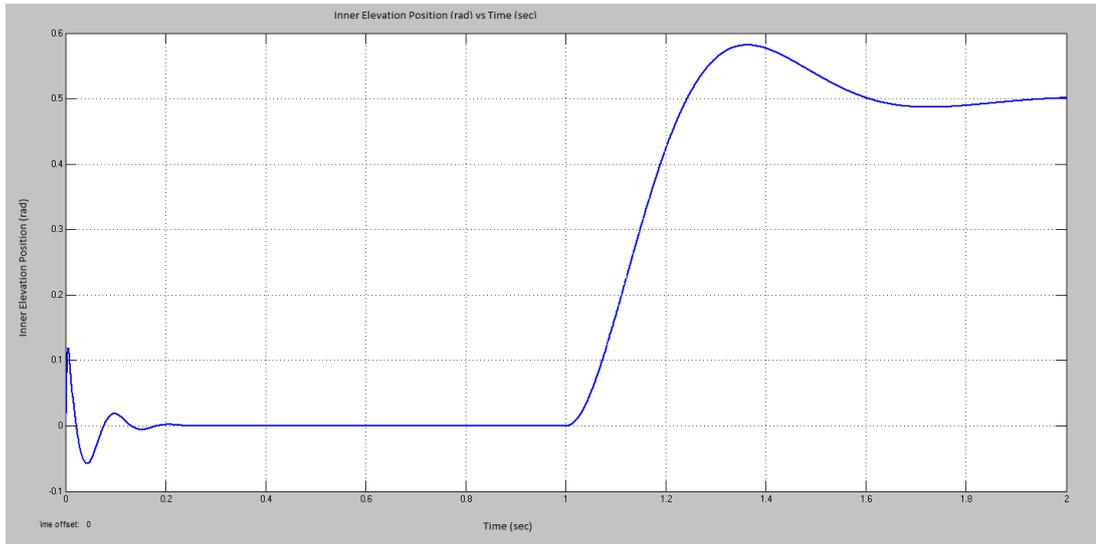
**Figure 5.21:** Inner Elevation Position Step Response with SMC
