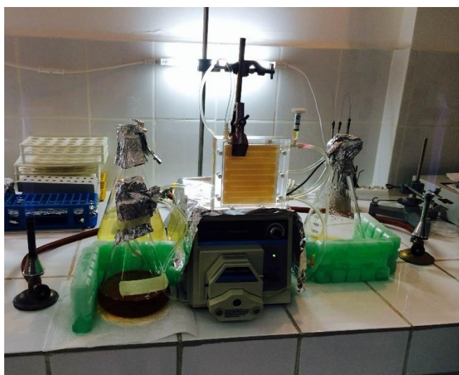
Figure 2. 1. 30kDa molecular cut-off ultrafilter set up unit for concentration of the K5 type yeast killer protein.
