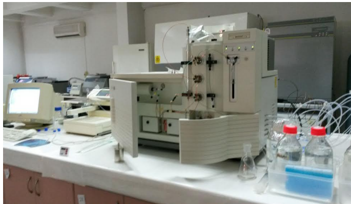
Figure 2. 2. FPLC for Gel permeation chromatography for purification of the K5 type yeast killer protein.
