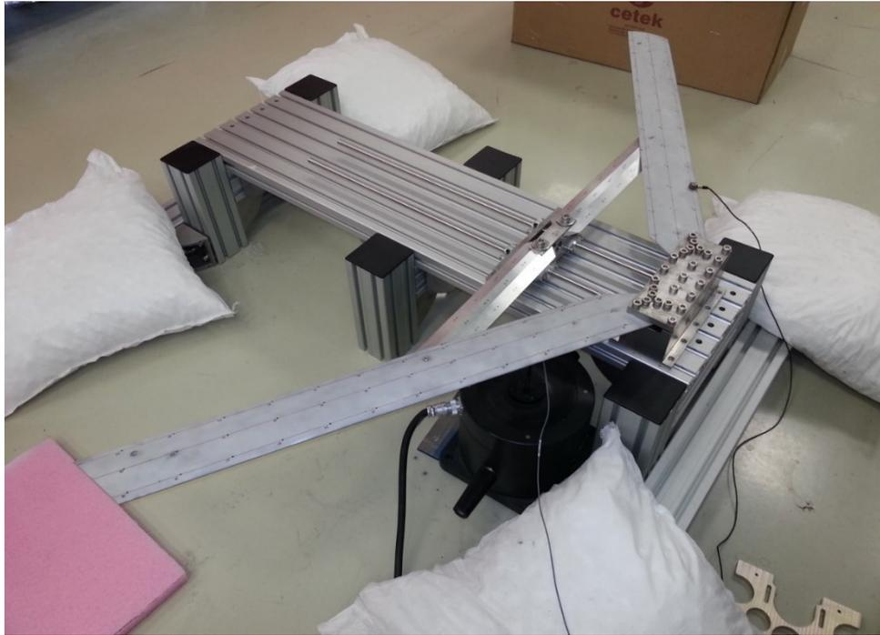
**Figure 5.23.** Test setup for shaker test of the Design Point 1
