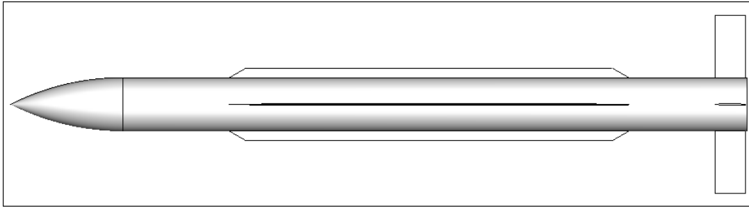
Figure 3.25 The optimum strake planform geometry and placement obtained by gradient optimization (+ view)
