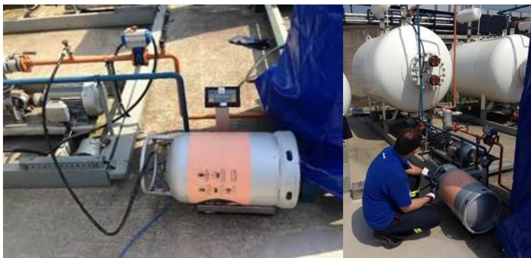
Figure 4.2: Transfer of LPG and olefins into tanks
