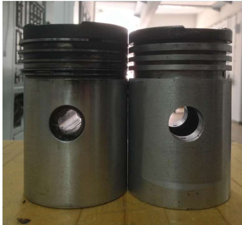
Figure 3.2: Comparison of piston height before (on the right hand side) and after reconditioning (on the left hand side)
