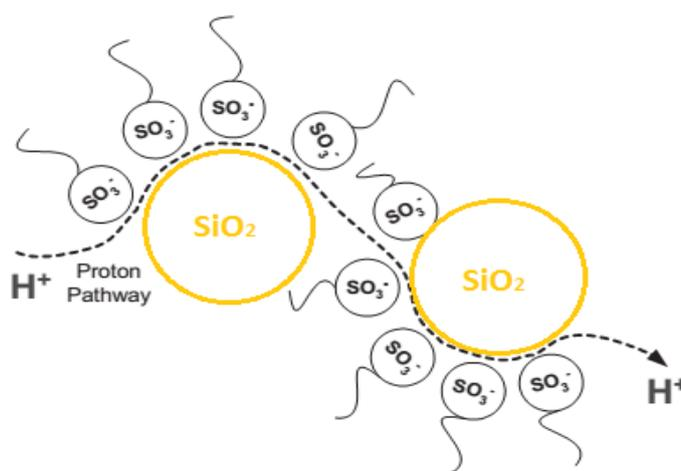
**Figure 44.** Representative view of proton transport in composite membrane including SiO<sub>2</sub> particles
