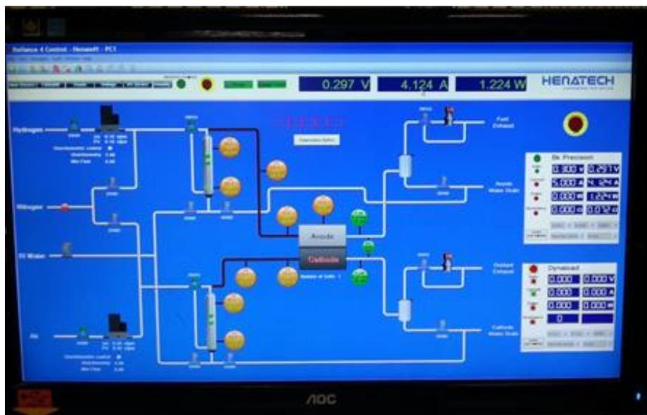
**Figure 47.** A representative PEMFC performance of M1 (2.5 wt. %) at 100 % RH of test station interface at METU Chemical Engineering Fuel Cell Laboratory (Anode: 0.1 slpm H<sub>2</sub> @ 100 % RH, Cathode: 0.42 slpm Compressed Dry Air @ 100 % RH)
