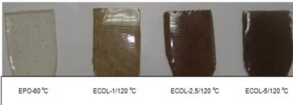
**Figure 3.4:** Color differences of the ECOL samples as a function of boron mineral loading (at 120 °C)
