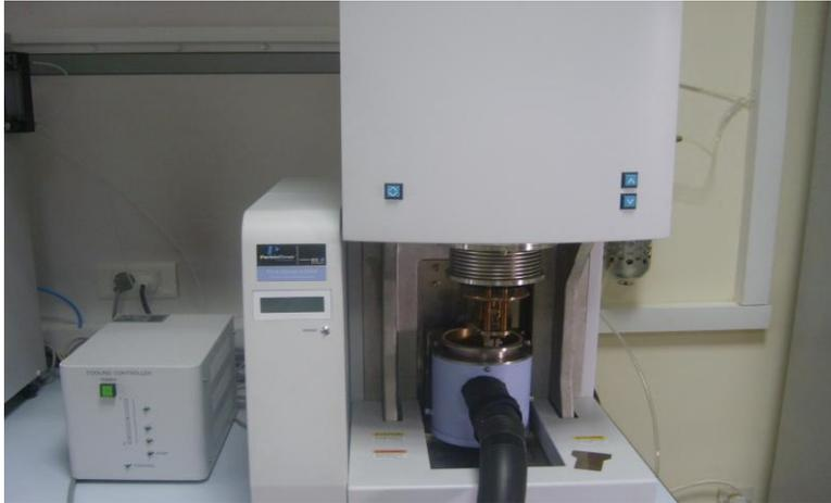
**Figure 2.5:** Perkin Elmer Pyris Diamond DMA
