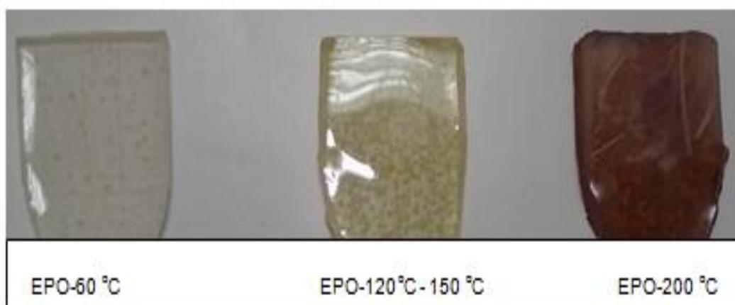
**Figure 3.1:** Color differences of the EPO samples as a function of curing temperature
