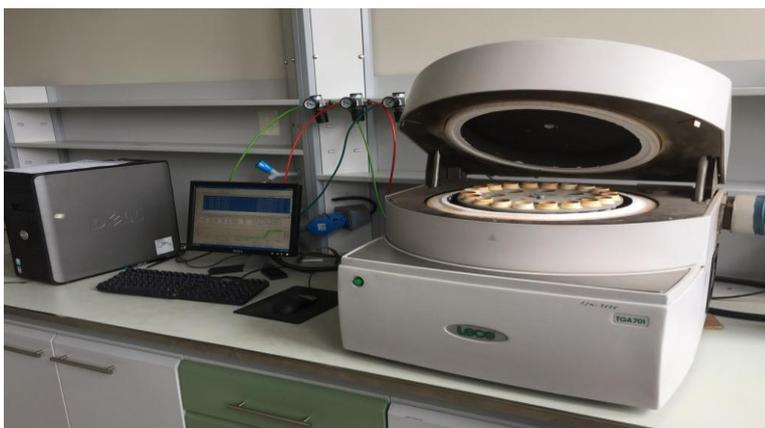
**Figure 2.6:** LECO TGA701 Thermogravimetric Analyzer
