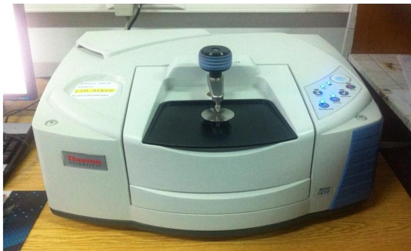
**Figure 2.4:** Thermo Nicolet iS10 ATR-FTIR Spectrometer
