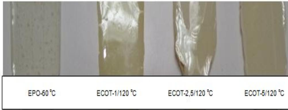
**Figure 3.6:** Color differences of the ECOT samples as a function of boron mineral loading (at 120 °C)
