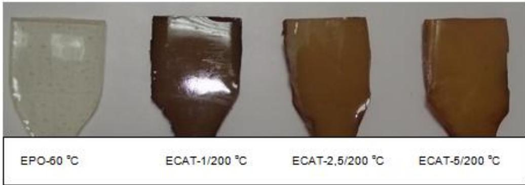
**Figure 3.3:** Color differences of the ECAT samples as a function of boron mineral loading (at 200 °C)
