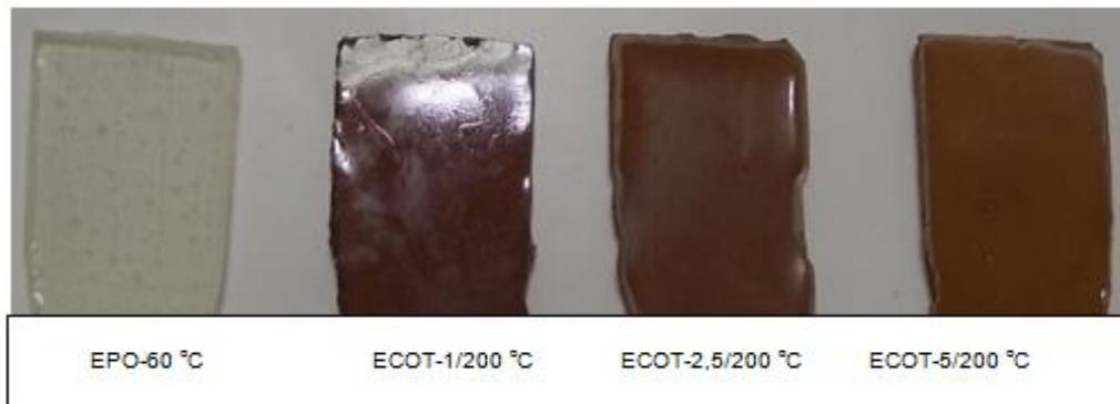
**Figure 3.7:** Color differences of the ECOT samples as a function of boron mineral loading (at 200 °C)
