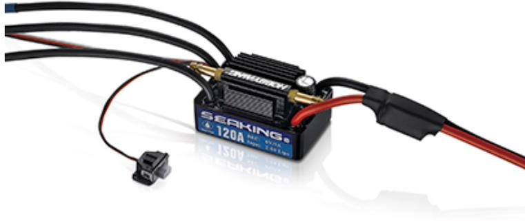
Figure 5.7: ESC utilized in the model boat [10]
