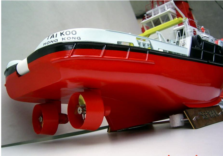
Figure 5.6: Twin propellers with kort nozzles [9]
