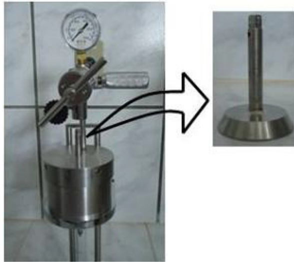
Figure 2.1. Differential Sticking Tester and a Plate (Amorim et. al., 2011)
