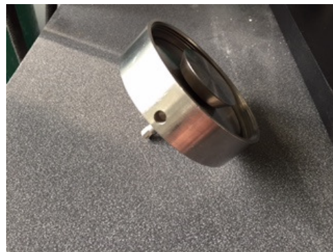
Figure 4.7. Top cap of the test cell with torque plate
