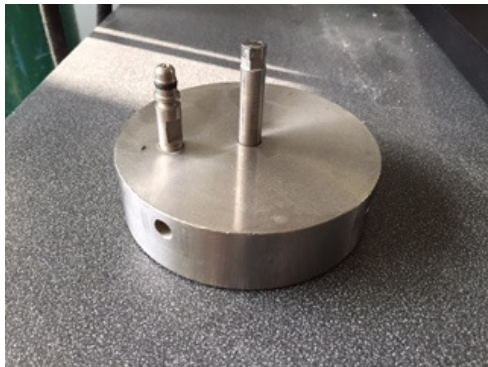
Figure 4.7. Top cap of the test cell with torque plate
