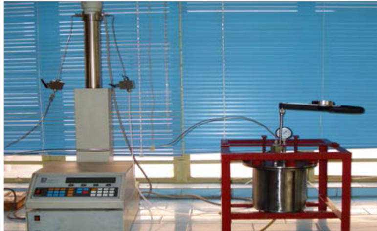
Figure 2.11. Self-Fabricated set up for determination of Sticking Tendency (Mahto et. al., 2012)
