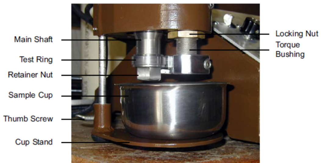
Figure 4.9. Lubricity Tester test ring with related parts (Ofite Instruments, 2009).
