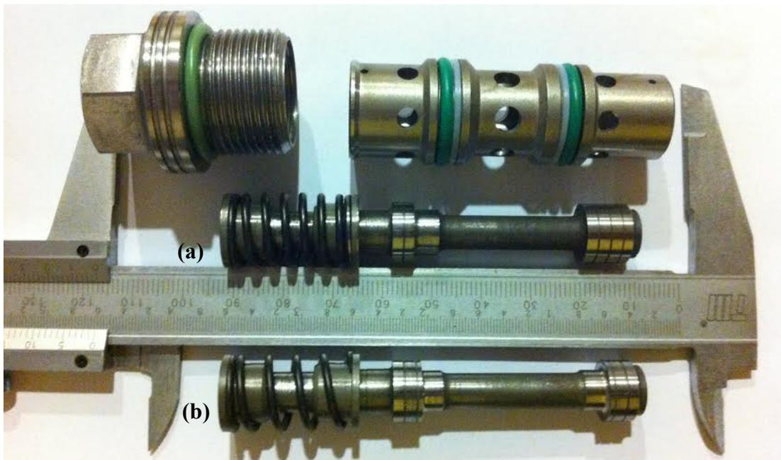
**Figure 5-31 Proposed shuttle valve spool structures, a-) AC port underlapped, BC port closed, b-) spring pre-load removed, AC and BC ports are underlapped**
