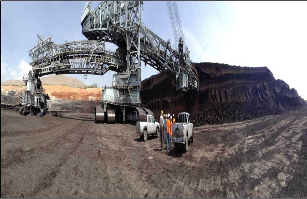
Figure 13. Bucket-Wheel Excavator in the Sector A (source: Düzgün et al. , 2014)
