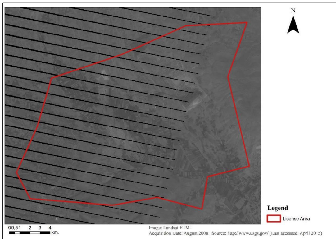
Figure 21. Raw Landsat ETM+ image with gaps
