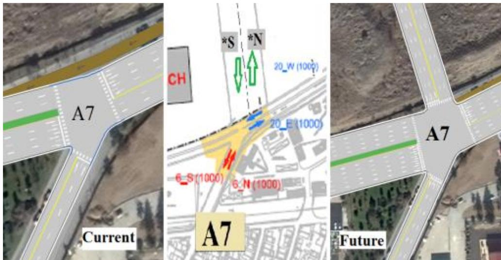
**Figure 6.4** Current and future geometry of "A7" intersection
