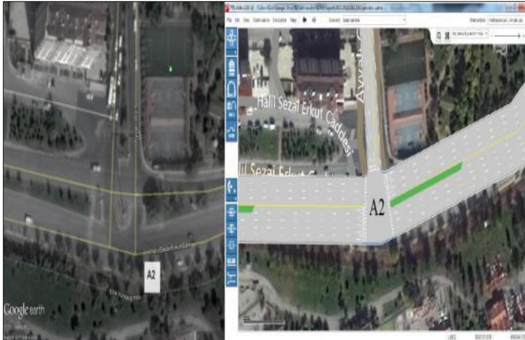
**Figure 5.9** the satellite image on “A2” intersection and its model in Vistro
