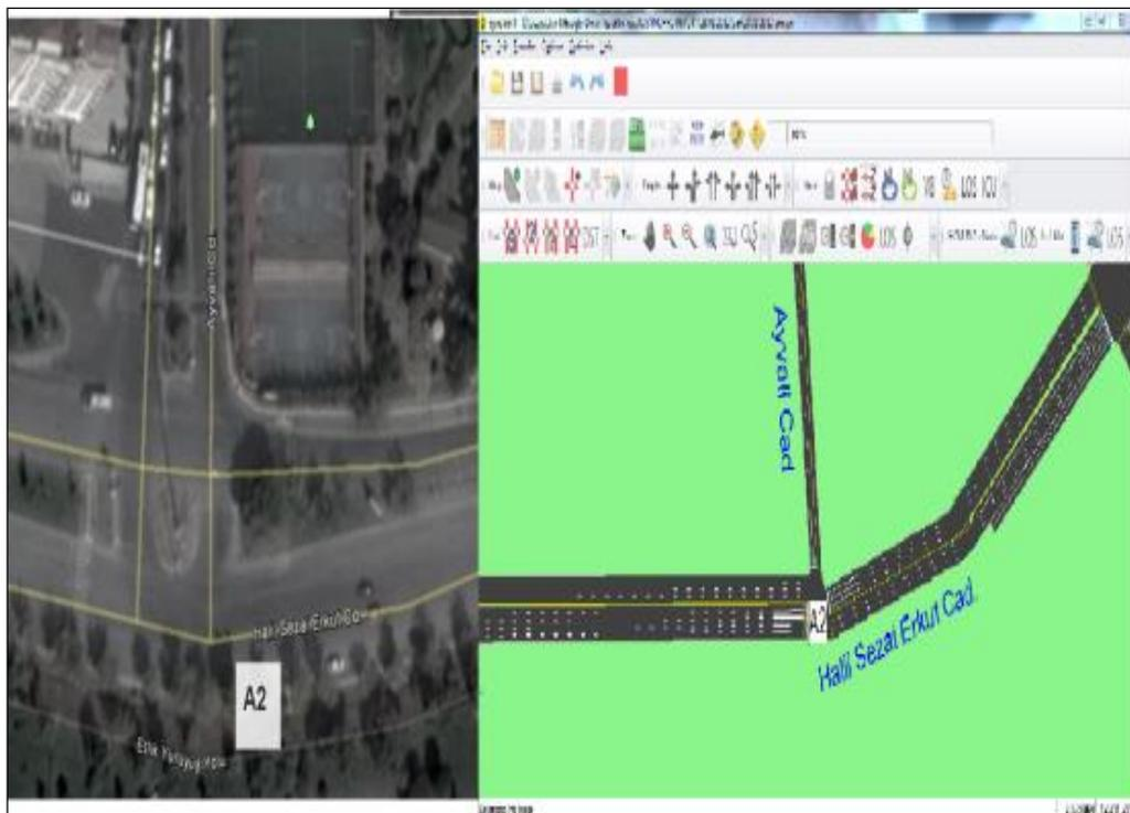
**Figure 5.2** The satellite image of "A2" intersection and its model in Synchro
