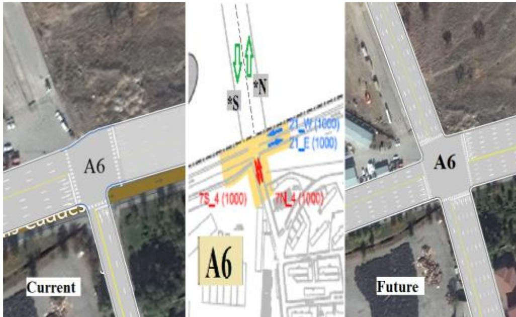
**Figure 6.3** Current and future geometry of "A6" intersection
