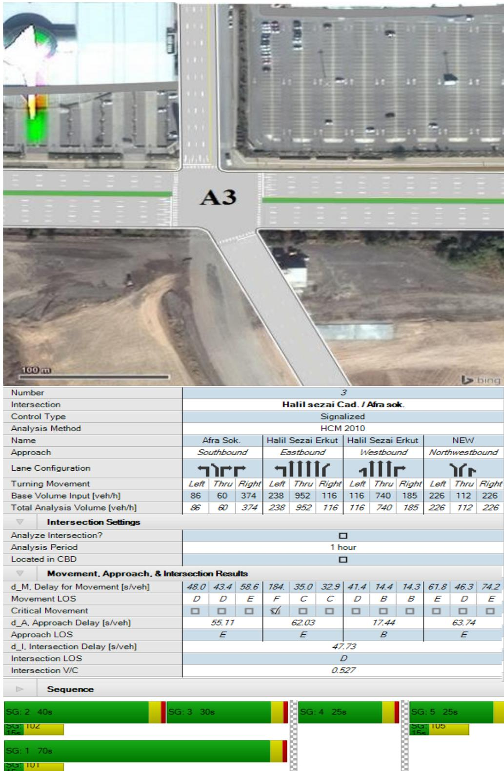
Figure E. 3 Results of Vistro for "A3" intersection
