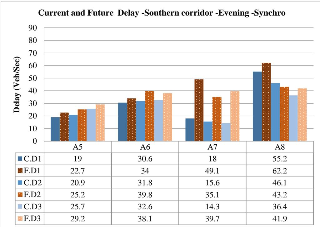
In general, the results showed that the Delay and LOS of all intersections increase in all days. Also, the results by Vistro generally showed higher delay than Synchro, because of their embedded delay function. That is why, the Vistro results seem more reasonable than Synchro.
