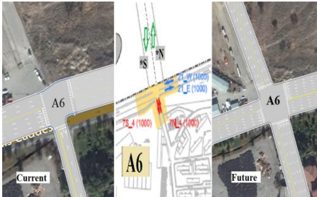
Figure 6.3 Current and future geometry of "A6" intersection
