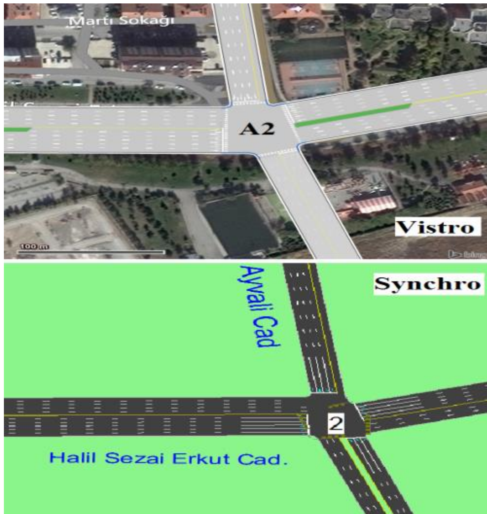
Figure 5.21 shows the new designed intersections for A2 in Synchro and Vistro software.
