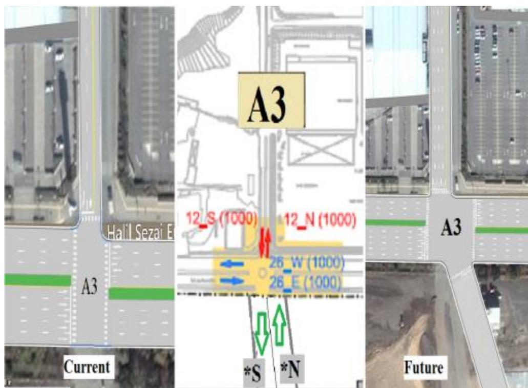
**Figure 6.2** Current and future geometry of "A3" intersection
