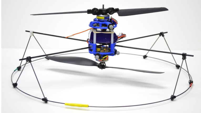
Figure 1.6: Coaxial Helicopter Configuration [21]
