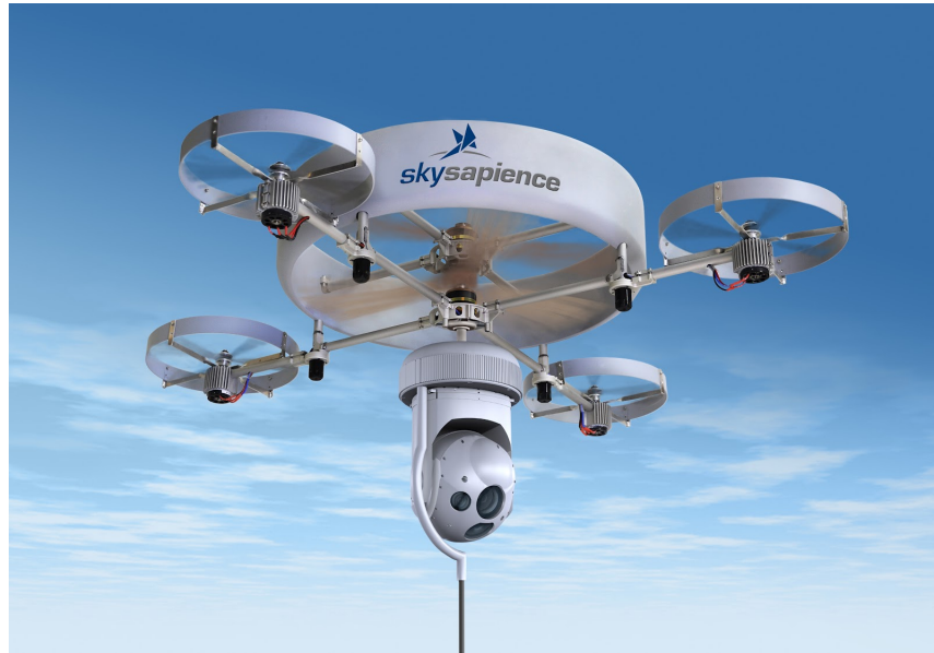
Figure 1.10: The HoverMast from Introduced by SkySapience Company [33]
