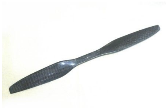
(b) 18x5.5 T-Motor Style Propeller Used as Main Rotor's Propeller
