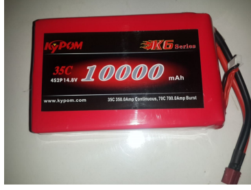
(a) 4s 10000mah Li-Po Used as Main Power Supply
